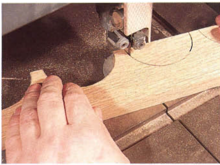
Figure 5: The large half circles in the back racks are created on a band saw; the kerf marks are removed with a drum sander.
