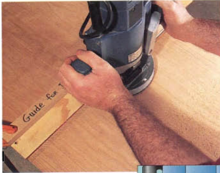
Figure 1: To cut the shelf dados in the cabinet sides, run a router against a straightedge jig clamped to the workpiece.
