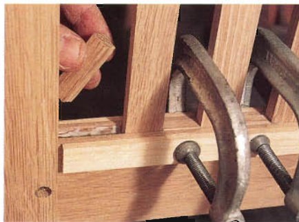
Figure 7: Use scraps of pine between the clamps and workpiece when installing the slat spacers in their dadoes.
