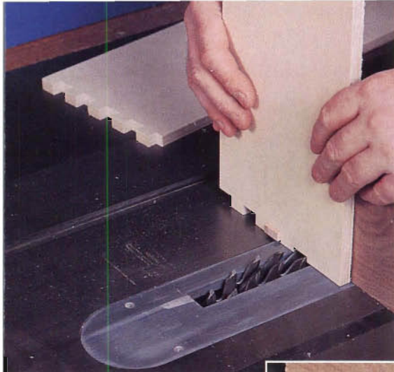
Figure 7: Cut the finger joints with a dado head, using an index pin on your miter gauge's auxiliary fence (see inset) to space the cuts evenly.
