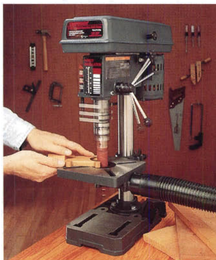
Sears' new Craftsman multi-function drill press is a bench-mounted unit with built-in dust collection and oscillation (for drum sanding).
