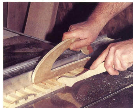
Figure 2: With the dados cut, simply rip off lengths of dentil molding on your table saw. Be sure to use a very sharp blade to avoid tearout.
