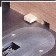
Figure 7: Cut the finger joints with a dado head, using an index pin on your miter gauge's auxiliary fence (see inset) to space the cuts evenly.
