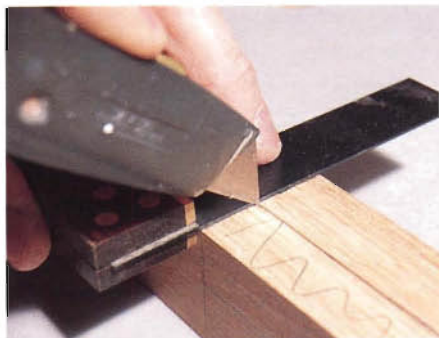
Figure 2: To stop chipping and tearout, a sharp utility knife is used to score across the grain at each end of the stopped rabbets.
