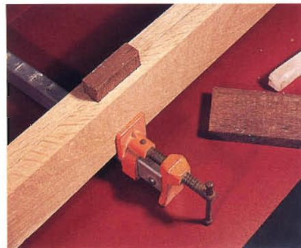
Figure 2: Then glue the two halves together to form the 1\frac{1}{2} " thick sides. I used waxed spacers to line everything up.
