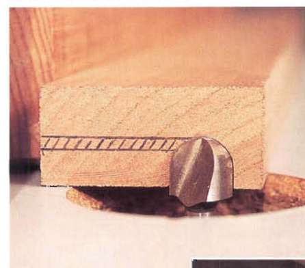
Figure 4: To create the cove molding, make the first cut on your router table with a cove bit, then remove the rest of the waste on your table saw (see inset).
