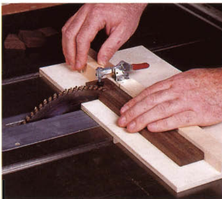
Figure 1: This cross cutting jig rides in the miter gauge slots of your table saw and is equipped with a toggle clamp to keep your fingers out of harm's way.
