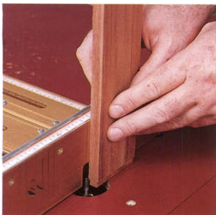
Figure 4: Use a 14° dovetail bit to form the joints on the drawer sides, fronts and backs.
