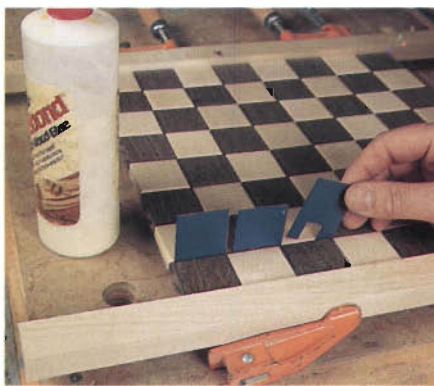
Figure 3: Use several plastic laminate spacers to assure proper alignment when gluing up the squares of the chessboard. Cut a recess in each spacer to fit around the grid pin dowels.
