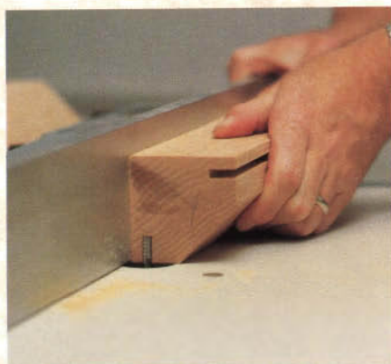
Figure 1: Mortises in the legs (they house tenons on the brackets and aprons) are cut on a router table using a 1/4" spiral fluted straight bit.
