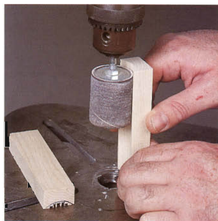
Figure 4: After removing most of the waste with your table saw (workpiece on table), you can form the concave face of the grader's blade with a 1½" drum sander chucked in a drill press.
