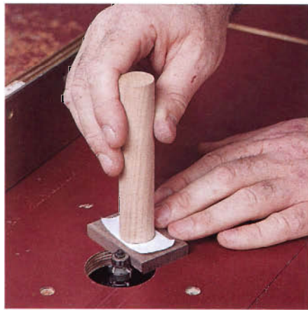
Figure 3: I like to hot melt glue a temporary handle to small parts when routing them, just to keep my fingers away from the cutter.
