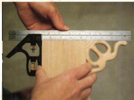
Figure 4: When gluing the brackets to the aprons, a combination square helps line up everything while the glue is still wet.
