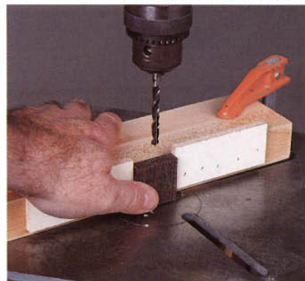
Figure 2: A simple jig facilitates drilling a series of accurate holes for the dowels that hold the chessboard grid together.
