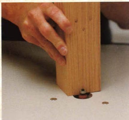
Figure 2: Ease the bottom edges of the legs with a 1/8" roundover bit. At 31 1/4" long, these legs are short enough to perform this operation while holding each leg vertically on the table.
