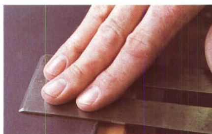
Figure 3: Begin tuning up the leading edge of the cutting iron by flattening its back on your glass lapping plate (above). Complete the process using fine honing stones.
