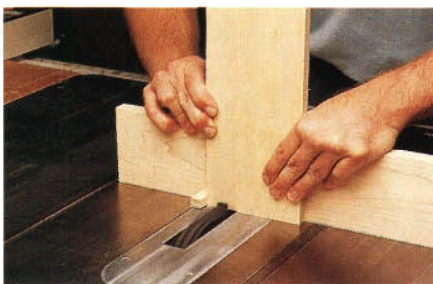
Step 3: Position your tray front against the fence, butted up to the key, and take your first pass. Now simply slip the newly created dado onto the key and take your second pass.
