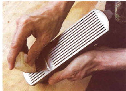
Figure 6: Lubricate your plane's sole often with paraffin wax. It won't contaminate the wood or interfere with the finish.
