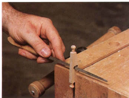
Figure 4: After you've drilled holes in the axles, use a file to elongate them to allow for the free movement of the axle retainer pins.
