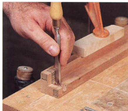
Figure 2: After removing most of the dado for the bottom panel on the drill press, clean out the remaining waste with a sharp chisel.
