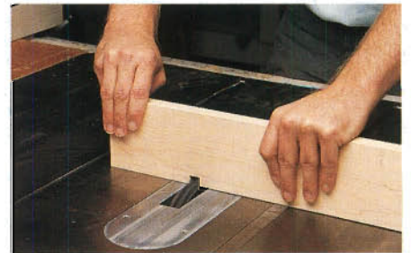
Step 1: Install a 1/2" dado blade in your table saw and screw a tall fence to your miter gauge. Make sure the gauge is square to the blade and, with the blade raised 1/2", make one pass.
