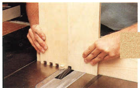
Step 4: After the last cut is made in the tray front, set the mating side tightly against it and start cutting its fingers. Follow this sequence as you work your way around each tray piece.
