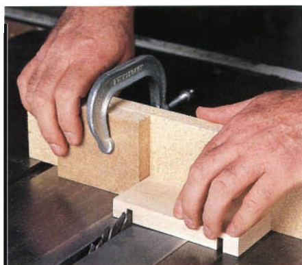
Figure 1: You don't have to use a dado blade to cut the two axle dados in the chassis. Simply make 3 or 4 passes with your regular saw blade.
