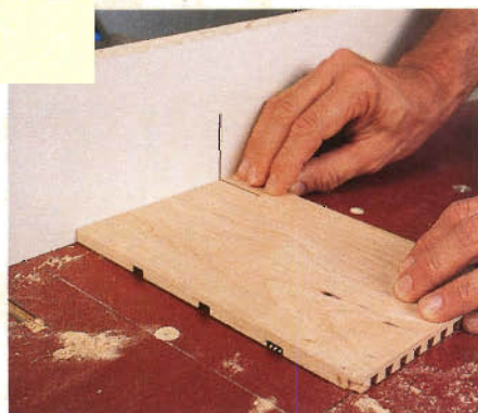
Figure 1: End the stopped dadoes 3/4" from the front of each carcass side by lining up marks on your router table fence and workpiece.
