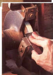
Figure 5: The primary 30° bevel on the cutting iron is created with a honing guide (above). A secondary bevel of 27°-28° is formed using an aluminum oxide wheel on the bench grinder (right).
