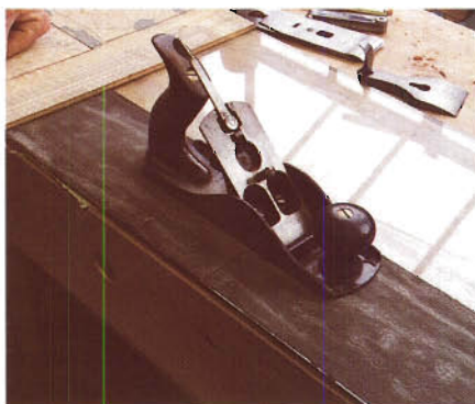
Figure 2: The sole is ground on an absolutely flat abrasive surface. To make a flat lapping plate, glue emery cloth or silicon carbide sandpaper to a sheet of 1/4" glass.
