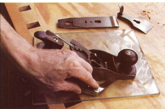
Figure 1: To discover how flat the plane's sole is, the author sets the tool on a piece of 1/4" glass, then he inserts automotive feeler gauges between the sole and the glass.
