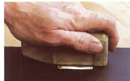
Figure 4: Grind the back of the cutting iron flat on the lapping plate, using a comfortable wooden block both to hold the iron down evenly and to protect your fingers.
