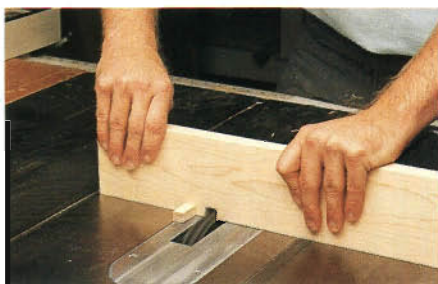
Step 2: Glue a 1/2" x 1/2" x 2" piece of scrap in the dado (the "key") and reposition the fence 1" further to the right on the miter gauge. Make another pass, leaving a 1/2" gap between cuts.
