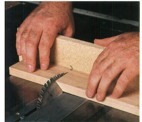
Figure 3: To ensure a square cut, attach a long auxiliary fence to your miter gauge when cutting long parts such as the lid front and back.
