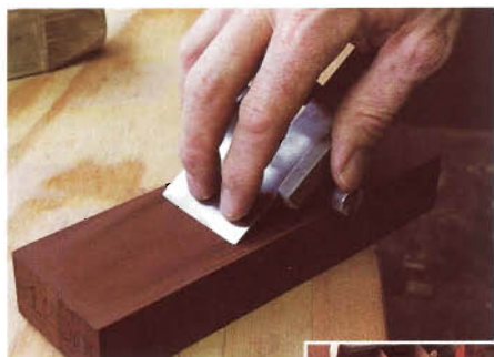
Figure 5: The primary 30° bevel on the cutting iron is created with a honing guide (above). A secondary bevel of 27°-28° is formed using an aluminum oxide wheel on the bench grinder (right).
