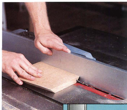
Figure 6: After all aprons are cut to size, remove the two jigs and reset the blade to make the 1/4" deep kerf cuts for the spines, as shown at right.
