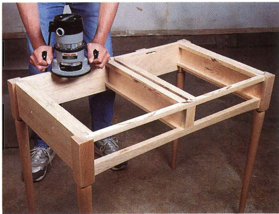
Figure 2: Once the drawer support assemblies are in place, chuck a slot cutting bit in your router to quickly cut the eight table top fastener openings around the top.
