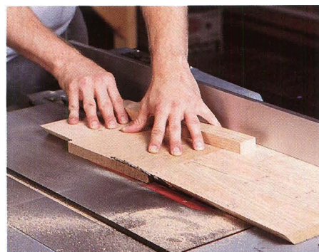
Figure 5: Keep your blade and rip fence in position and switch to Jig #2 to cut the left side of each apron. The scab piece on top keeps the newly mitered edge from riding up during the cut.
