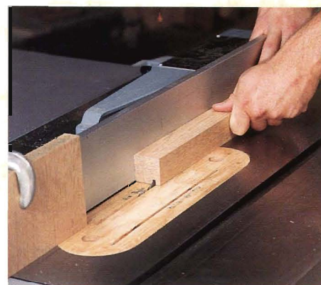
Figure 3: With a stop block in place to create a 7" spline groove, cut the right side of each leg, then reset the fence to cut the opposite sides.
