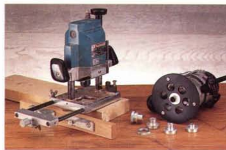
Figure 4: Along with a new router, every basic woodshop should be outfitted with an edge guide (left) and a set of rub collars.
