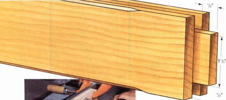
Figure 1: Plough grooves in the rails and stiles first, then use a 1/2" dado blade, a set up block and your miter gauge to cut the tenons. Later you can rout the outside edges with a chamfering bit.
