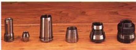
Figure 3: For the tightest grip on router bits, better collets have tapered bodies with at least three expansion slots.
