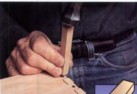
Figure 6: Make a pad for driving in your pins by boring a shallow dimple in one end of a piece of scrap wood.
