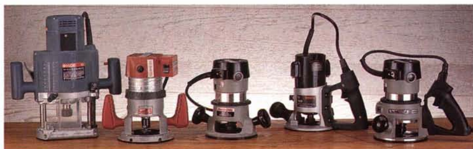
Figure 2: Although there are many slight variations, you'll find that routers have handles that are either shaft grips (left), pommel grips (center) or D-grips with secondary pommels (right).
