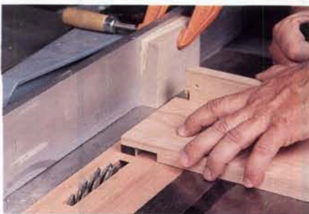
Figure 4: Form tenons using a 1/2" dado blade, a set up block and a miter gauge, adjusting the blade height for the various tenon layouts.
