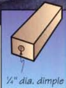
Figure 6: Make a pad for driving in your pins by boring a shallow dimple in one end of a piece of scrap wood.
