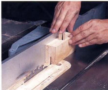
Figure 2: The jig safely holds the hubs at the correct cutting angle. Leading with one end of the jig, and then switching to the other keeps the kerfs centered.
