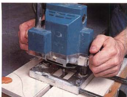
Figure 1: Cut the slot in the seat using your router, a fence attachment and a 1/2" bit, making several passes to ensure a tight fit with the head.
