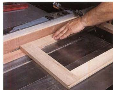
Figure 3: After cleaning glue off the internal frames, form tongues on the rails with a 1/4" dado blade. Be sure to clamp a wood face to the fence.
