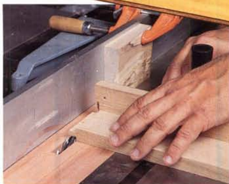
Figure 1: Plough grooves in the rails and stiles first, then use a 1/2" dado blade, a set up block and your miter gauge to cut the tenons. Later you can rout the outside edges with a chamfering bit.
