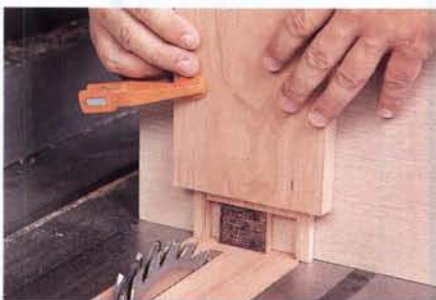
Figure 5: To remove the extra waste for the back apron tenons, screw a tall fence to your miter gauge and clamp the stock for each pass.
