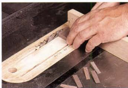
out the slots for the wedges and use a band saw for the cuts. Follow up by drilling a 1/8" hole at the end of each slot to reduce the chance of splitting when driving in the wedges.
