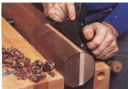
Figure 1: After trimming most of the waste off your laminated block with a table saw, complete the shaping of the fuselage with a hand plane.
