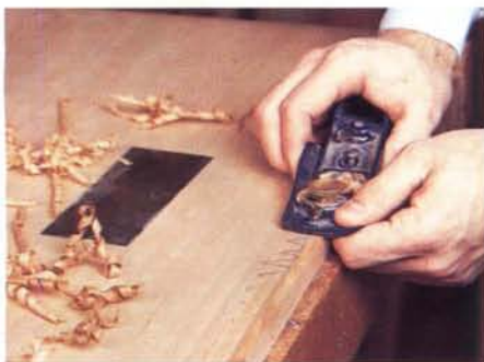
Figure 2: Scribble pencil lines alongside the banding, then when you begin planing through the lines you'll know it's time to switch to a scraper.
