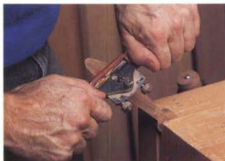
Figure 3: Bandsaw the propeller from a piece of 1/2" thick walnut and then use a spokeshave, a file and a whittling knife to bring the blades to final shape.
