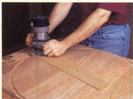
Figure 7: To rout the top round, make a trammel jig from 1/4" plywood and mount it to your router base. Use a 1/2" long wood screw for the pivot point.
