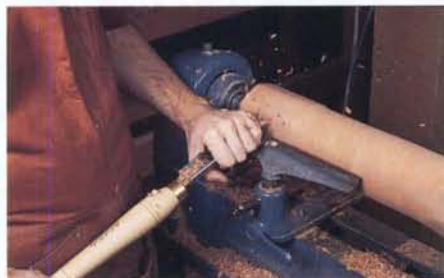
Step 2: Mount the blank in your lathe and, with the wood revolving at a slow speed, turn a 3/4" diameter cylinder using a large roughing gouge.
