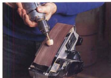
Figure 4: Shape your spinner into a cone by chucking the assembly in your drill and holding it against a belt sander while both tools are running
