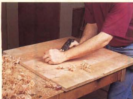
Figure 6: Surface the panel for the table top with a well-tuned and sharpened hand plane after the glue in the joints is thoroughly cured.
