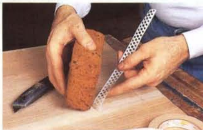
Step 1: Joint the edges and hold them together with masking tape, then flip the veneer over and apply veneer tape to the seam.
