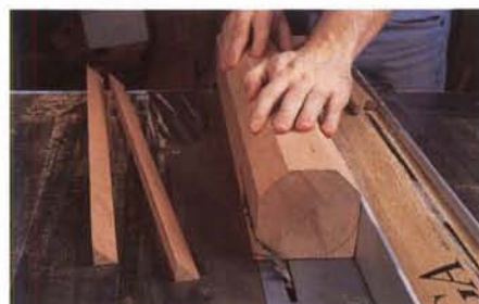
Step 1: Trimming the corners of the blank at a 45° angle will quickly reduce the amount of wood you have to remove during the turning process.
