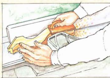
Figure 4: Taper each side of the legs by making three light passes over the jointer, each pass being a few inches longer than the one before.
