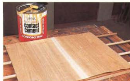
Step 3: Apply contact cement to both the veneer and the substrate and let it dry. Use stickers to position the veneer over the substrate.
