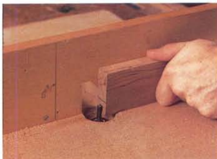
Figure 3: To rout the stile mortises, chuck a 1/4" straight bit in your router table and draw a line on the fence that shows where to stop the cuts.
