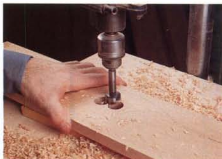
Figure 3: The best tool for boring the four holes that make up each clover cutout is a Forstner bit, although a spade bit will also do the job.
