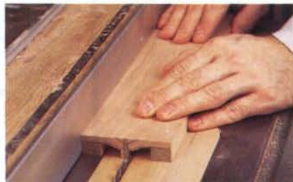
Step 1: Draw the pattern for a pair of handles on 3/4" stock and, adjusting the blade height for each cut, rip the waste from the pull areas.
