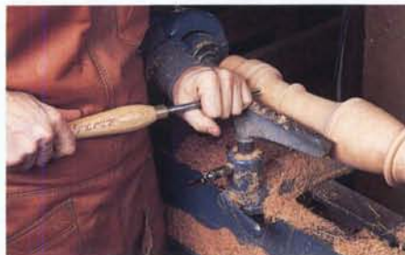
Step 5: Shape the inside curves with a set of spindle gouges, making the final passes with the bevels firmly contacting the wood for smooth cuts.
