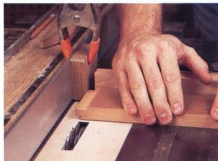
Figure 4: Clamping a set-up block to the fence for aligning the tenon cheek cuts will reduce the chance of a kickback.
