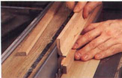
Step 3: Once the shaping is completed rip off the outside bridges, leaving perfect surfaces for gluing the handles to the drawer faces.
