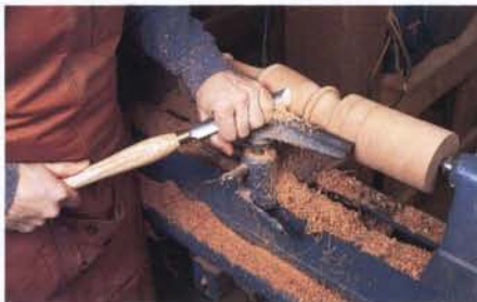
Step 6: Use your skew chisels to form the beads, base, tenon and urn, and to plane the flatter areas of the pillar to their finished size.
