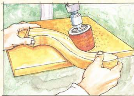
Figure 5: To form the bevels, tilt the drill press 15° and keep your legs in contact with the most acutely angled point on the drum sander.
