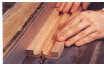
Step 2: Tilt the blade 45° and cut a shallow V on the top surface of the stock. These cuts begin to form the drop on the front edge of each handle.
