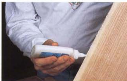
Step 2: Remove the masking tape and spread white glue on the seam, then unfold the veneer and place it under pressure while the joint dries.
