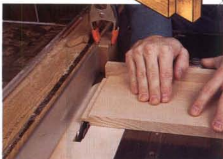
Figure 2: Cut tenons on the shelves, apron, top rail and bottom with a 1/2" dado blade, making sure to use a set-up block for safety.
