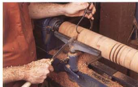
Step 4: Using a parting tool and a caliper, define the major high and low points of the pillar by taking your measurements off the storyboard.
