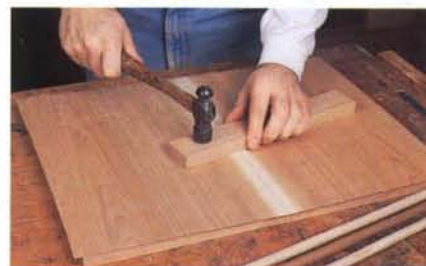
Step 4: Carefully pull out the stickers and lay the veneer on the substrate, then tamp the surface with a hammer and scrap wood block.
