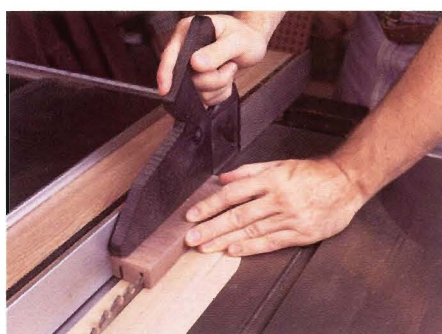
Figure 1: After cutting stock to size for the upper cab, adjust your blade height and fence and make two cuts to define the inside edges of the posts.
