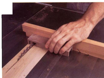
Figure 3: Lay out the posts and overall length of the cab, then support the stock with your miter gauge while clearing the remaining waste.
