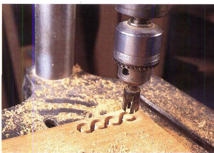
Figure 5: Make your own mahogany plugs using a 3/8" plug cutter. Try to pick wood for the plugs that matches the grain and color of the project.
