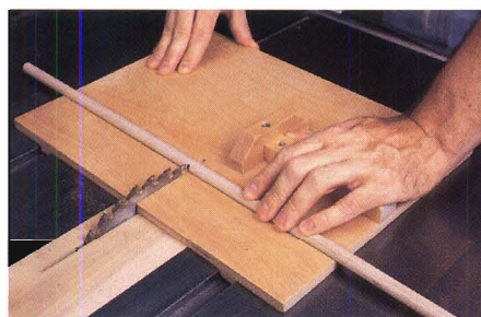
Figure 2: To improve the safety of cutting dowels to length, construct a simple table saw sled with a V-groove that rides in the miter gauge slots.
