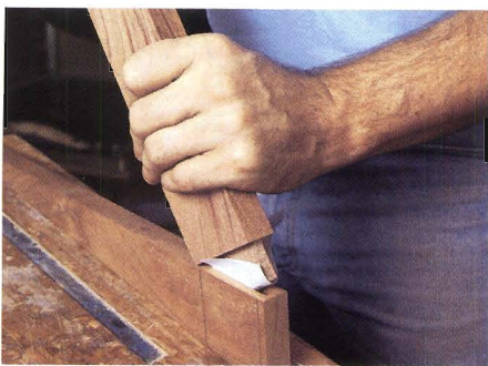
Figure 3: To judge the fit of a mortise and tenon joint, wrap the tenon with a slip of paper and see if it slides into the mortise with only slight resistance.
