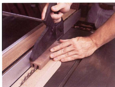
Figure 2: Continue adjusting the fence about 1/16" at a time to make a series of passes for nibbling away the waste in the cab.
