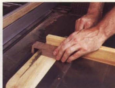
Figure 3: Support the cab with a miter gauge while removing the waste that remains between the cab posts and to cut the piece to length.
