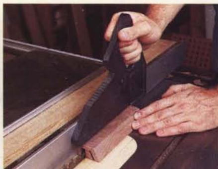
Figure 2: Return the blade to 0° and define the back posts, then clear the waste from between the posts by moving the fence a little bit for each pass.
