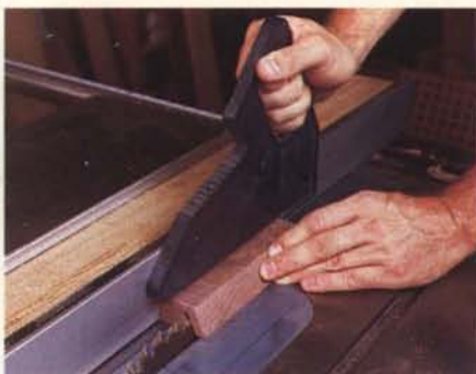
Figure 1: Rip the front edge of the cab at a 25° angle, then lower the blade and move the fence 5/16" to cut the inside edge of the front posts.
