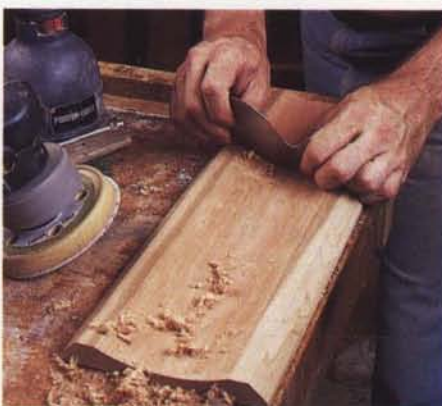
Figure 2: After shaping the walls, clean the saw marks off the stock with a gooseneck scraper, then smooth it with a random orbit or palm sander.
