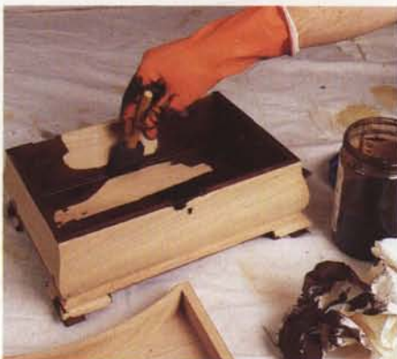
Figure 4: Using a sponge brush, apply the aniline dye stain liberally, and wipe off the excess after allowing it to soak in for several minutes.
