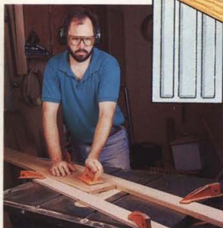
Figure 1: Clamp the fences to the saw table with the blade centered between them. To further ensure that you cut a symmetrical arch, run the stock through, then turn it end for end and make a second pass.
