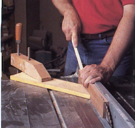
Figure 2: To resaw the clapboard, tilt the saw blade 5° (leaning away from the fence), and use a fingerboard and push stick during the cuts.
