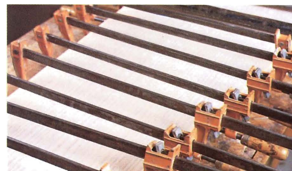
Figure 1: The 1/4" banding will easily conform to the front edge of the sides, but use as many clamps as you can to get a seamless joint.
