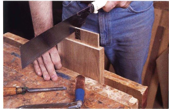
Figure 5: Once you've formed the tenons with your table saw, dado blade and miter gauge, cut the gap in each lower rail tenon with a hand saw.
