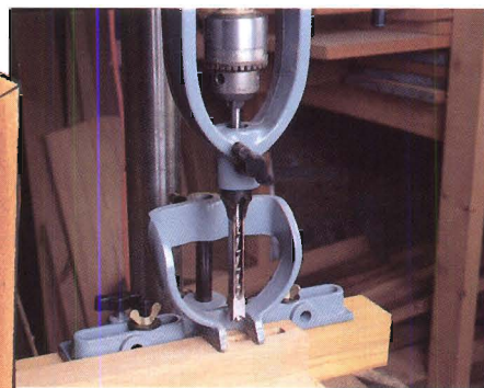
Figure 3: A drill press attachment will make short work out of mortising the legs. As the coarse drill bit removes most of the waste, the chisel shapes each hole into a square.
