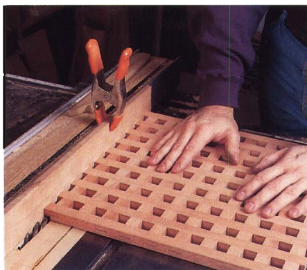
Figure 2: Cut tenons on the assembled grate after clamping a protective wood face to your fence.
