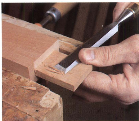
Figure 4: Pare the tenons with a 3/4" chisel. At the point when you can slip a dollar bill between the tenon and the mortise you'll have a perfect fit.
