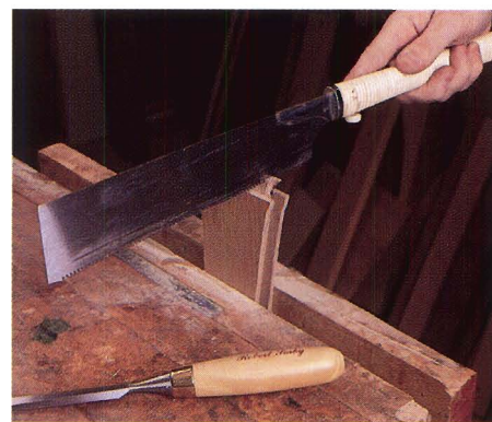
Figure 3: You'll need a handsaw to cut off the small tips that remain on the curved rail tenons after routing the grooves with a slot cutting bit.
