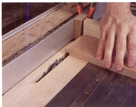
Figure 1: To safely cut tenons with your table saw, clamp a set-up block to the fence and use the miter gauge to support the stock.
