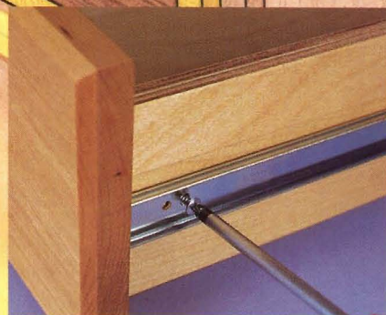
The elongated holes in Accuride slides make it easy to adjust the drawer for a better fit.
