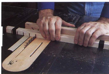
Figure 3: Stiffen the shingle veneer strips by sandwiching them between scrap wood, then use tape as a marker for the repetitive kerfing cuts.
