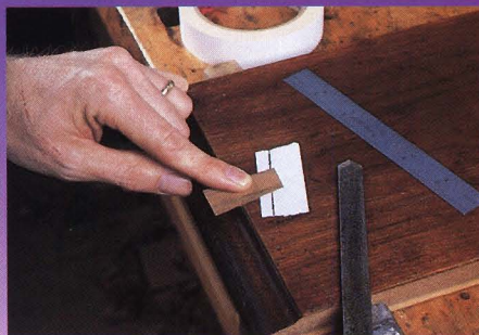
Step 5: For a three sided repair, press white tape over the end of the hole, draw the cutting angle and mark the angle on the patch.
