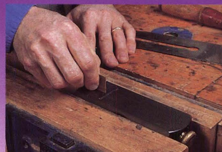
Step 3: While holding your block plane in a vise, pass the veneer patch over the blade to straighten one edge for matching the edge of the hole.
