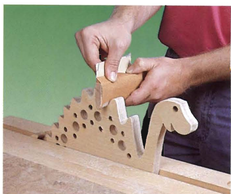
Step 4: Make a V-shaped sanding block out of 1/2" stock for getting into the tight spots in the gaps along Nessie's back.
