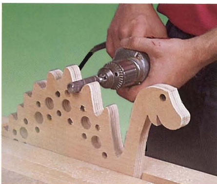
Step 3: Secure Nessie in a vise while you sand the bandsawn edges with a 1/2" diameter drum sander chucked in a portable drill.
