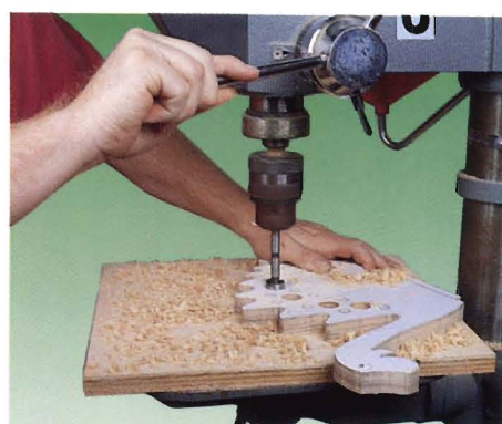
Step 2: Drill all the button holes completely through the figure, making sure to back up the plywood with a scrap piece to prevent tear out.
