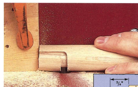
Figure 3: Rotate the ends of each support dowel over a \frac{1}{2}" straight bit raised \frac{1}{4}" to form tenons with a router table.
