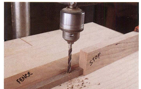
Figure 1: To repeatedly drill all the 1/4" diameter pivot pin holes in the fence rails, set up a fence and stop on your drill press table.
