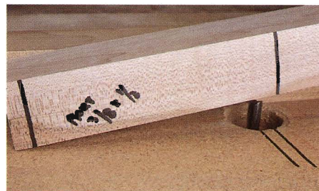
Figure 2: Clearly mark the end points of all the post grooves so you can start and stop your drop cuts at the right spots on the router table.
