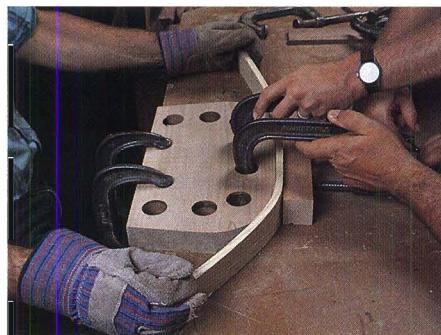
Figure 1: Once the steamer was working properly our ash bent quite easily—a bending strap wasn't even necessary.
