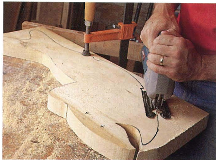
Figure 1: Layout the fish body and the other shaped pieces so they avoid knots in the lumber, then cut them with a band saw or saber saw.
