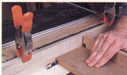
Step 1: When cutting a rabbet in the drawer front, clamp a protective wood face to your saw fence.
