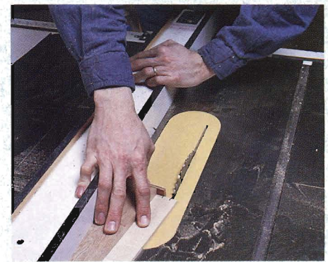
Figure 4: Screw a stop to the square corner of one cutting guide and, keeping the saw off, use it to align the marks on the maple with the saw blade.
