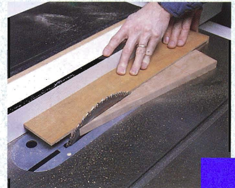
Figure 2: To rip the cutting guides, nail a scrap of plywood to the board so its edge aligns with the pitch line, then cut the piece along this line.
