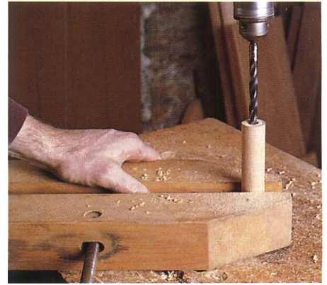
Figure 1: To ensure straight holes in the handle and washers, use a wood handscrew clamp to hold the dowels square to the drill press table.
