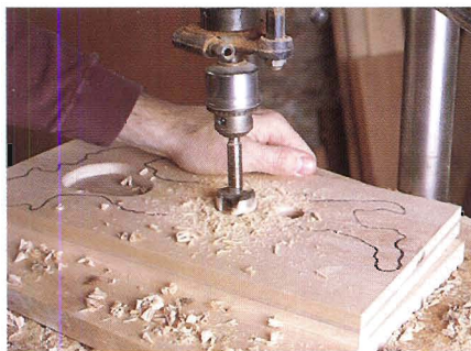
Figure 1: Forstner bits produce the smoothest holes, but to avoid tearing out the back of the lamination be sure to use a back-up board.
