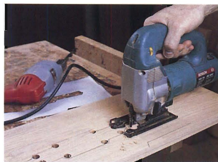
Figure 5: To form the opening on the backsplash, first drill relief holes at every inside corner, then use your saber saw to cut from hole to hole.
