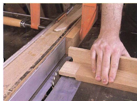
Figure 2: Chamfer the ends of the tenons by tilting your blade 45° and clamping a clearance block to the fence to align the workpiece with the blade.
