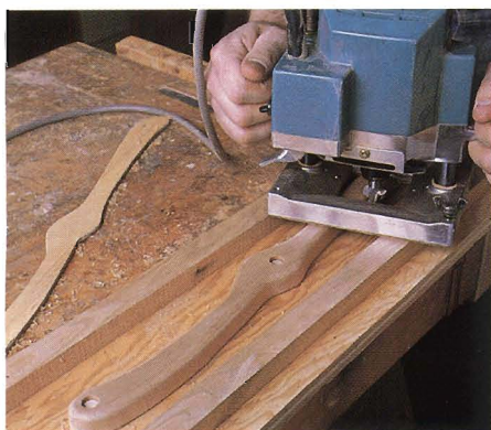
Figure 1: The routing jig (see drawing at right) holds your stock steady and supports your router while you roundover the legs and arms.
