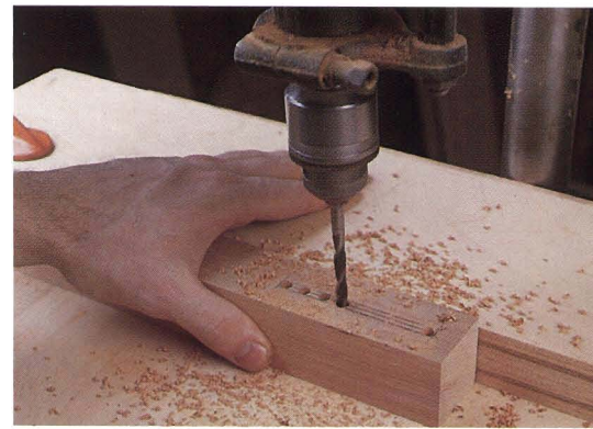
Figure 5: To rough in a mortise, first drill at the ends of the layout, then bore holes every 1/2". Finish up by drilling out the stock between the holes.
