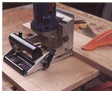
Figure 2: To keep the biscuit joiner steady during a face cut, first position the machine on the cutting line, then clamp a fence to your stock.
