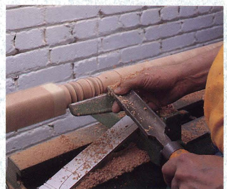
Figure 4: A small gouge and a diamond shaped scraper work well for cutting the beads and coves on the legs, while a large gouge and a skew chisel are best for shaping the long tapers.
