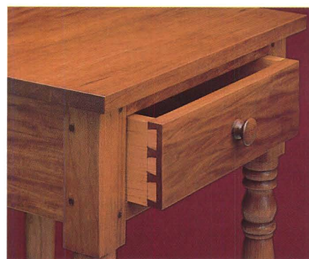
Figure 6: Marking gauge layout lines, slightly irregular dovetails and square drawboring pegs are telltale signs left by the hand of a craftsman.
