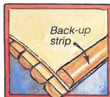
Figure 4: Covering the end of the canvas with a back-up strip will keep the fabric from unraveling.
