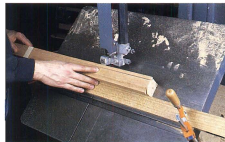
Figure 1: To make your legs easier to turn, tilt your band saw table 45° and trim the edges off each blank from the foot end to the shoulder lines.
