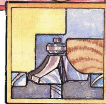
Figure 2: To keep the strips stable while routing, cut them six inches longer than necessary, then rout all but the last two inches on each end.
