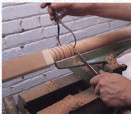
Figure 3: The story stick lines represent the high and low areas of the leg. Use your caliper and a parting tool to cut the low areas to a slightly larger diameter than their finished dimension.
