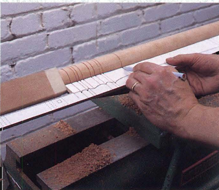
Figure 2: Once you've turned the blank round with a large gouge and nibbled up to the shoulder lines with a parting tool, use your story stick to layout the major parts of the leg.
