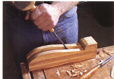
Figure 5: Once the walls are cut, remove the rest of the waste with a chisel, making sure to extend the groove into the crease below the knob.
