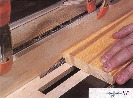
Figure 1: For protection, clamp a wood face to your fence while cutting the tongues with a 3/8" dado blade raised 1/4".
