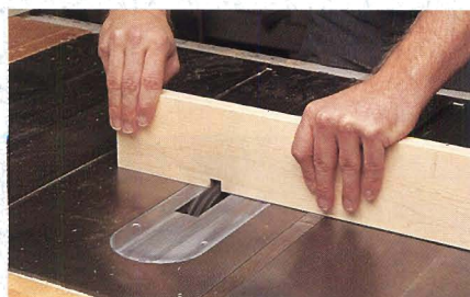
Step 1: Install a 1/2" dado blade in your table saw and screw a tall fence to your miter gauge. Make sure the gauge is square to the blade. With the blade raised 9/16", make one pass.
