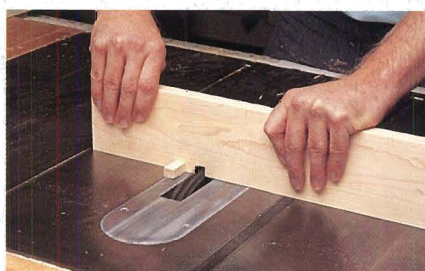
Step 2: Glue a 1/2" x 9/16" x 2" piece of scrap in the dado and reposition the fence 1" further to the right on the miter gauge. Make a another pass, which should leave a 1/2" gap between cuts.
