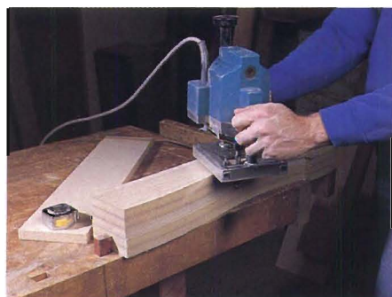
Figure 1: Glue the particleboard form together with the smooth piece in the middle, then rout the others to match with a flush cutting bit.
