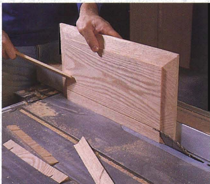
Step 2: With the blade tilted 12° and the fence 5/16" away, raise the end grain edges of the panel first, then the long grain edges.
