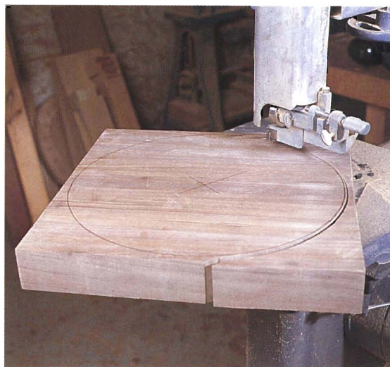
Figure 2: Once the chip and dip cavities are routed to a depth of 1½", turn over the blank and use a compass to layout the outside perimeter of the tray. Next, cut the tray out with a band saw, but stay about 1/16" outside the line.
