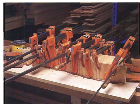
Figure 3: Begin clamping at the deepest curve, then work out from there. Vary the clamp positions so that the entire lamination is under pressure.
