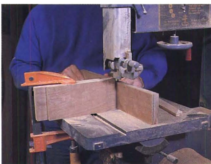
Figure 2: For resawing, clamp a V-block fence to your hand saw table to guide your thicker stock. Always use a push stick during this operation.
