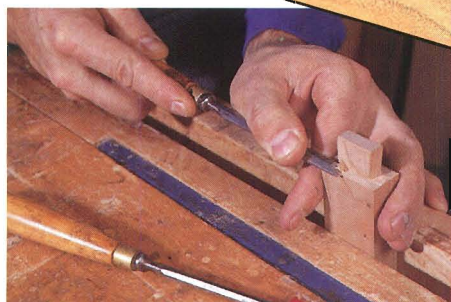
Figure 3: Paring the tenon shoulders until they're flush all around ensures a perfect fit.
