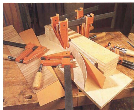
Figure 6: To even the clamping pressure on the thin laminations, use backer strips of plastic laminate and bending plywood or untempered hardboard.
