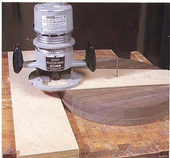
Figure 3: To finish the outside edge use a circle routing jig. Define the radius of your circle on the jig, then nail the jig at this point to the center of the tray. Make two passes to rout the full depth.
