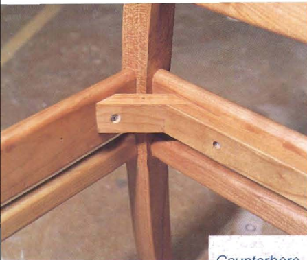
Figure 5: Corner blocks ease excessive stress on a chair and serve as a base for securing the seat.
