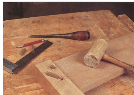
Figure 2: Adjust the hole positions in the aprons by 1/32" and square the holes. Driving the pegs in this assembly will pull the apron shoulders tight.
