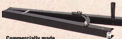
Commercially made aluminum jigs are available from most mail order tool suppliers.
