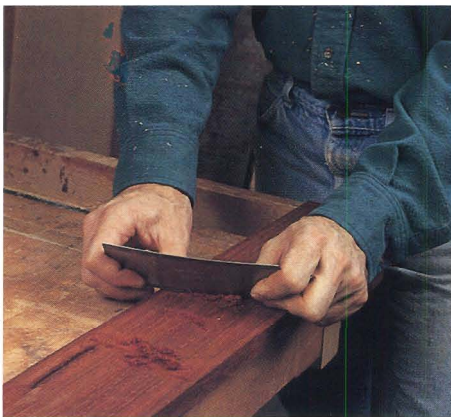
Figure 5: To produce fine shavings with a scraper, firmly hold the blade so it curves slightly in the middle and keep it at a 45° angle to the wood.
