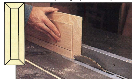
Figure 2: Raising the panels is a two step process. First cut 1/8" deep kerfs on the face of the panel (shown above), then raise the blade and angle it 12° to cut the sloped edges (shown below).
