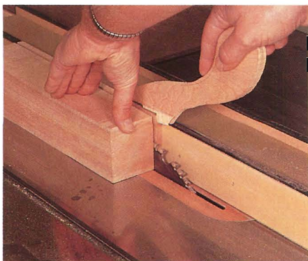
Figure 2: Continue with 1" deep cuts until the wood is split, using a push stick to keep the narrow resawn piece from kicking back.
