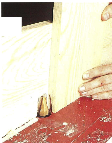
Figure 8: The new panel raising bits from Byrom Manufacturing are very safe for the home shop woodworker. Be sure to use a tall fence to gain greater stability while routing large panels.
