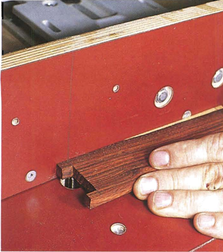
Figure 3: Mark a line on the fence to show the center of the 3/16" bit and line up one shoulder of each side with it. Gently set the side onto the bit and rout until the shoulder at the other end of the piece reaches the fence line. Square the rounded ends of the grooves with a chisel.
