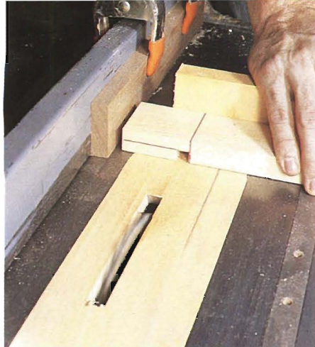
Figure 2: Cut the lap joints with a 1/2" dado blade raised to 3/8". Adjust the fence and set up block to align the shoulder on the face frame piece with the blade. Take a first pass to cut the shoulder, then take more passes to clear the waste.
