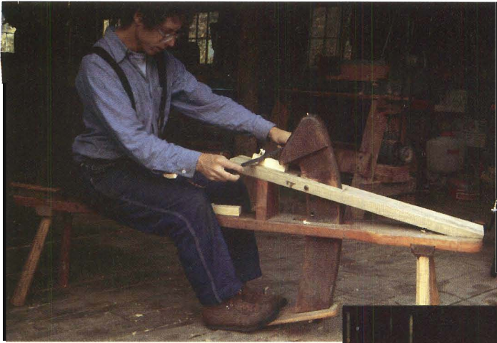
Drew works at his shaving horse with a drawknife to round the outside face of the staves and to bevel their edges close to the finished angle.
