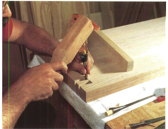
Figure 4: Remove the tail opening waste with a series of chisel cuts, setting the chisel just inside the layout line and tapping the mallet lightly.
