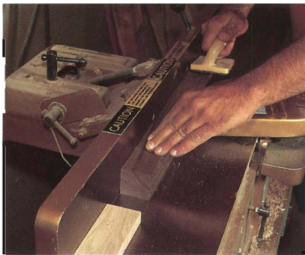
Figure 5: Take one pass to create the leg's reveal, pushing the stock through the jointer until it hits the stop block, then carefully lifting it away.
