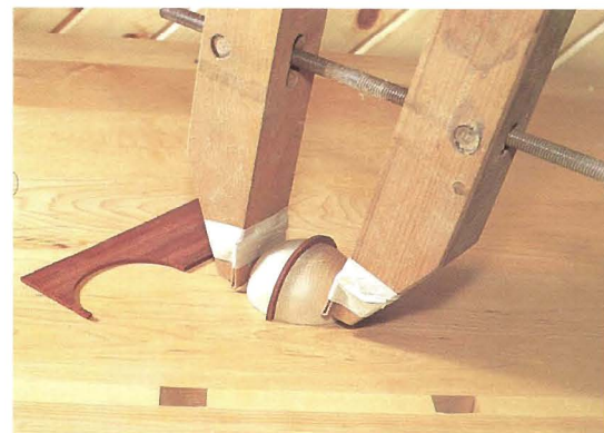
Figure 6: A wooden handscrew clamp works well to assemble the ball caps. Tape a folded piece of sandpaper to the ends of both jaws to get a better grip and to protect the maple ball sections.
