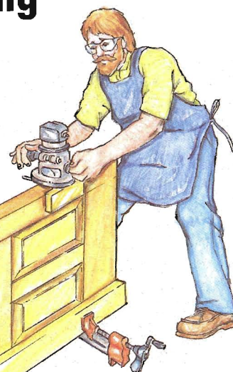
Figure 2: Carefully rout away the flat bottom of the mortise, staying 1/32" inside the cut you made with the utility knife.
