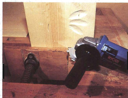
Holding the grinder so the blade is at right angles to the workpiece yields the greatest control and the fastest cutting action.
