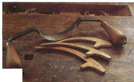
One pattern, or modell, is made for each different bowl circumference to indicate both the outside curvature and the edge angle of the staves.
