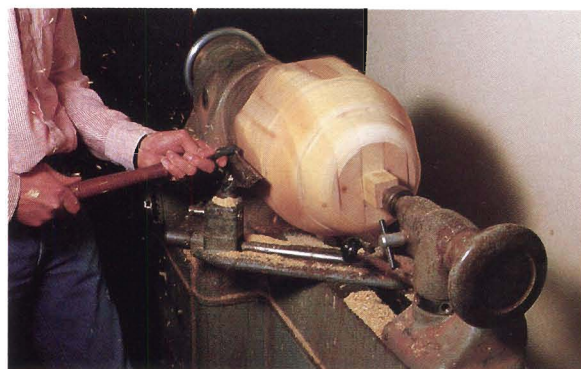
Figure 2: Use a large roughing gouge and run the lathe at a very low speed to turn the blank into the apple shape.
