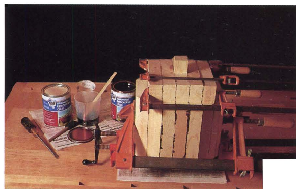
Figure 1: Clamp the birdhouse together by turning the assembly upside-down and setting it onto two bar clamps. Add more clamps as needed.
