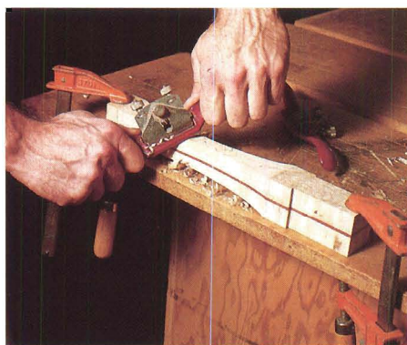
A comfortable handle is the key to a successful mallet. To reduce tearout while spokeshaving (above) work from the high points to the low.
