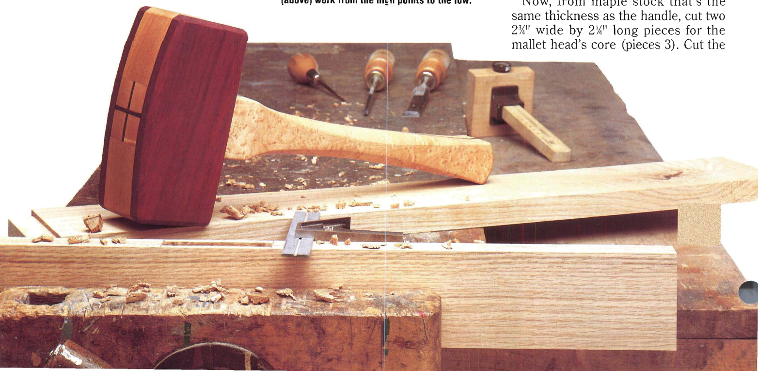
A comfortable handle is the key to a successful mallet. To reduce tearout while spokeshaving (above) work from the high points to the low.
