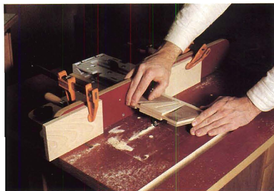
Figure 1: Make the pressure bar slot by clamping stop blocks against the fence to limit the cut and routing 1/4" deep per pass.
