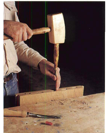
Figure 2: Use the pattern above to layout all the angled tenons in the project. Hollow out the rail mortises with a 3/8" drill bit, then clean up the mortises with very sharp chisels.
