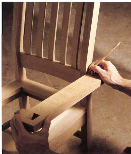
Figure 3: Align the arm mortise with the front leg tenon and rest the arm on the shoulder. Layout the rear joint where the arm intersects the back leg.
