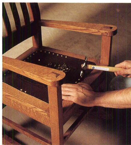
Figure 6: Trim the leather to lap onto the side rails by 1" and 2" on the front and back rails. To prevent splitting, predrill the nail holes 1" apart.
