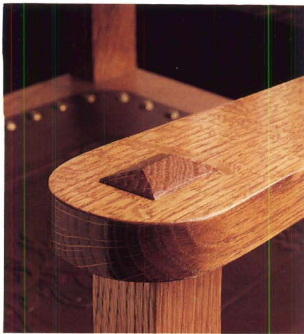
Figure 5: Recreate this symbol of superior craftsmanship from the Arts and Crafts era using a 1" chisel, a tenon saw and your hand tool skills.
