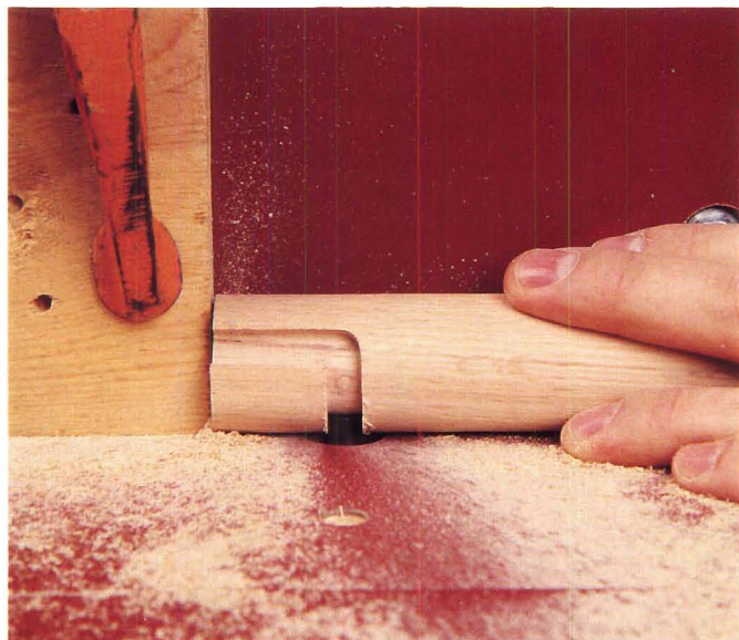
Figure 2: The next step on the legs is routing the tenons. Install a 1/2" straight bit in the router and clamp a stop block to the fence. Approach the bit from the right until the dowel touches the stop block, turn the leg once to cut the shoulder, then slide the dowel in and out over the bit to remove the rest of the waste.
