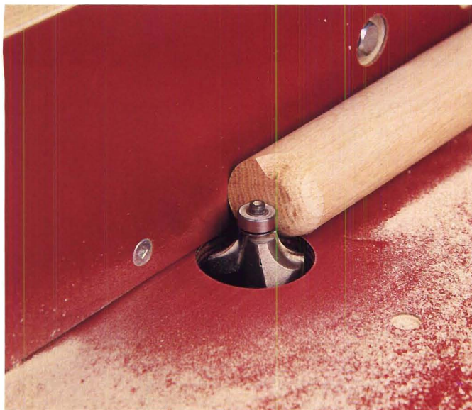
Figure 1: The first operation on the router table is rounding over the ends of the legs. Clamp the fence 5/8" away from the center of the bit, then carefully approach the spinning bit from the right side until the dowel contacts the bearing. Now rotate the dowel in place to roundover the entire edge on the bottom of the leg.
