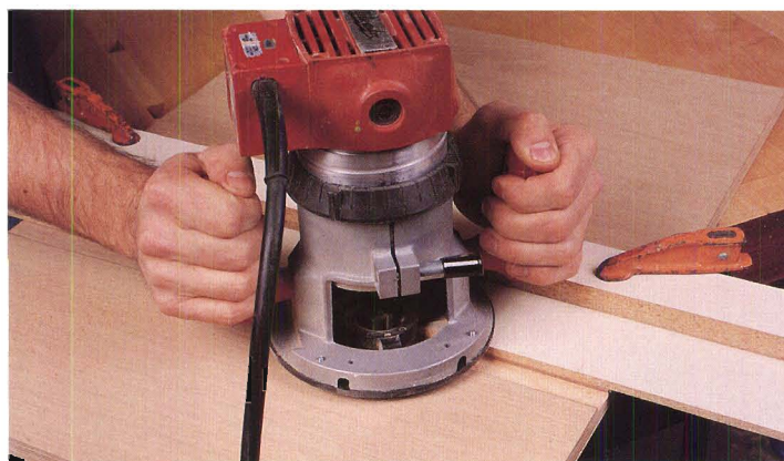
To make this jig, fasten a straight, narrow board to an oversized piece of hardboard, then rout the edge of the jig with the router and bit you intend to use for the dado. Next, align the edge of the jig with the layout line and rout the dado.
