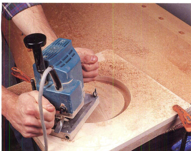
Figure 5: Rout the recesses in the platform and seat using a template and a piloted straight bit. Since the router base won't reach the center of the circle from the template's original position, move the template over as you go.
