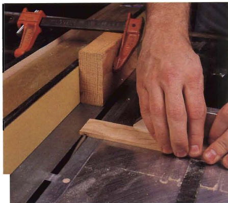
Figure 2: When crosscutting or dadoing the slats, always use a spacer block to prevent the wood from binding between the fence and blade.
