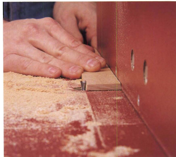
Figure 1: Bevel one edge on 26 slats while they are slightly oversized, then reset the fence to bevel the second side on 22 of these slats. Remember to always approach the bit so that it is rotating into the stock, which in this case is from the left.
