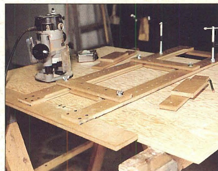
After the stops are bolted in place, the adjustable frame guide is tightly clamped to the work piece.
