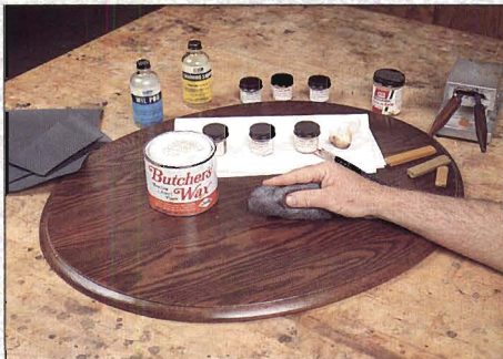
Step 4: The last step is to match the sheen to the rest of the finish, using either 400 grit wet and dry compound or steel wool, depending on your piece.
