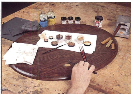
Step 1: Get started by using your burn-in knife to re-establish the grain lines in your repair area.
