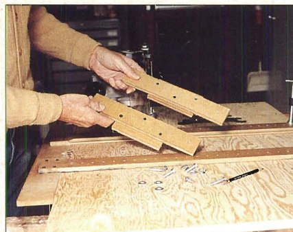
When you screw the stops to the cross arms, be sure the overhangs are exactly 1/4", 1/2" and 3/4", so you can stop dados in 1/4" increments.
