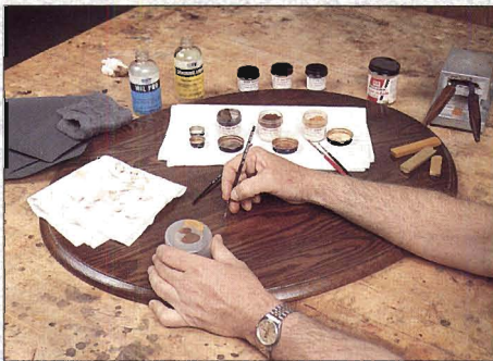
Step 3: Once the color matches, a fine brush is used to randomly draw in the fine grain lines.
