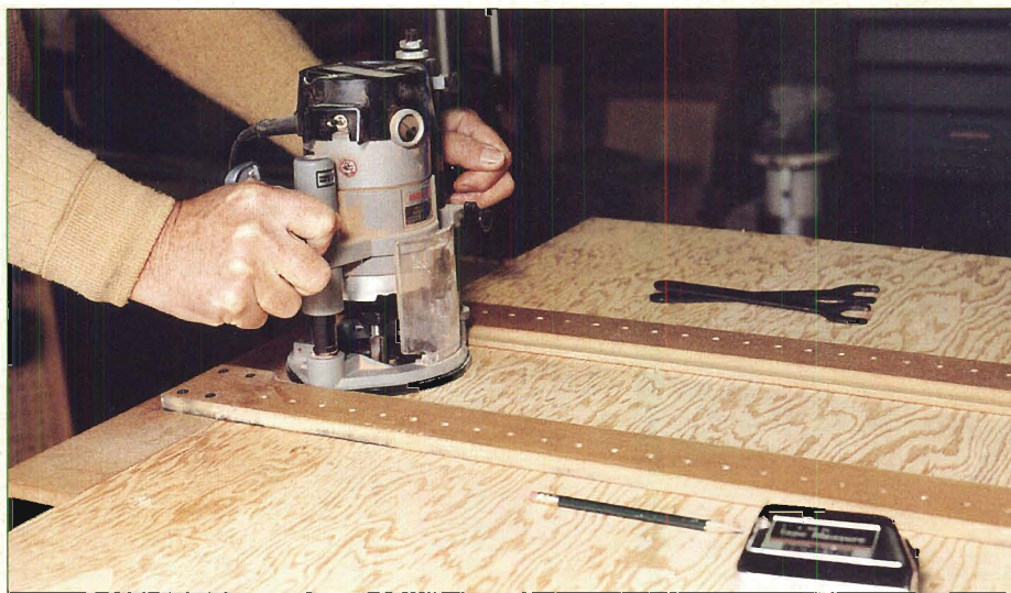
The router frame guide will keep your router bit exactly where you want it to be.
