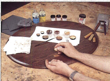
Step 2: Next, use your finger to gently wipe on the powdered stain and lightly apply the padding lacquer with a lint free cloth.
