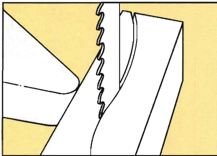
A pivot block fence allows the operator to stay on track by pivoting the back end of the workpiece. This fence is particularly useful when cutting curved stock.
