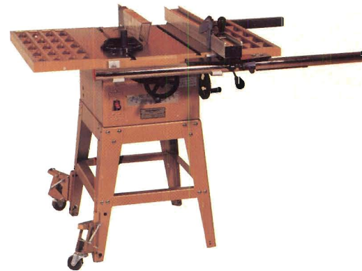
This Powermatic tablesaw (top) addresses a couple of age old woodworker concerns—an accurate fence and integrated dust control.
