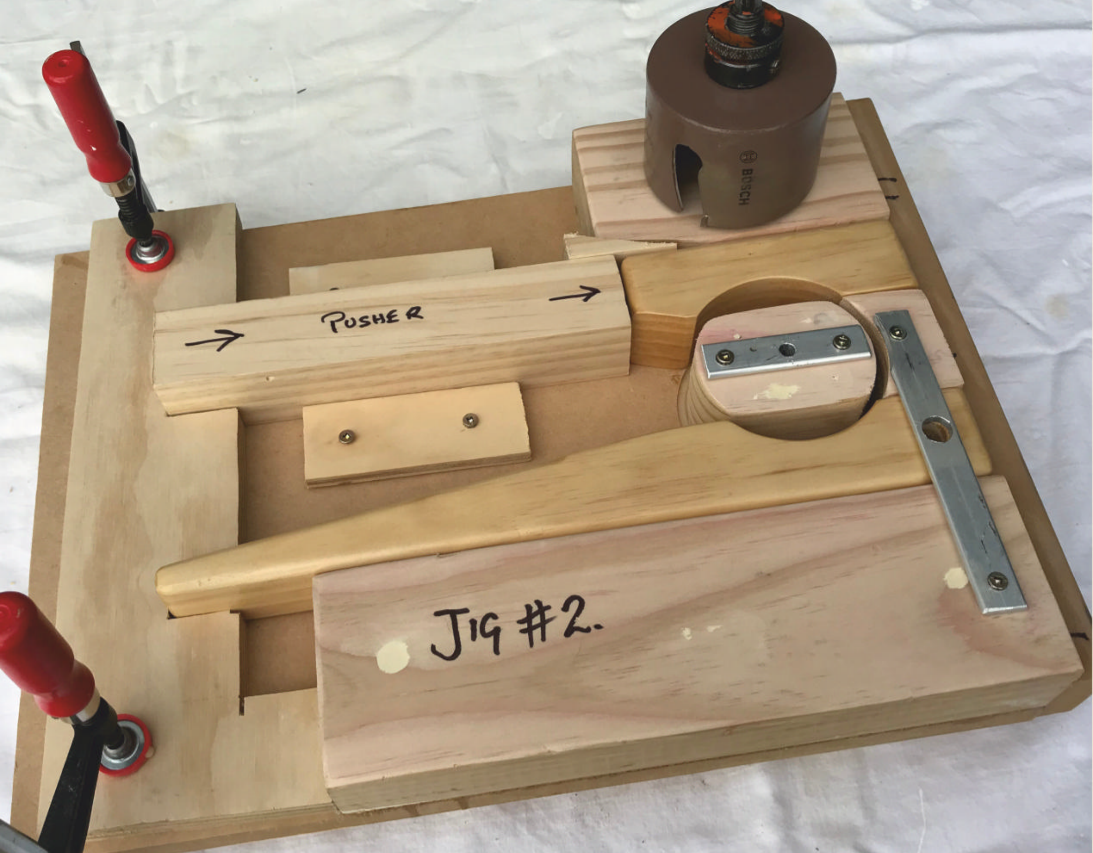
Image 10. Production jig No. 2 for cutting the 90mm gripping form and the pivot hole
