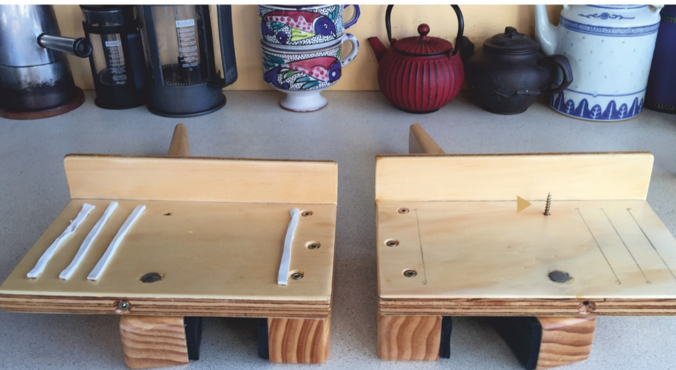
Image 12. Semi-permanent mounting: (left) the base is held by four strips of butyl rubber; (right) the base is held down onto the bench with a 38mm screw
