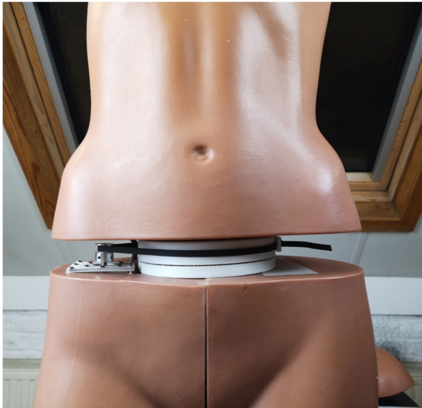
The final assembly of the body with the new mechanics for the rotation. When I finished this part, all the remaining components were developed and tested from inside the small cavity of the torso
