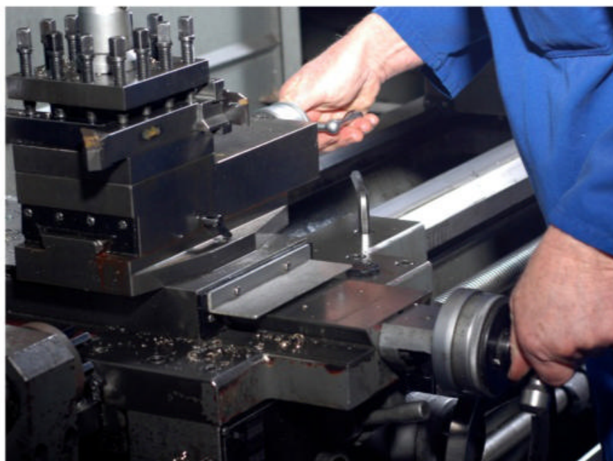
Turning both the cross slide and compound slide handles simultaneously
