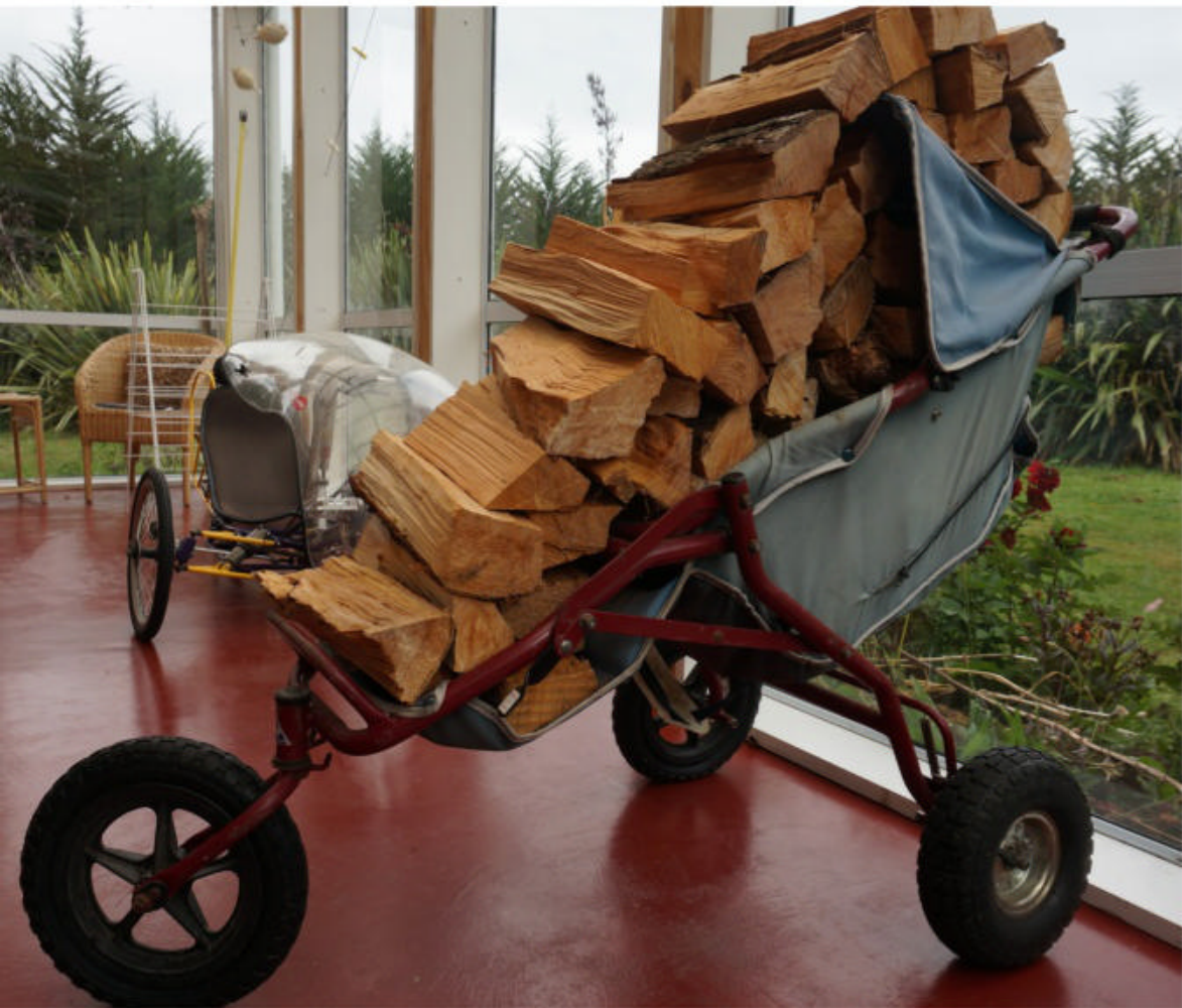
An acrylic bath, a couple of tubes and a pair of BMX wheels: our most-used wheelbarrow
