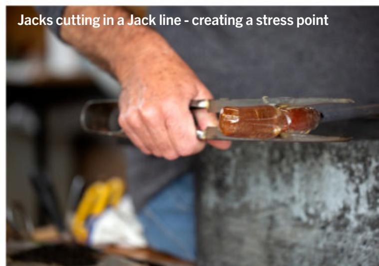
Shears cutting a hair-line in the glass head
