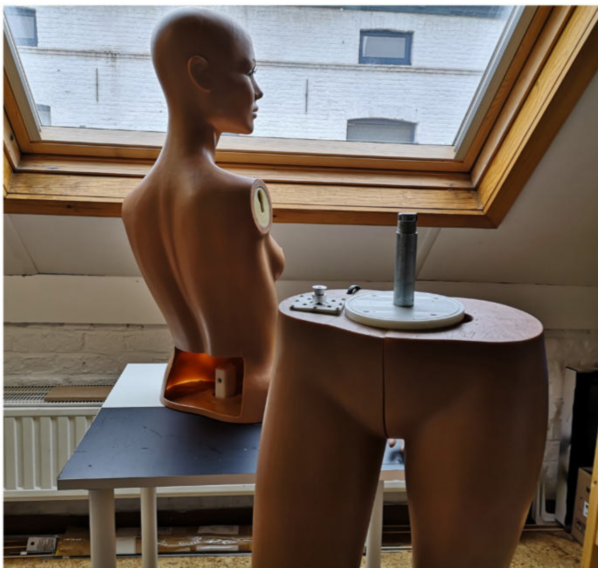
The top surface of the legs. To the left there is the 20-tooth pulley fixed to the stepper motor shaft, while the central position is to the non-rotating side of the lazy Susan bearing. The top part will be fixed to the torso for the upper body rotation. The diameter of the 3D-printed bearing can support the weight of the torso for a fluid rotation. Note the vertical shaft at the centre of the bearing that will hold the torso part
