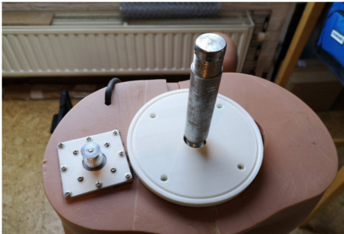
The top surface of the legs. To the left there is the 20-tooth pulley fixed to the stepper motor shaft, while the central position is to the non-rotating side of the lazy Susan bearing. The top part will be fixed to the torso for the upper body rotation. The diameter of the 3D-printed bearing can support the weight of the torso for a fluid rotation. Note the vertical shaft at the centre of the bearing that will hold the torso part
