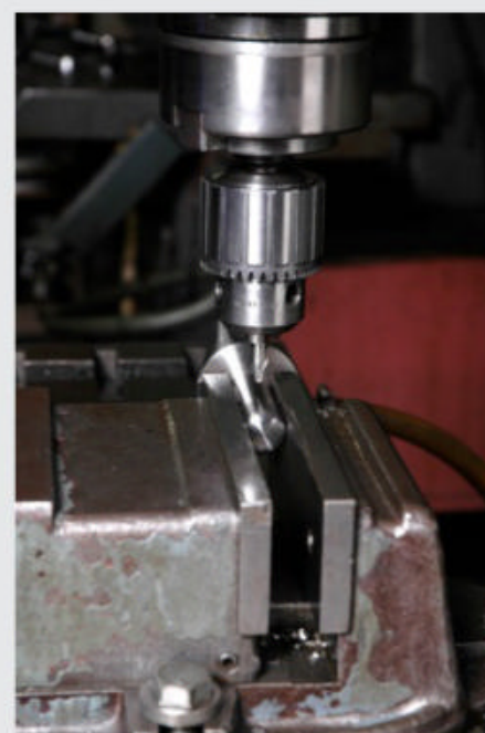
Pilot hole boring
