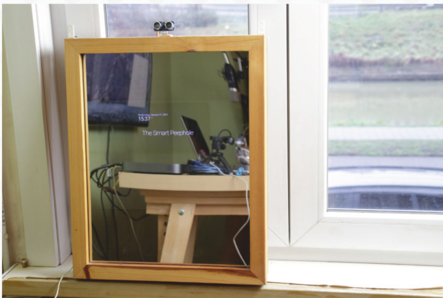
The image shows an example of the sequence of different textual screens shown by the smart peephole. The text strings are shown by a module that is configured to change the text randomly from a list every five to ten seconds, with a fade-in, fade-out effect; to the left: the camera triggered by the sensor covering the screen
