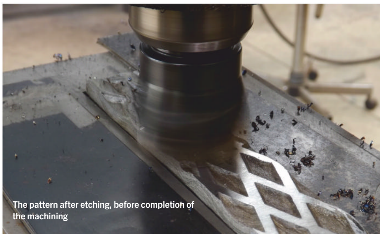
The pattern after etching, before completion of the machining
