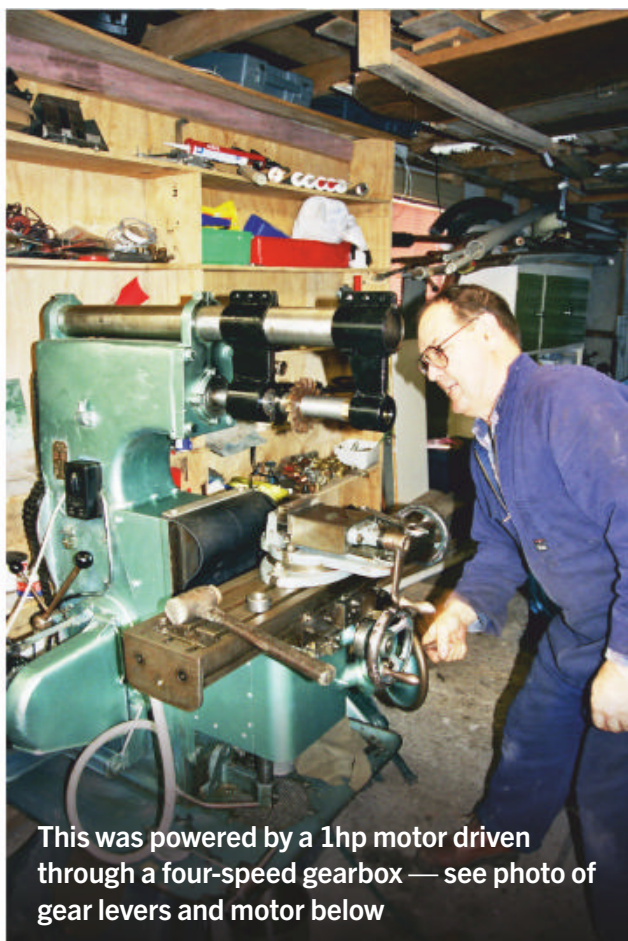
The quill is 3.375-inch diameter with a 5-inch stroke; this has turned out to be very beneficial for serious drilling up to 1.250-inch diameter
