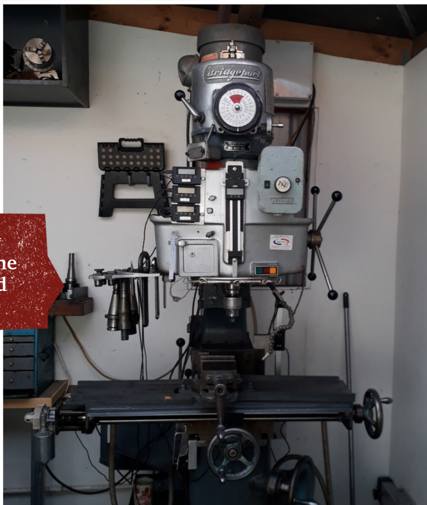
The milling machine, showing the wiper-motor drive on the left-hand end of the table
