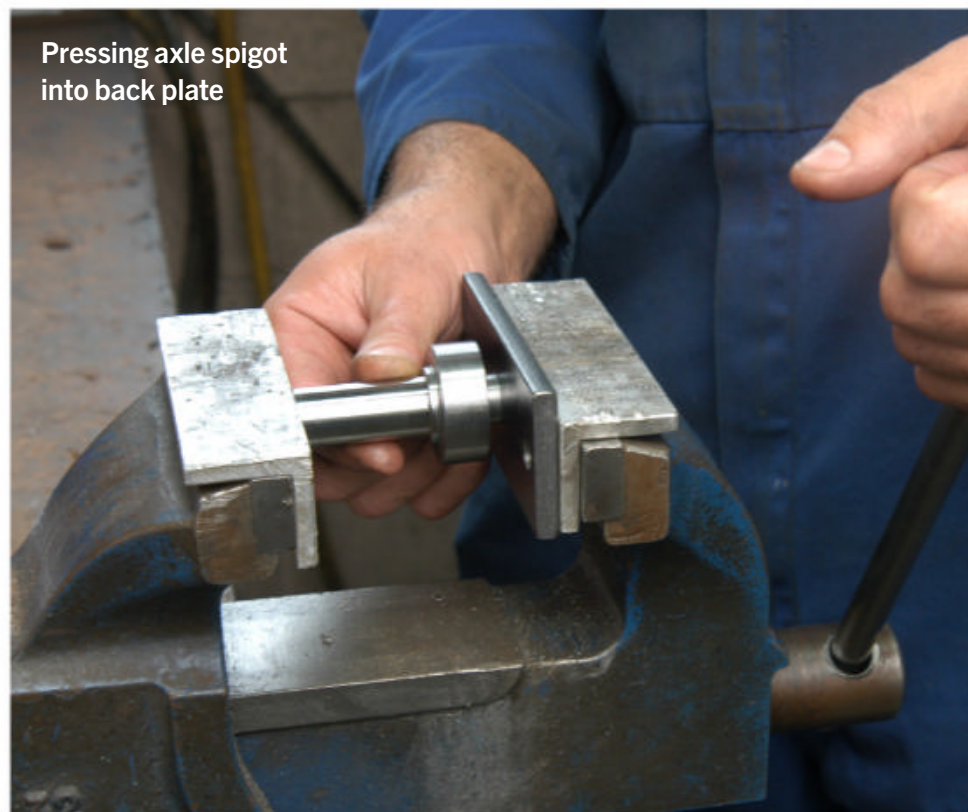
Protect from chuck marks with aluminium drink can strip
