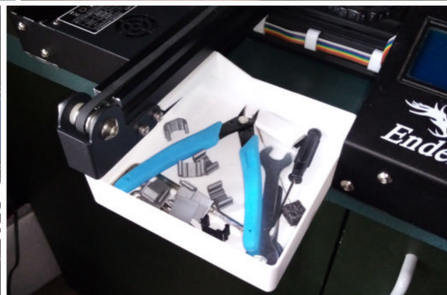
Finished tray fresh off the printer with support structures still in place; these can be cut off with a sharp knife. Support structures can be switched on and off by ticking or unticking a box in the print settings of the slicer
