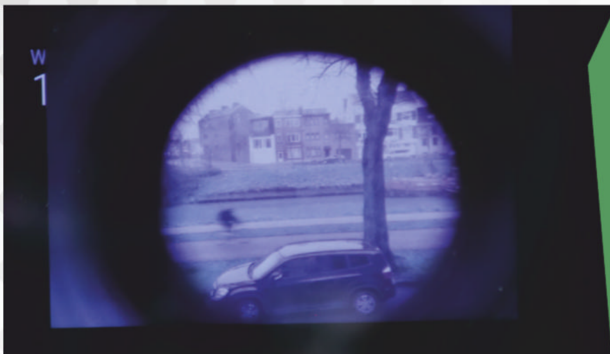
Detail of the Pi camera showing the outside image with the classic 'peephole' effect. It is not a software effect, but the camera with the peephole lens mounted on top of the fixed-focus lens. Most of the quality of the image depends on the quality of the peephole's extra lenses. I strongly recommend using a good-quality product with glass lenses to achieve the best result
