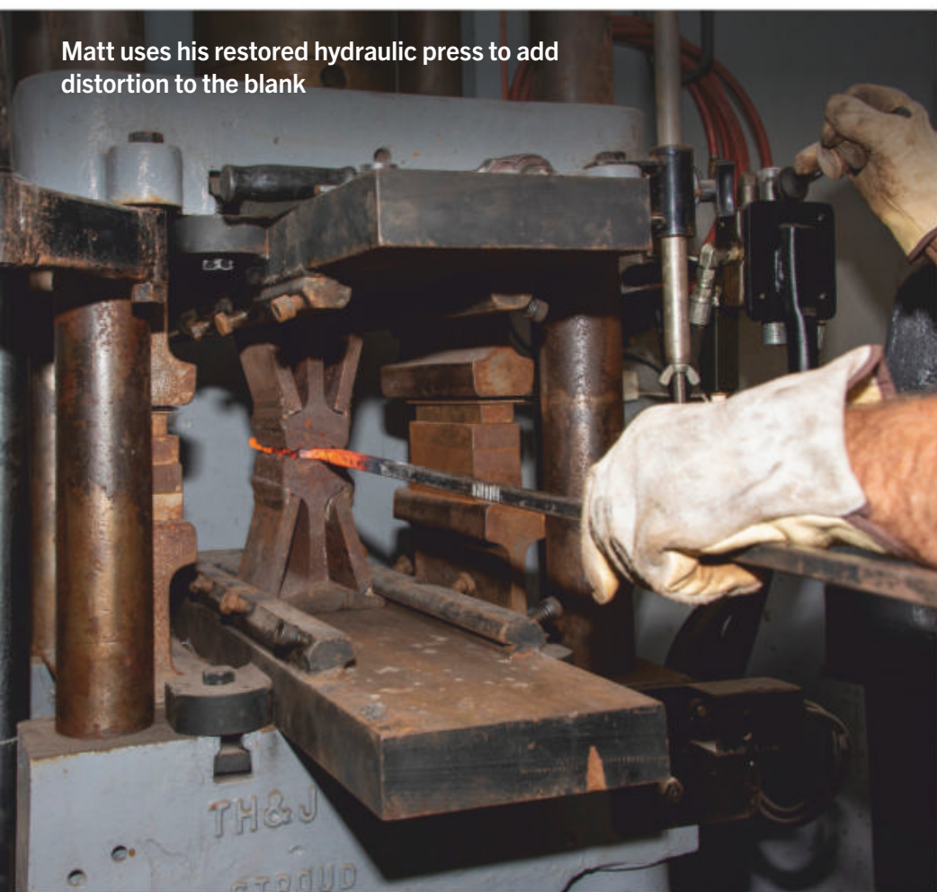
The pattern that becomes devil's darts after machining
