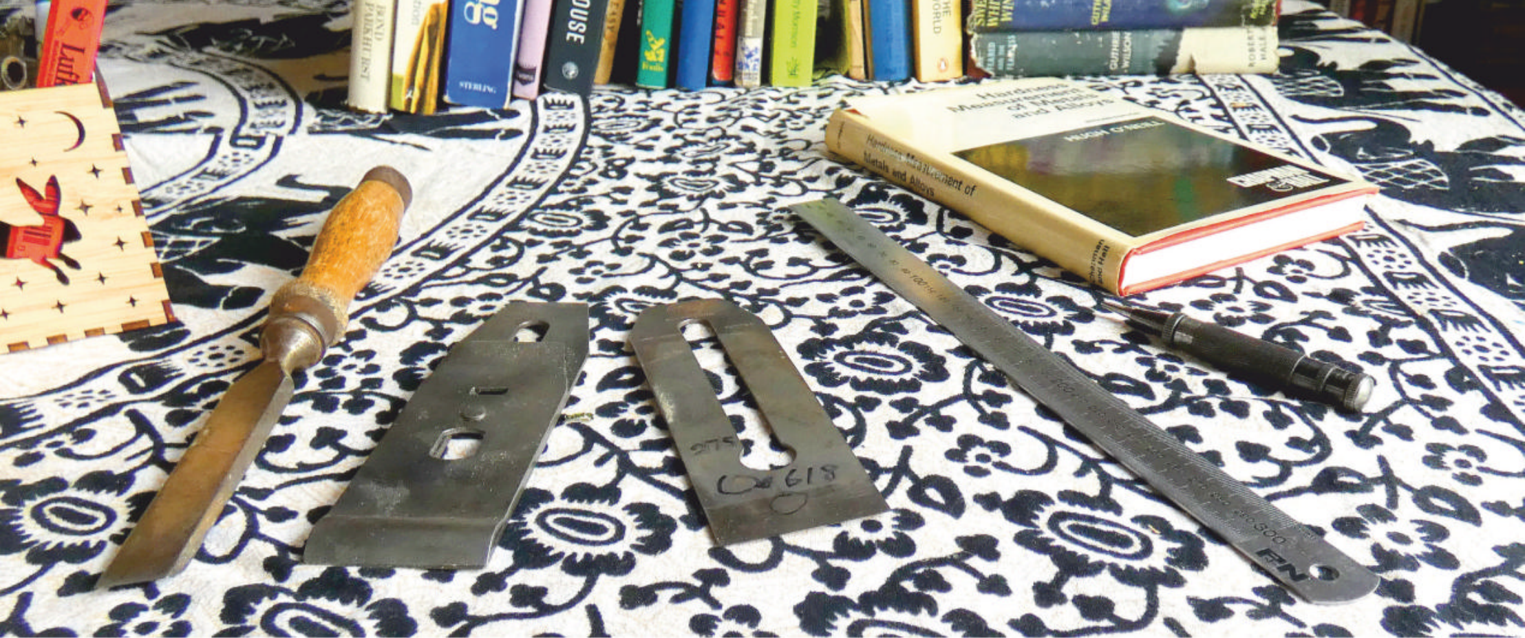
A Falcon-brand plane cutter flanked by a Titan Tools plane cutter (showing the different steel at the cutting edge) and firmer chisel. A firmer chisel has square sides
