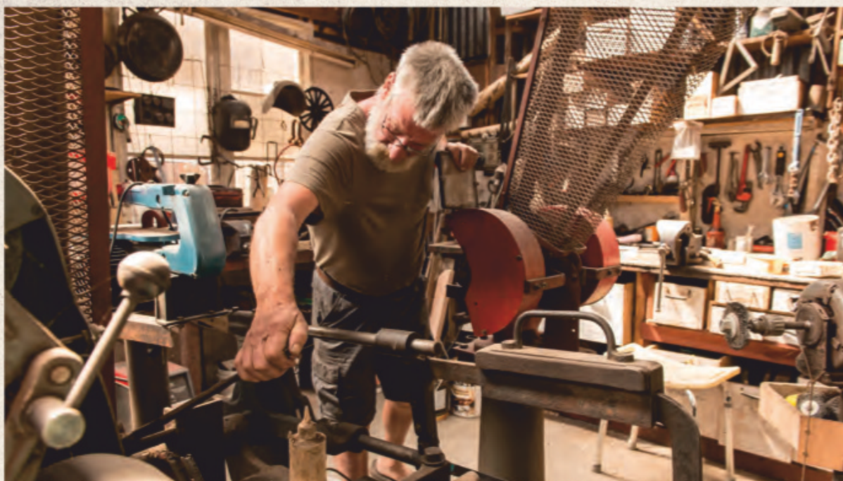
Bruce Chapman pulling in the dog clutch to drive the 1904 power hacksaw
