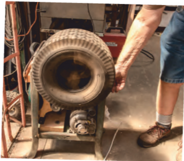
Max Hyde checking out the ‘new’ tumbler, hand built by Bruce Chapman from items lying around in his shed. There is stone and steel shot in the tyre and it is used to remove rust and scale from nuts, bolts, and other small items
