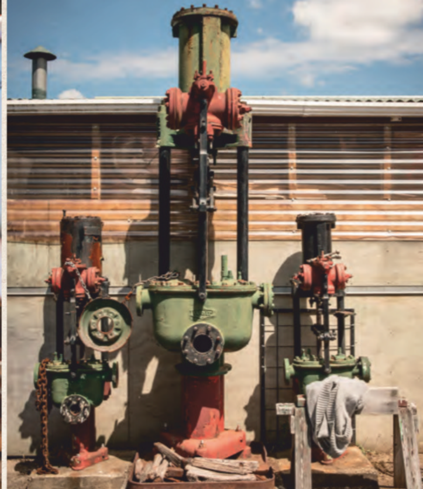
The museum has six Weir pumps, three of them attached to an 8hp Anderson boiler. Weir is a Scottish firm that still makes pumps, mostly hydraulic
