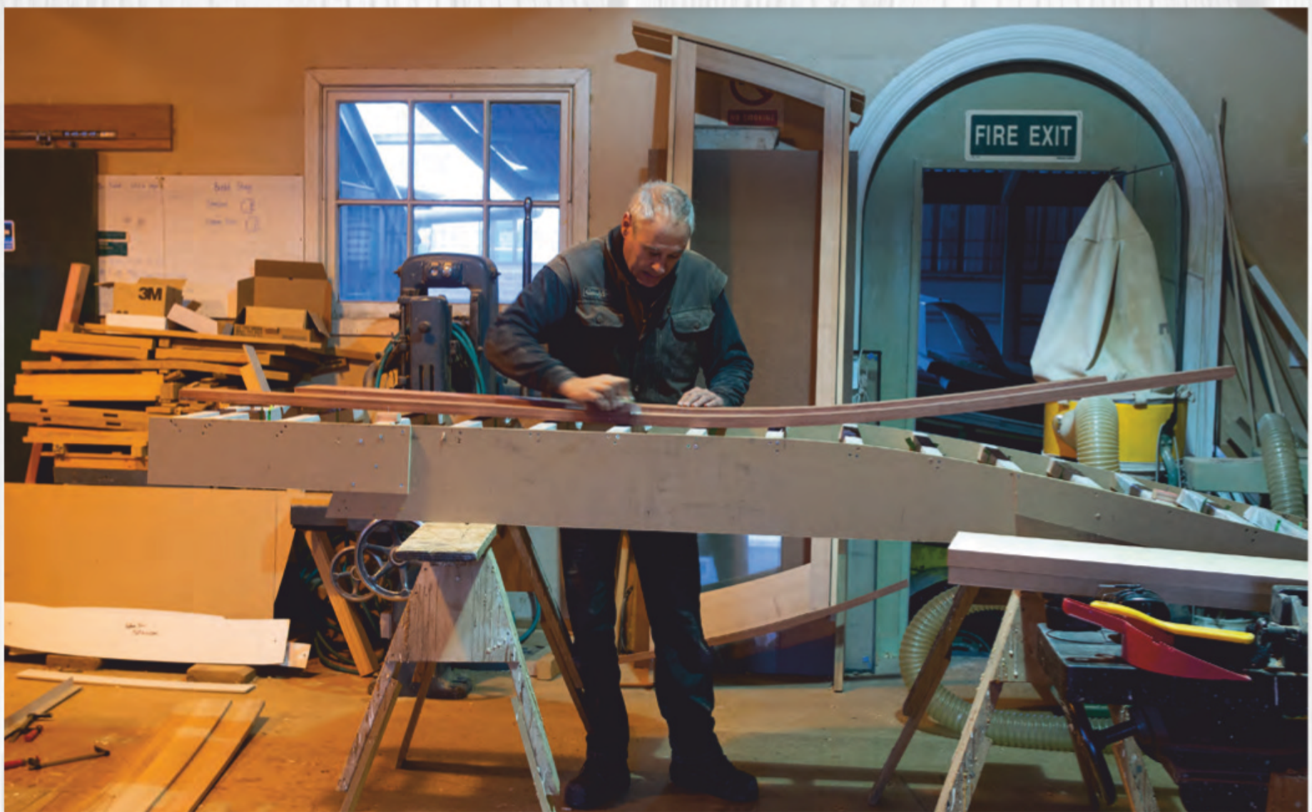
Sanding a curved jarrah window sill that has been removed from the curved jig underneath
