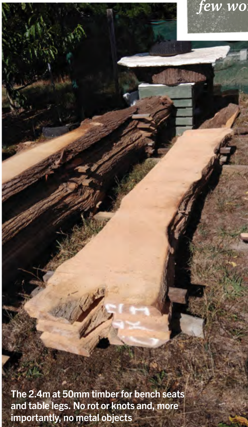
Of the four trees dropped, one yielded some nice straight pieces that were trucked to the mill. Some were converted to 200x100, and two others were flitched at 75mm and 50mm to be used for tables and bench seats. The 200x100 timber — these are 6m long from two branches of the fourth tree
