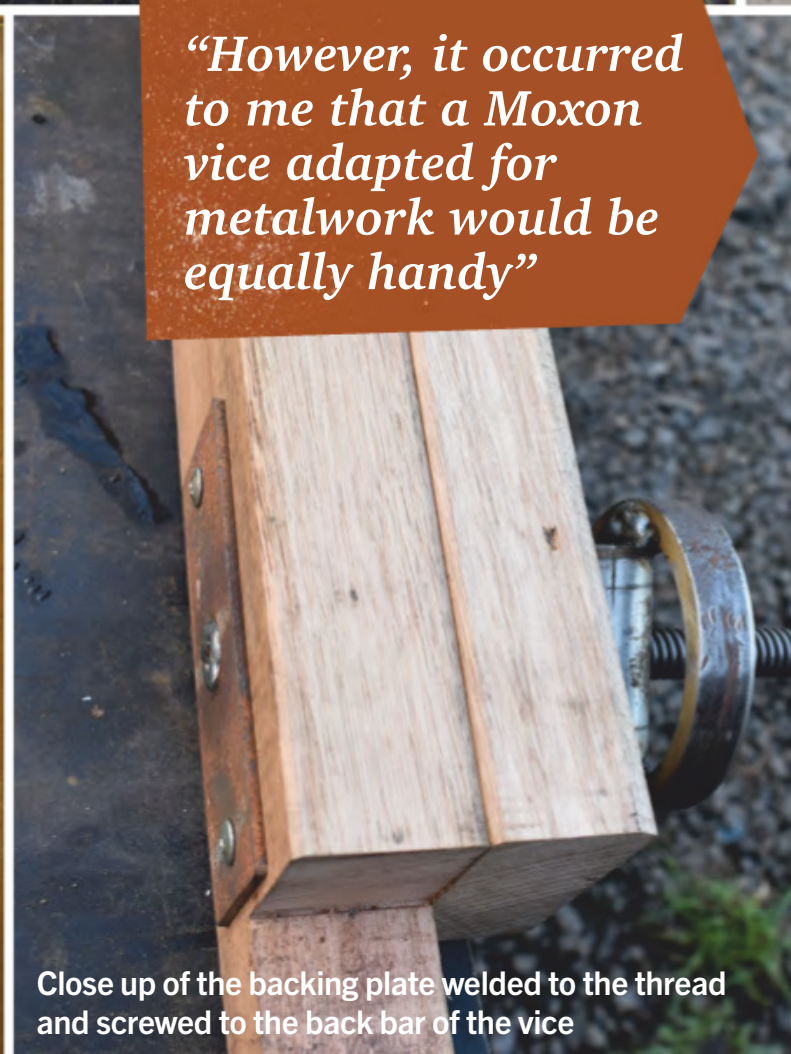
Ring welded onto the nut block to make using the vice a bit easier
