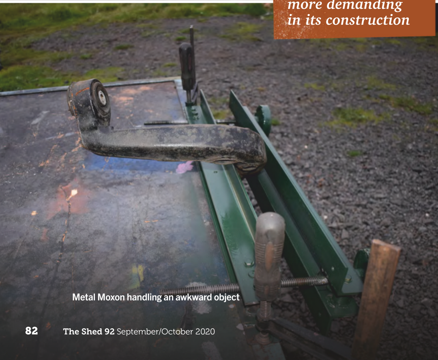
Close up of the screw nut block and the supporting blocks welded in place
