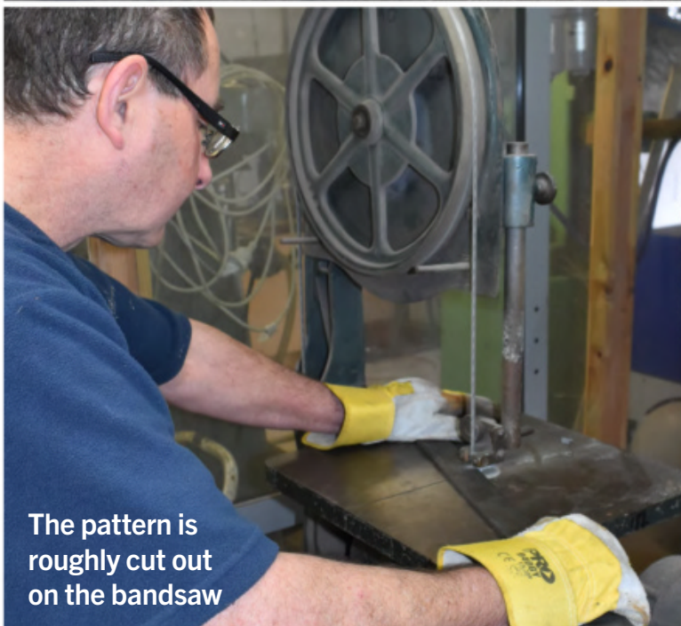
Blanks are stacked and pinned so four can be cut out at once
