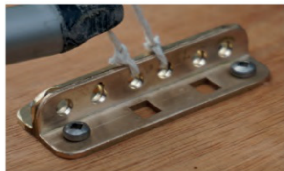
Two brass locks furnished the adjustable jib-stay mount; the jib boom started life as a hang-glider batten
