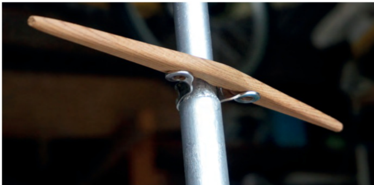
Ski-pole mast and a twisted saddle carrying the cedar spreader
