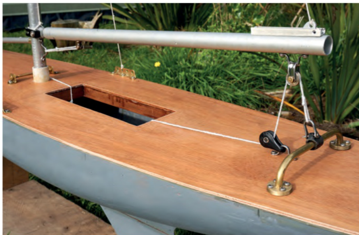
Outhaul filed from a curtain track; traveller was a ballcock arm
