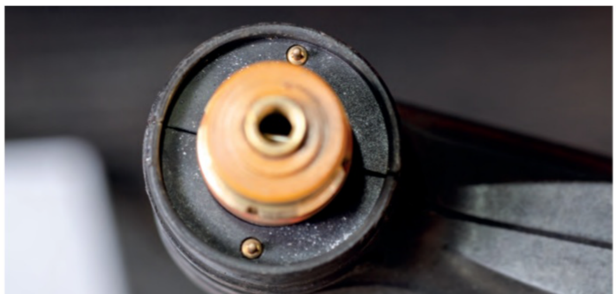
These two pins in the heads are microswitches for the parts-in-place sensor, which helps prevent accidental electrocution when changing electrodes
