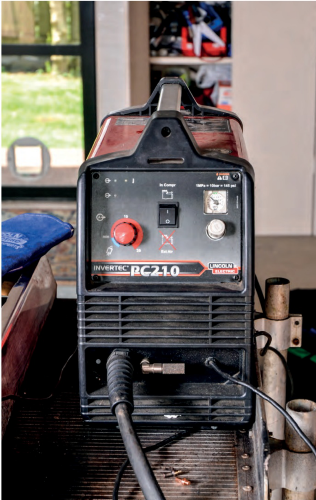
The front panel on the Lincoln Electric Invertec PC210 showing the amperage control and a switch to turn the internal compressor on or off
