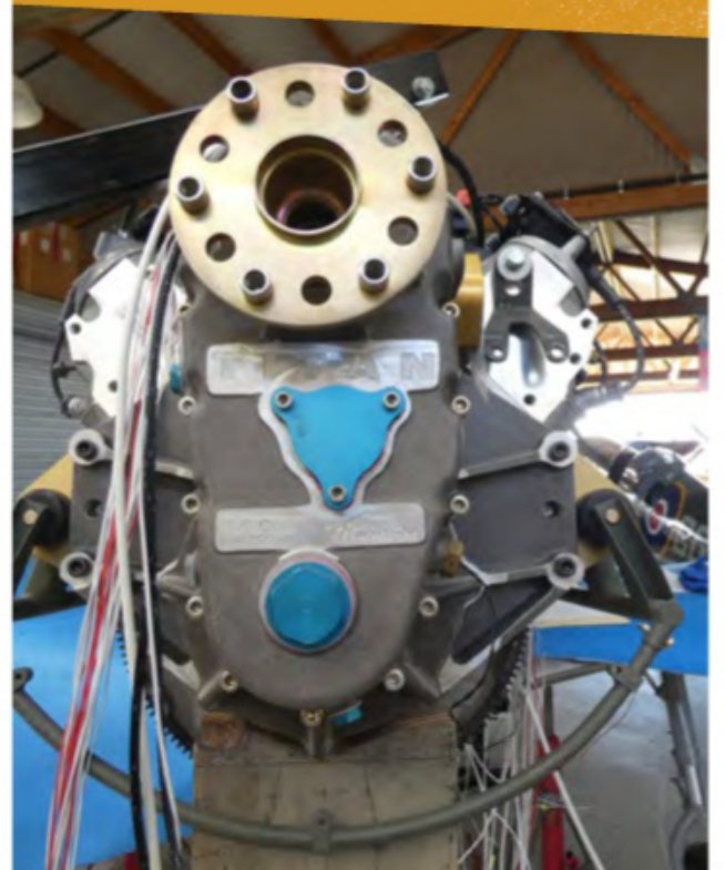
The New Zealand-made reduction gear incorporating two rubber belts
