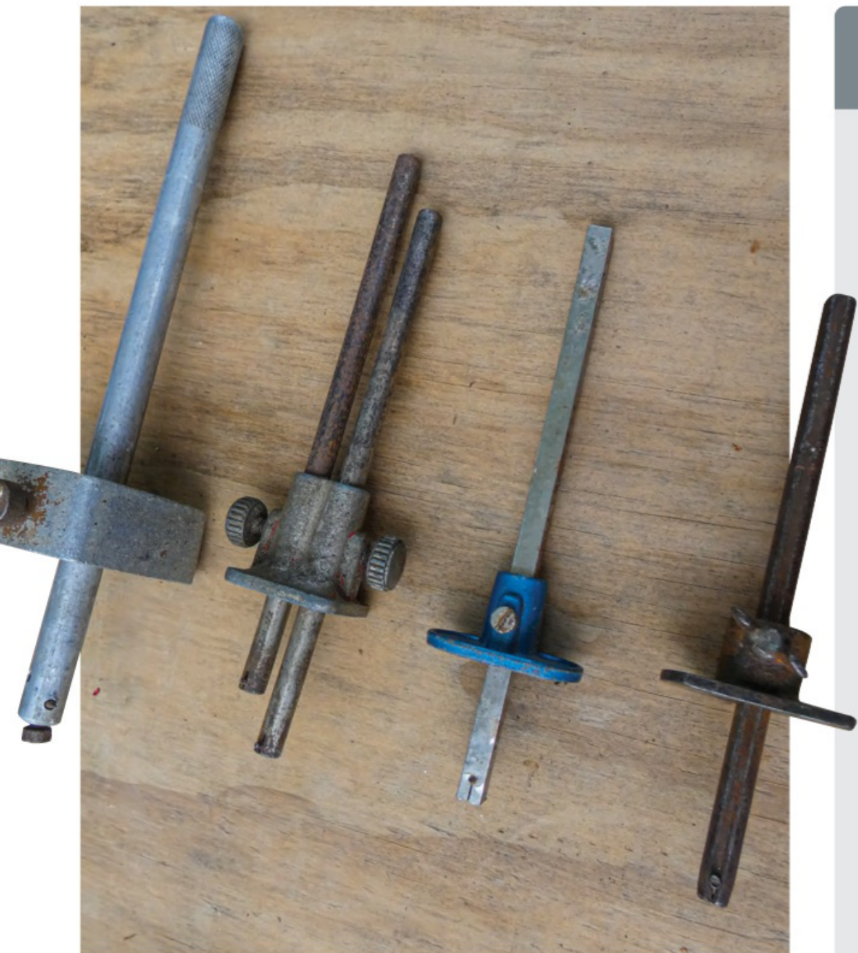
Four marking gauges — the two in the middle are factory made; the left and right ones are craftsman made. The left one is made from aluminium; the right one is made of steel. The steel one has a fence made from steel components brazed together. The steel rod has a groove nicely milled in it. The mortise gauge — the one with two rods — is another Silex Tools product
