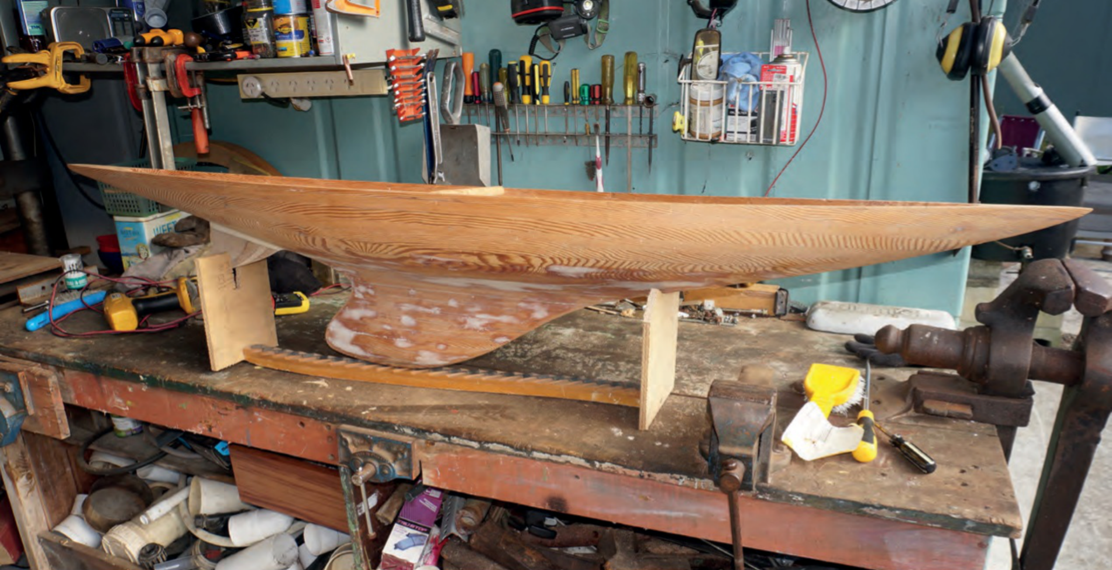
The hull as inherited, in my 'office'. She is hand-hollowed from a stack of cedar planks
