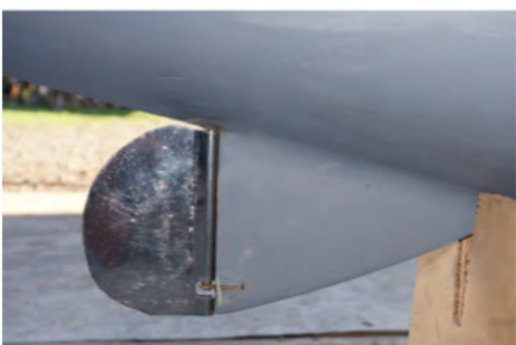
Rudder is of stainless sheet wrapped around a stainless drinking straw
