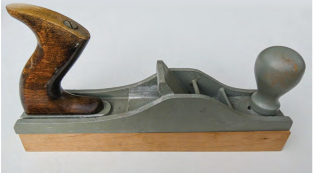
The pattern-maker's plane with replaceable wooden soles; the cutter and its securing clamp are missing
