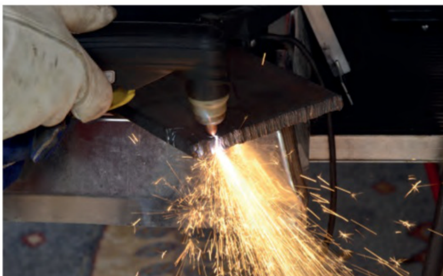
Plasma cutting is one of the fastest means of cutting steel to shape
