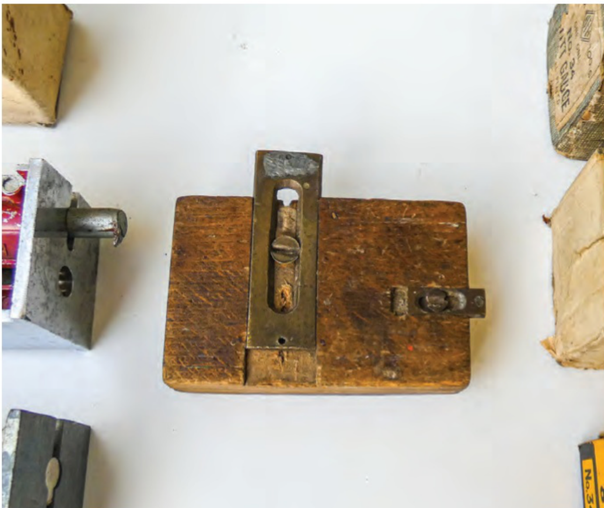
A home-made wooden butt gauge, for marking out the rebates required for installing door hinges, etc. The brass sliding pieces with a steel point soldered to the end move in dovetailed housings in the wood. The settings are kept secure by tightening the screws. Today, electric routers and templates are very widely used to cut hinge rebates quickly, so newer butt gauges often show little use
