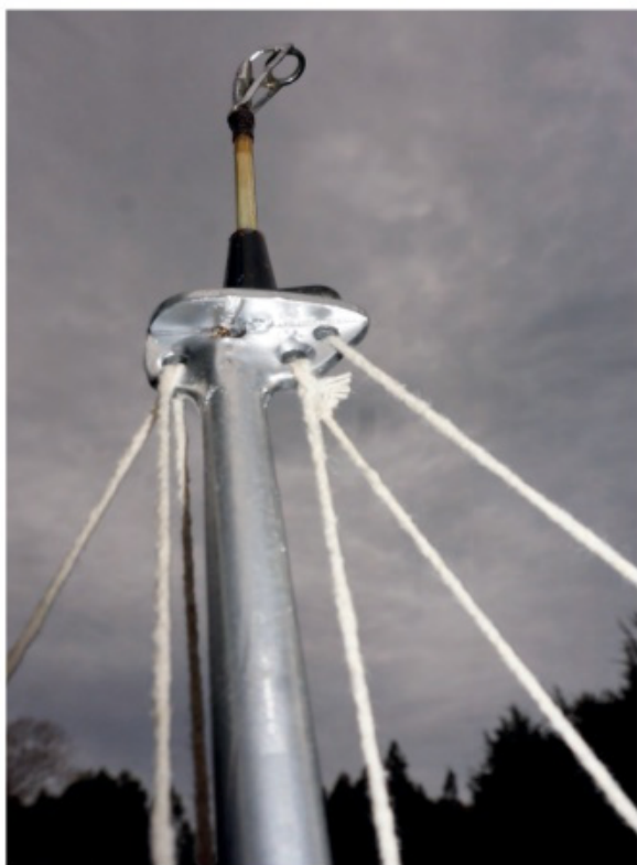
Masthead fitting with trial rigging attached. Having used one end of a fishing rod for the lower mast, it seemed appropriate to use the other as a flagstaff
