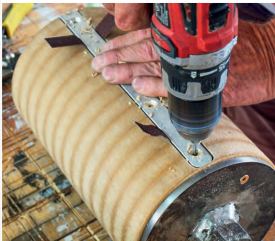
The aluminium strip being checked again by being screwed in place
