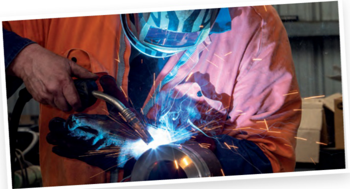
MIG welding is the preferred method of welding on the majority of buggy components
