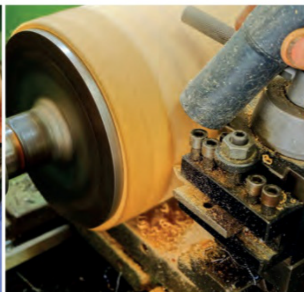
Note the vacuum cleaner being used for dust control
