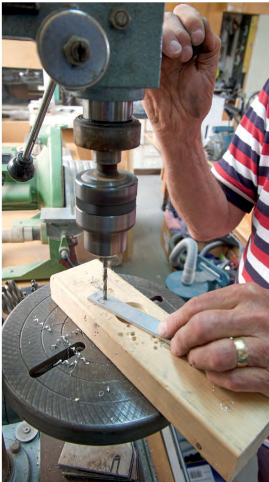
The aluminium strip being drilled
