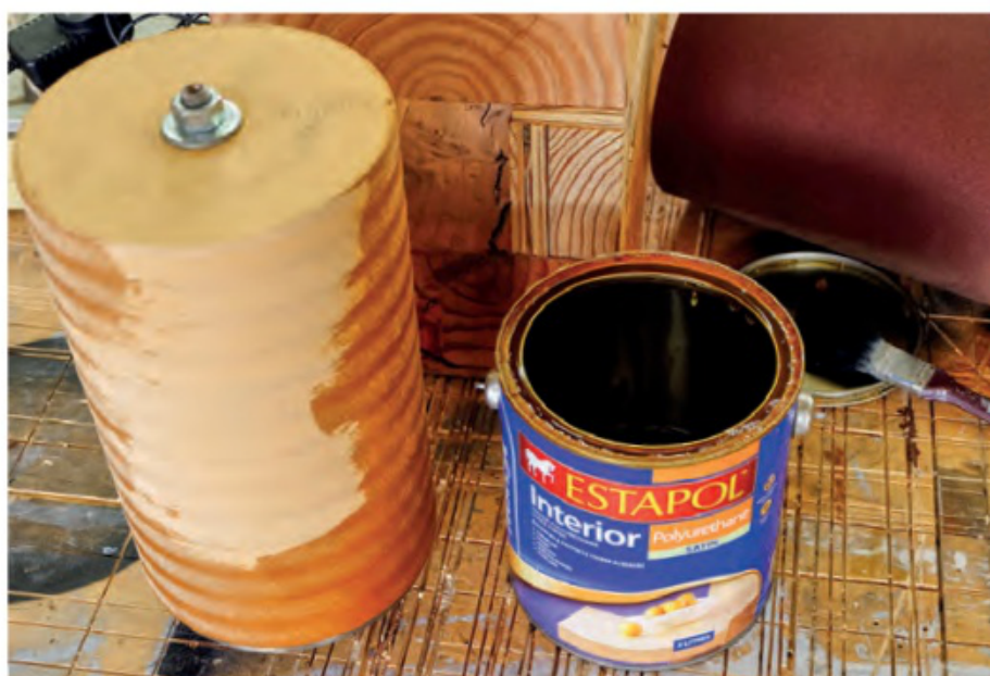
The MDF sander spindle getting a coat of polyurethane to seal it
