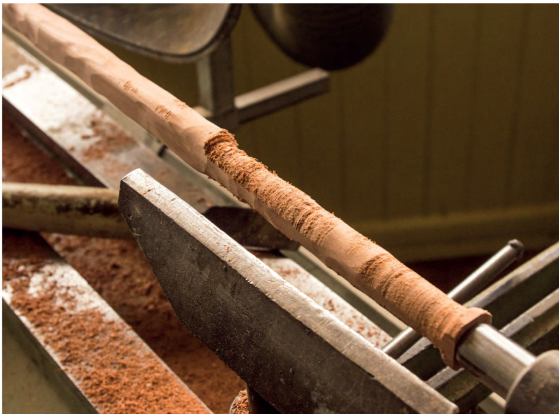
Turning the myrtle cane on the wood lathe
