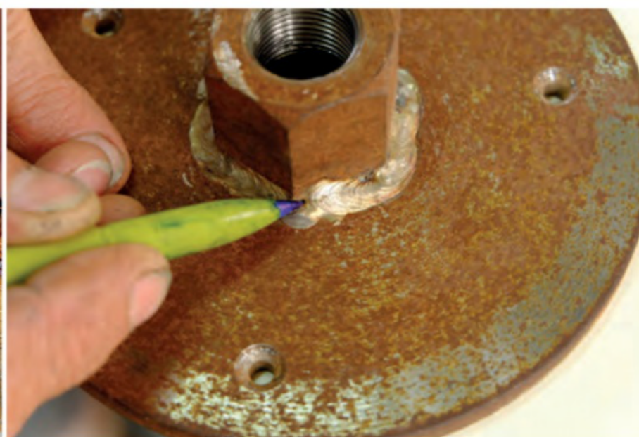
The cracks in the original weld of the faceplate connector
