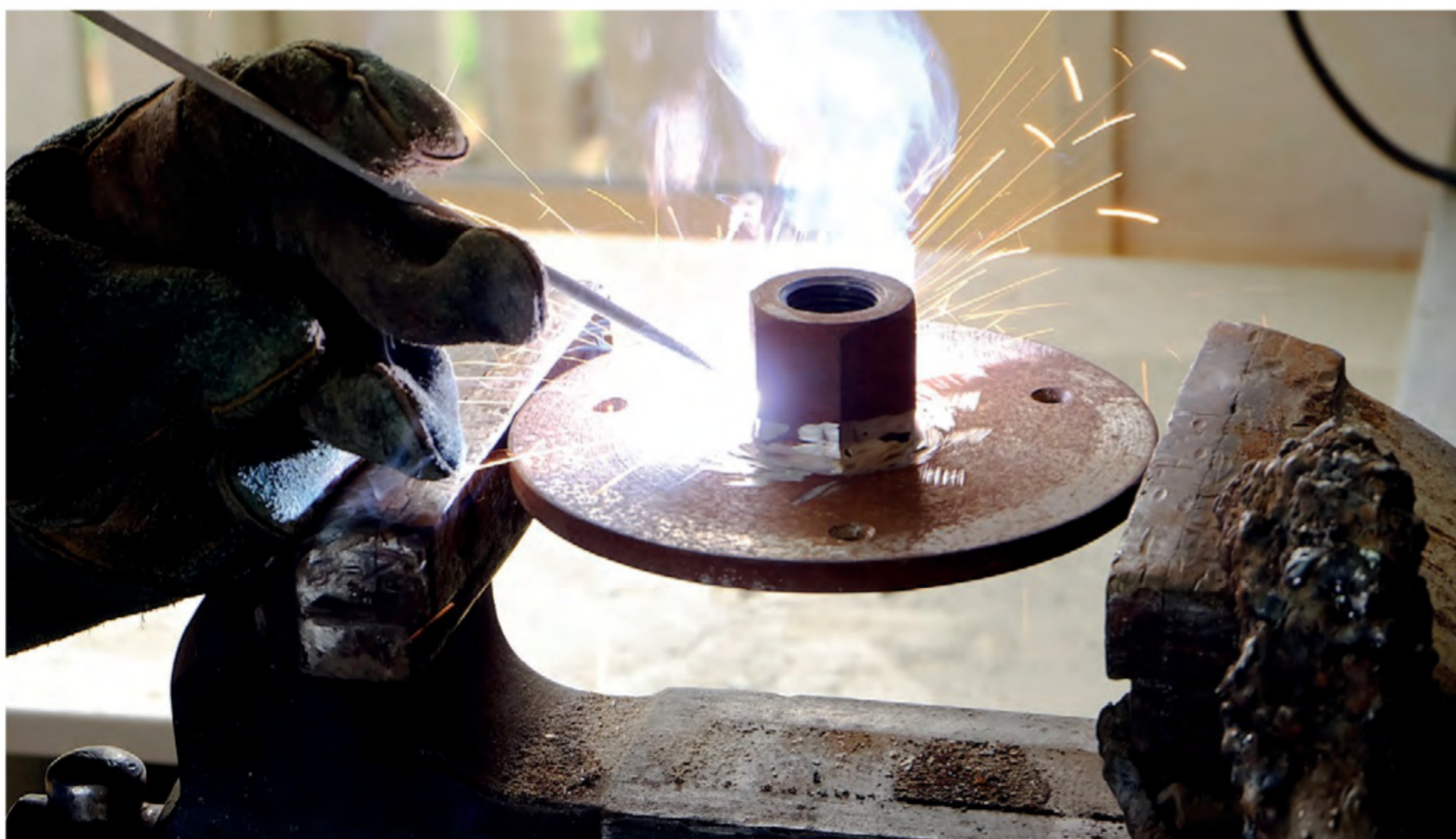
the cracked headstock thread being re-welded
