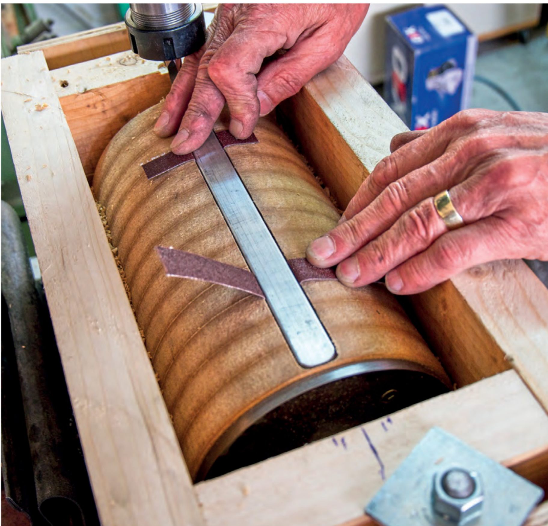
The grooved spindle being 'fitted' with a piece of the recessed aluminium strip over some sandpaper offcuts, to see how well we had done
