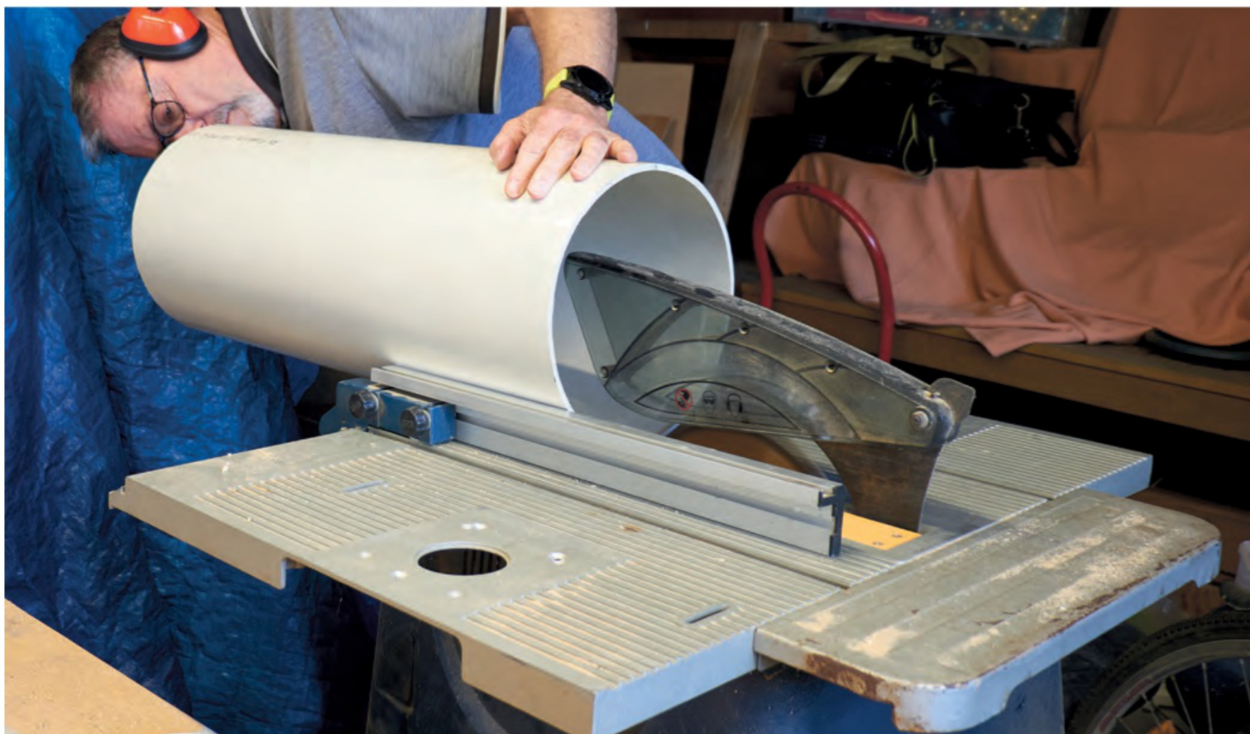
Cutting the PVC pipe — even with ear protectors it was loud
