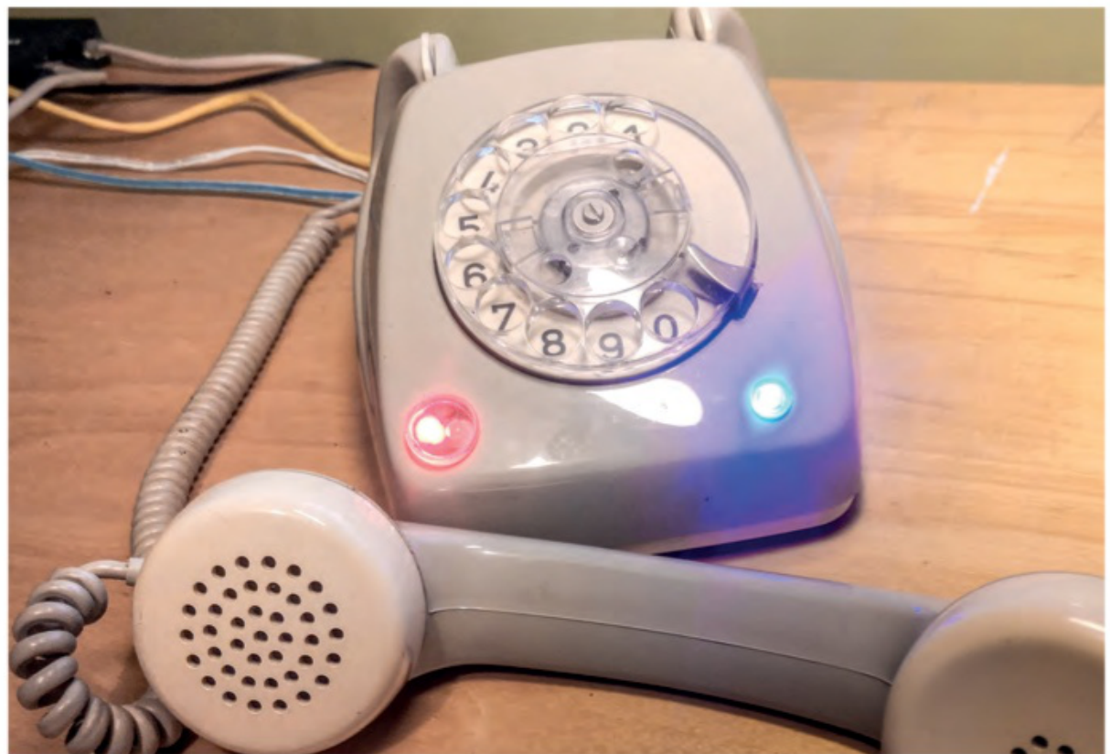
The Pi rotary in action — the blue LED indicates that the system is ready and working, while the red LED indicates that the system can accept numeric commands
