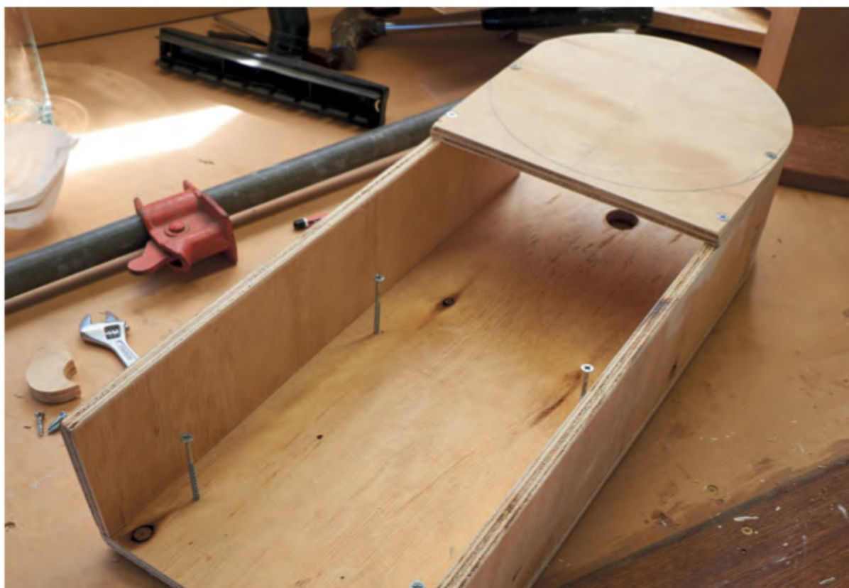
The belt sander cover completed and ready to be installed
