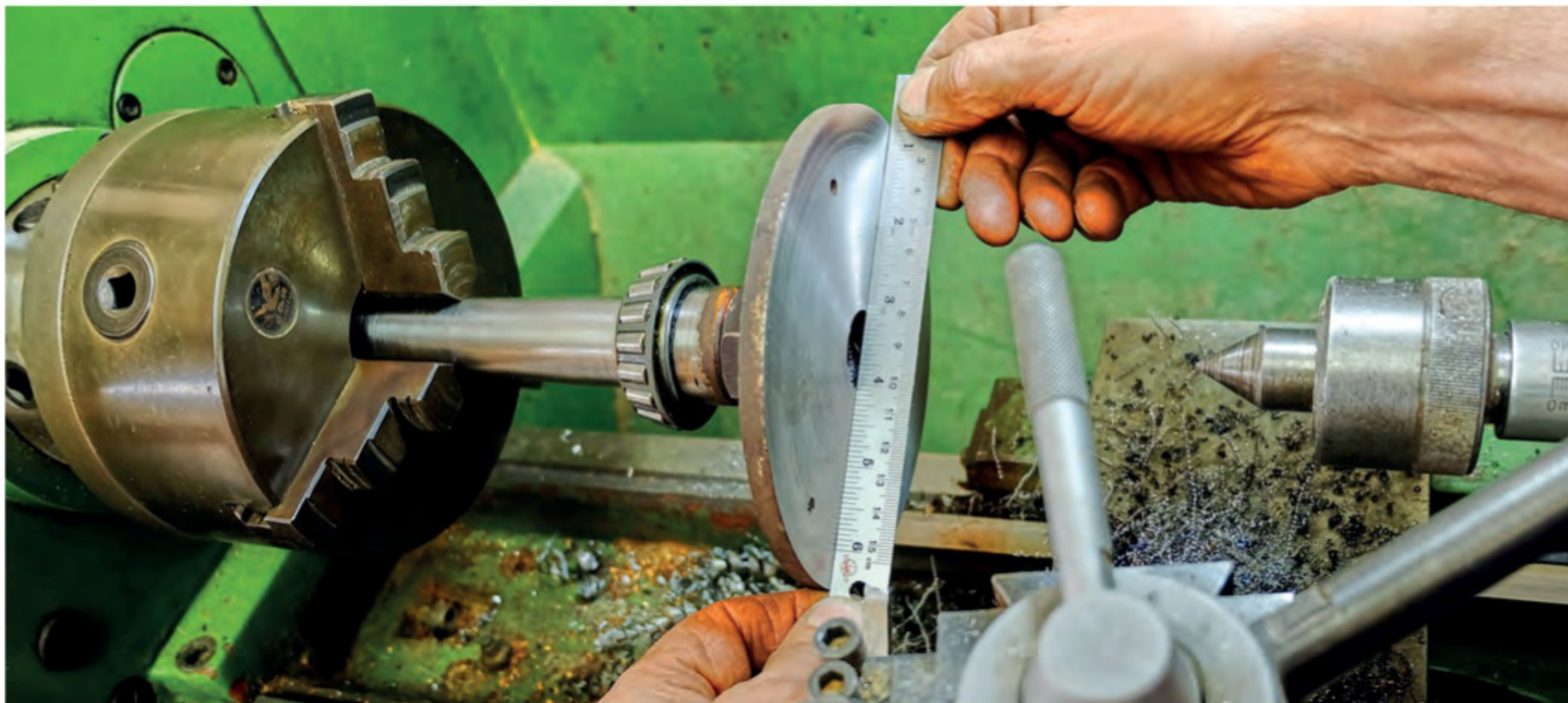
The planed faceplate being checked for accuracy
