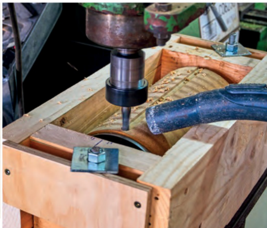
The spindle being grooved with a mill in order to provide the join for the sandpaper
