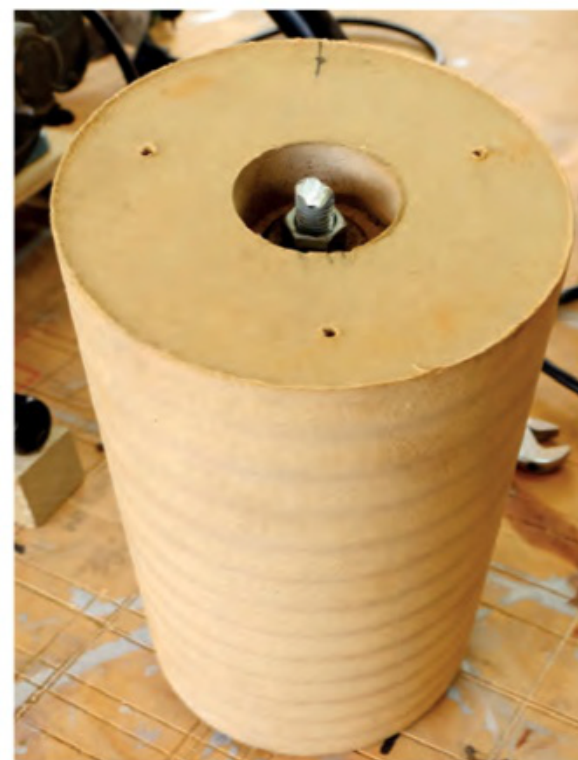
The MDF sander spindle showing the recessed M12 threaded rod
