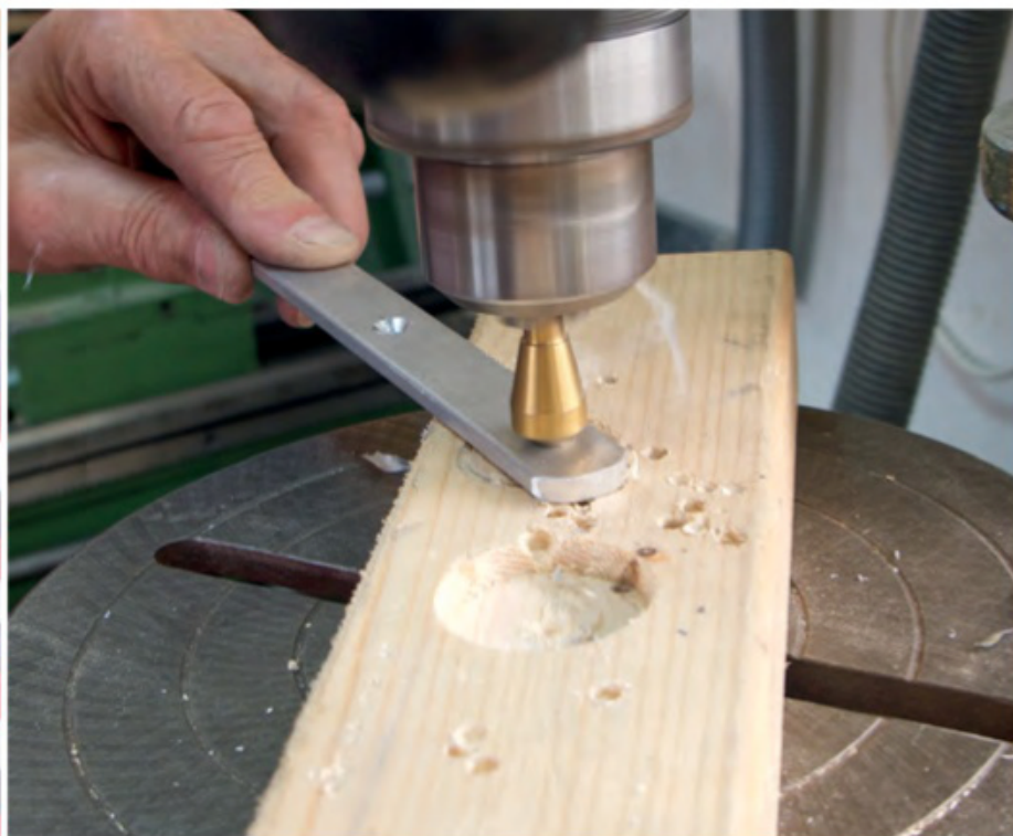
The aluminium strip being countersunk
