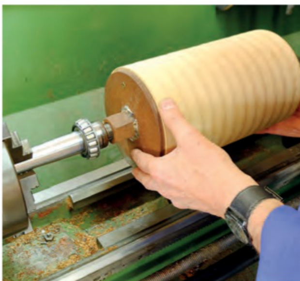
The completed spindle being mounted for machining to remove any wobble
