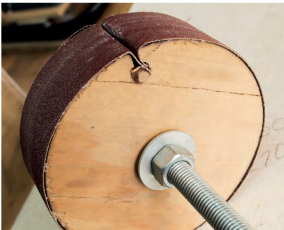
A previous attempt at joining; it was unsuccessful as the dowel used to lock it could not be contained in the right position, with the result that the end was loose
