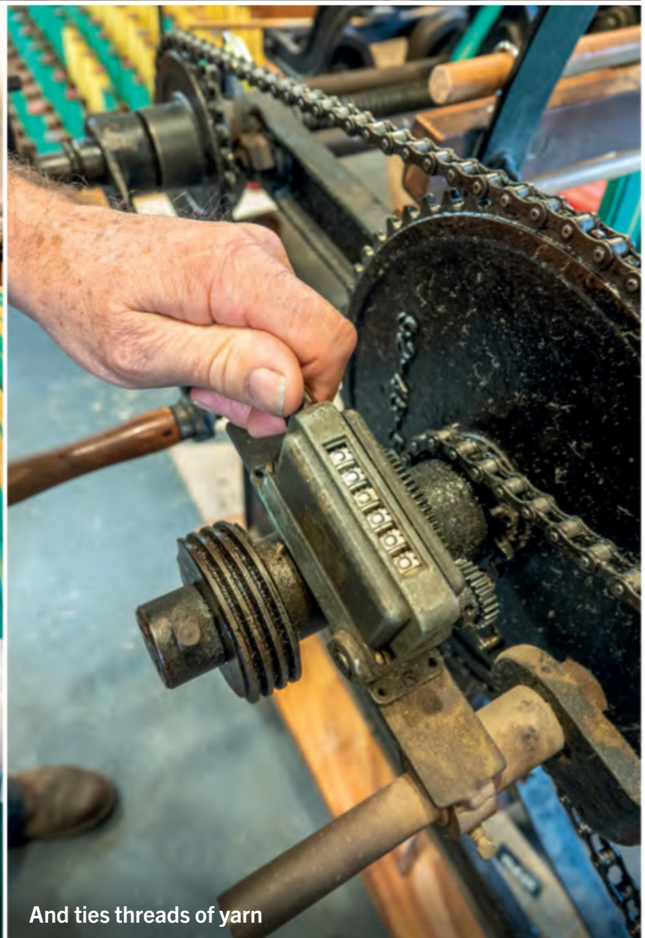
He adjusts the counter to zero in preparation for winding the next section of the warp onto the mill
