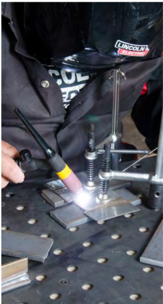
Clamping pieces makes TIG welding easier
