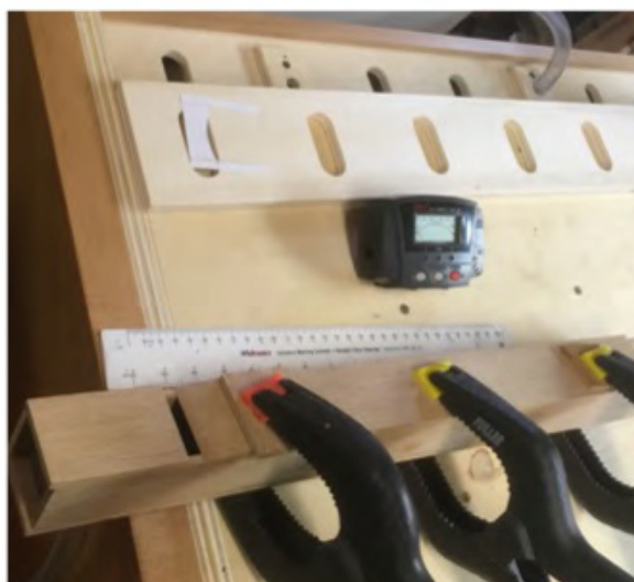
Left: Gluing up an organ pipe
