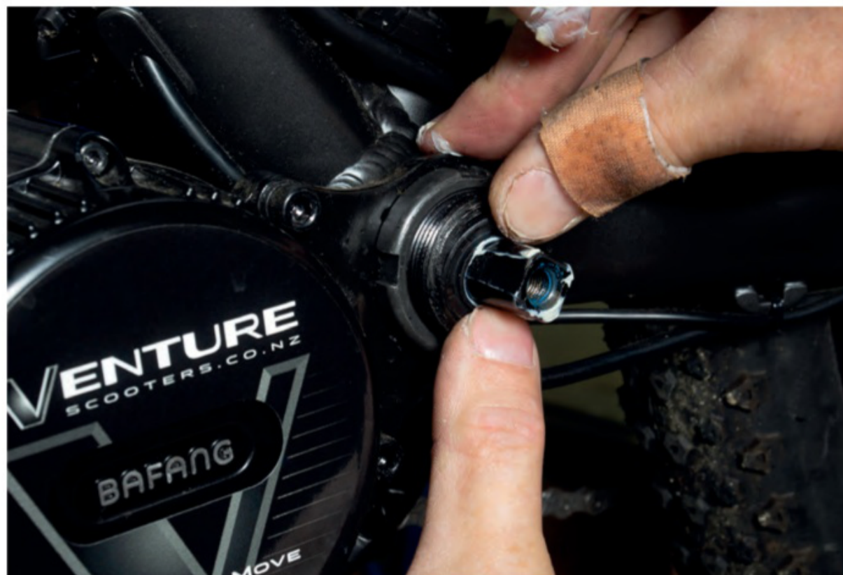
Seal should go in by hand
