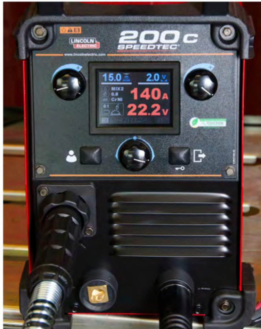
Typical settings for fillet welding 5mm stainless
