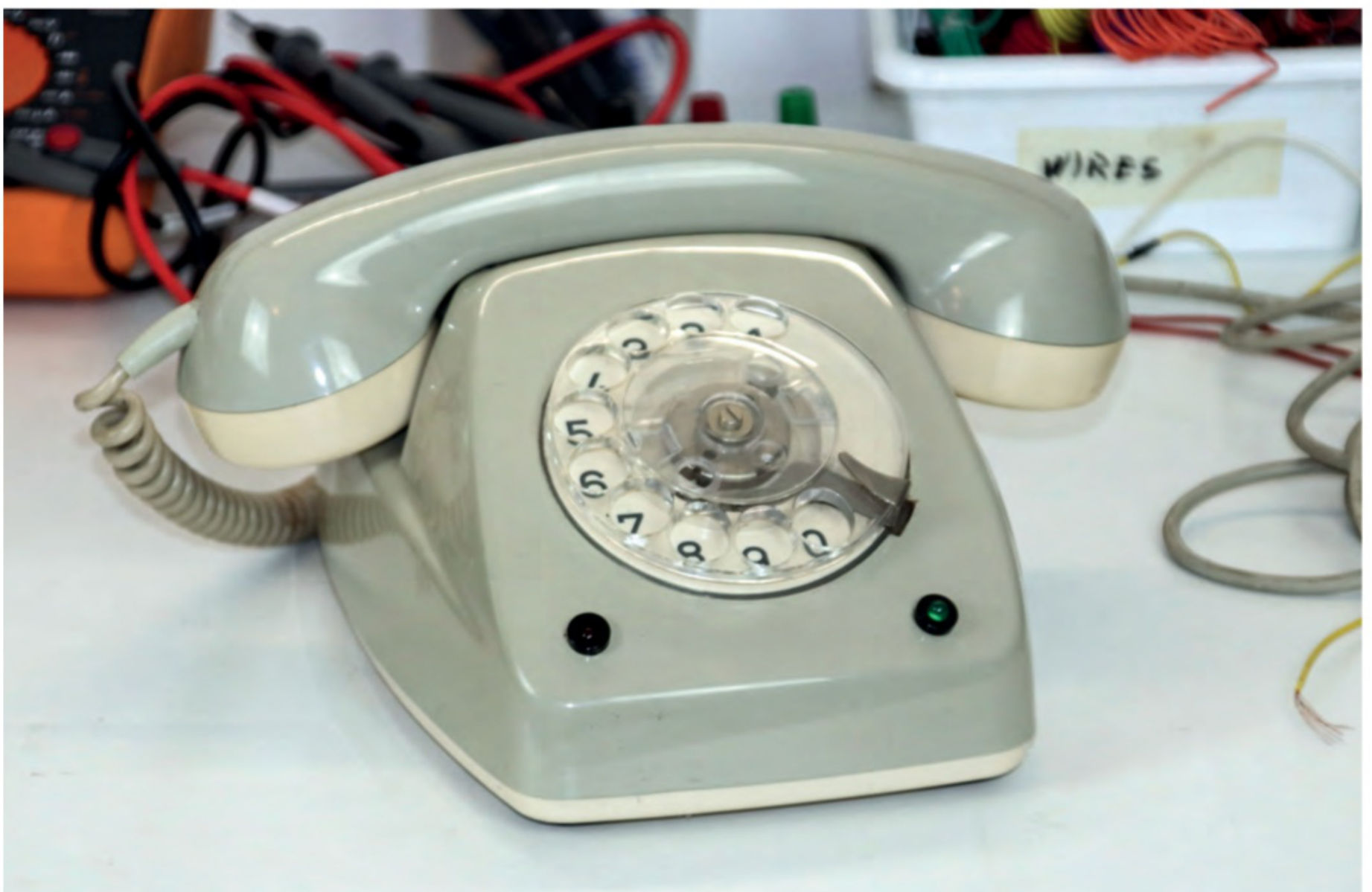
The vintage rotary phone before upcycling. Note that there are also two LEDs — possibly the result of a past customization — that will be removed. The final version will also include three new LEDs controlled by the Raspberry Pi that monitors the hang-up switch and the rotary dial status
