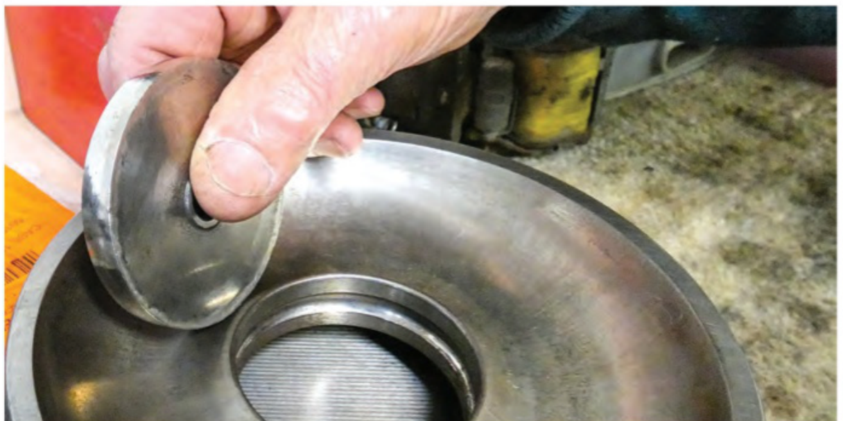
Transmission torus and one roller in the orientation to give low ratio
