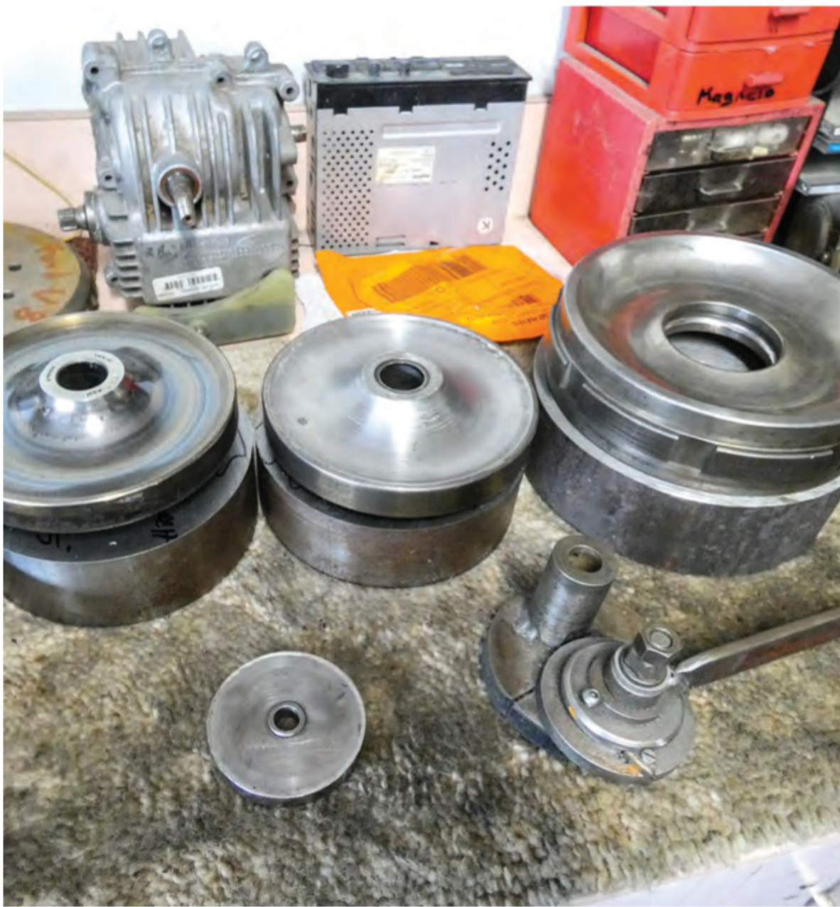
Tori on top of steel pieces which Bob will make into their replacements. Next to the roller in the foreground is the lathe tool made to machine the constant radii curvature of the tori
