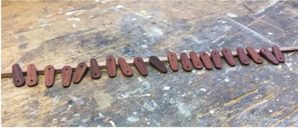
Left: The kwila clips that hold the pipes in place Below: One of the cloth flaps that acts as a valve Bottom: Pipe installation
