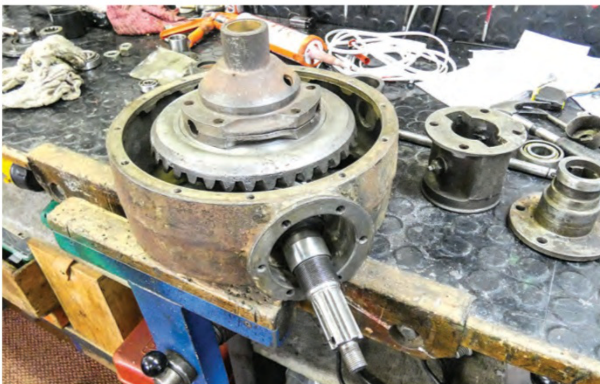
Ford V8 crown wheel and pinion (CWP) — the raw material for the new Austin back end parts
