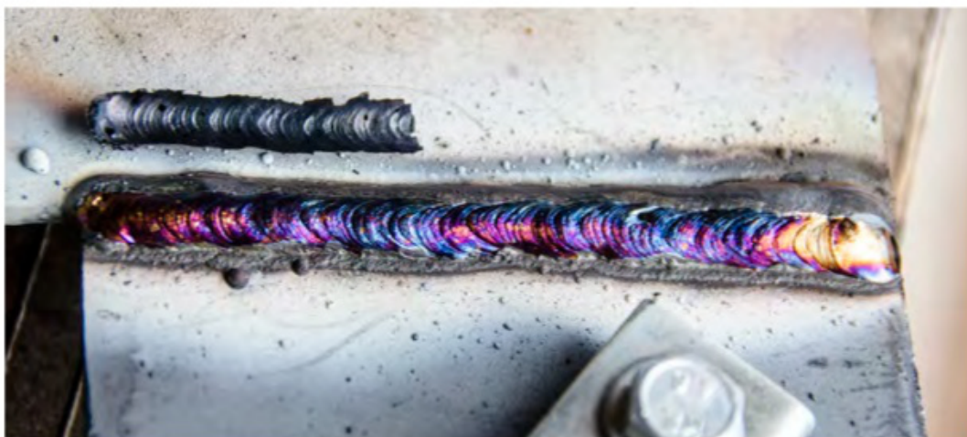
Arc weld on stainless steel. Note the glassy slag and the typical colour
