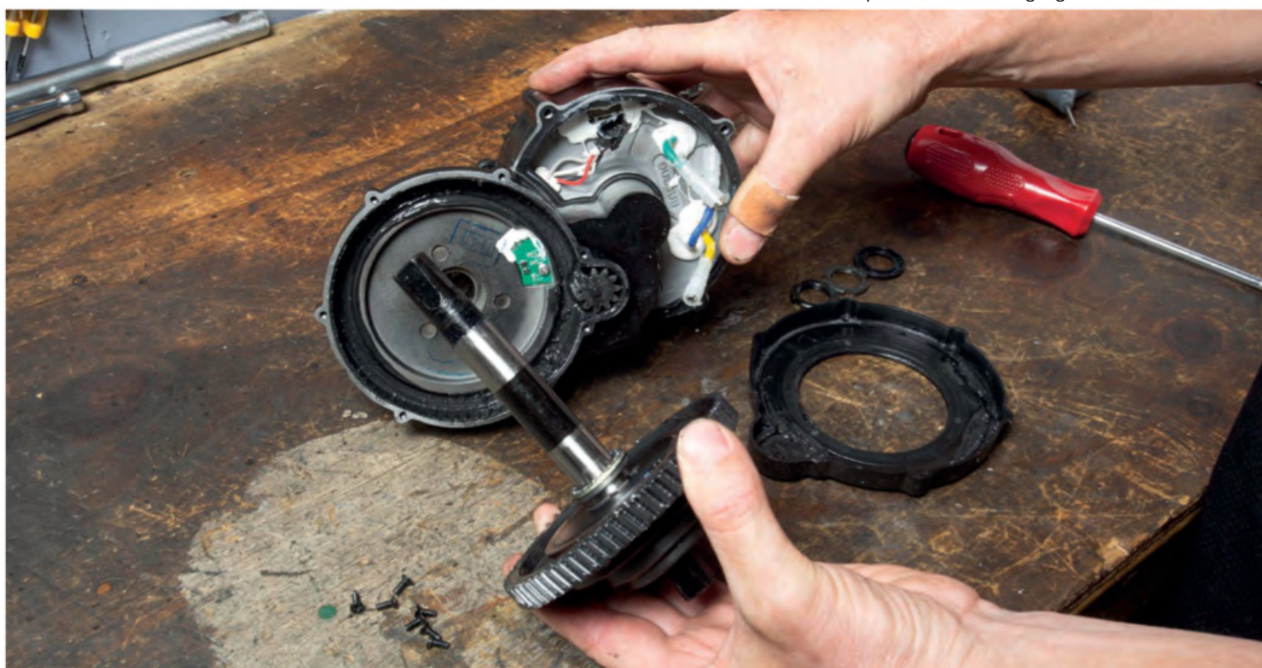
Removing axle and main drive gear
