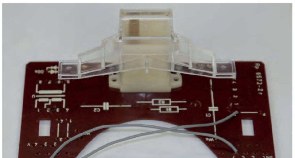
Bottom and top view of the phone board after removing all the components and connector terminals. The two grey wires are soldered onto the clean printed circuit on the bottom side, detecting the hang-up switch
