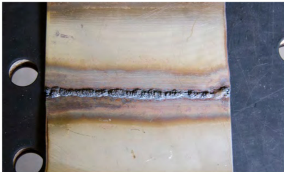
Chromium oxides on underside of weld
