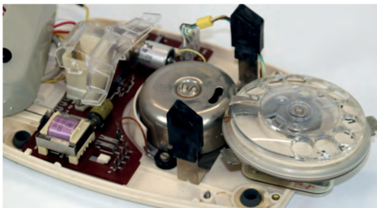
Detail of the inner part of the phone, showing the ringer bell and the solenoid group. Both these parts will be removed as they are no longer needed, creating space to install the Raspberry Pi board
