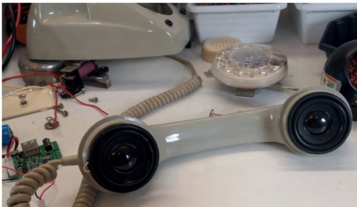
Using the four wires of the original cable in the microphone holder of the phone, I removed the microphone and speaker to solder the cable terminals to the two speakers. These are almost the same diameter as the internal speaker and mic holder. After sandpapering inside, it was possible to insert the speakers and close the holder with the original caps
