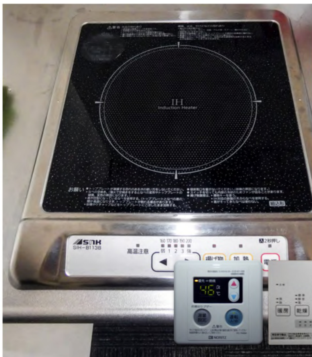
Induction cooktop. The on/off switch is outlined in red. Press and HOLD. Inset are the control panels for the instant hot water (left) and the bathroom heating and ventilation (right)
