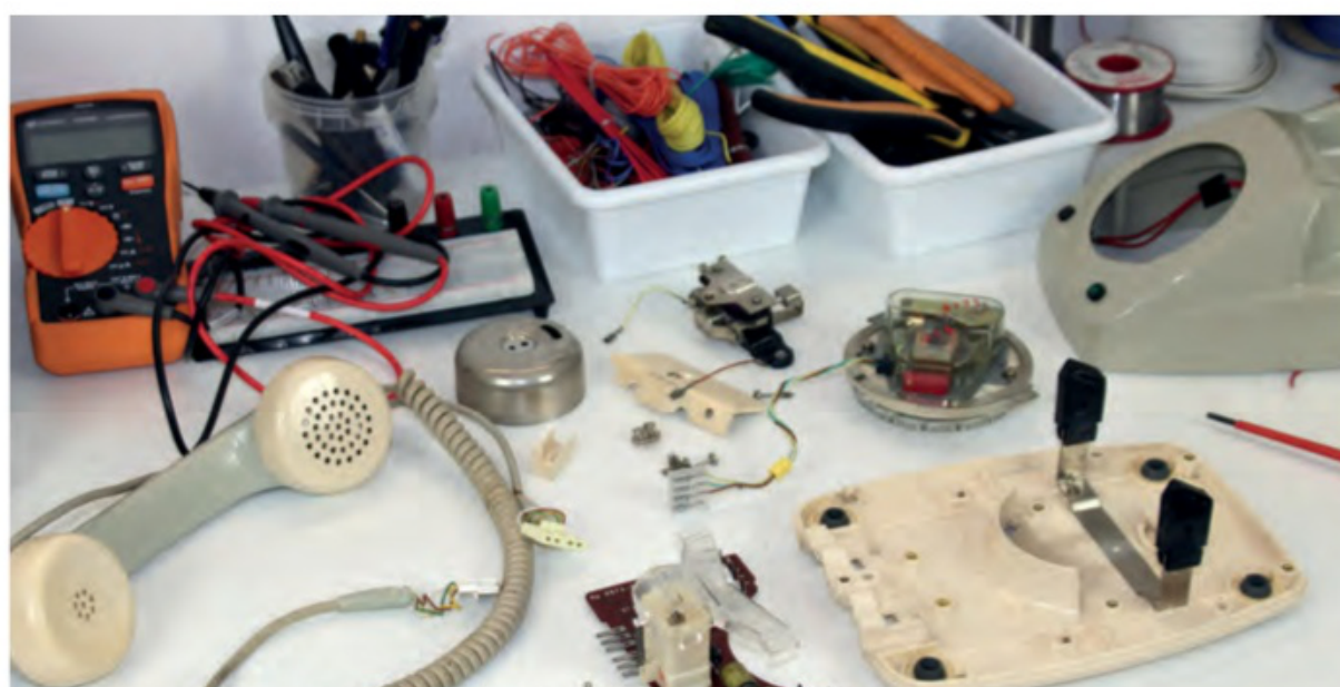
The phone fully disassembled. From left to right: the pick-up (that will host the amplifier speakers), the ringer bell, the phone circuit with the hang-up switch mechanism, the solenoid group and the dialer, the phone plastic base, and the cover at top right
