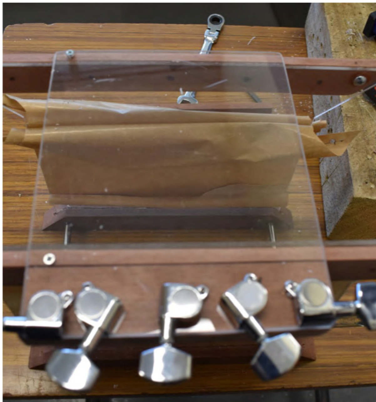
fitting the tensioners
