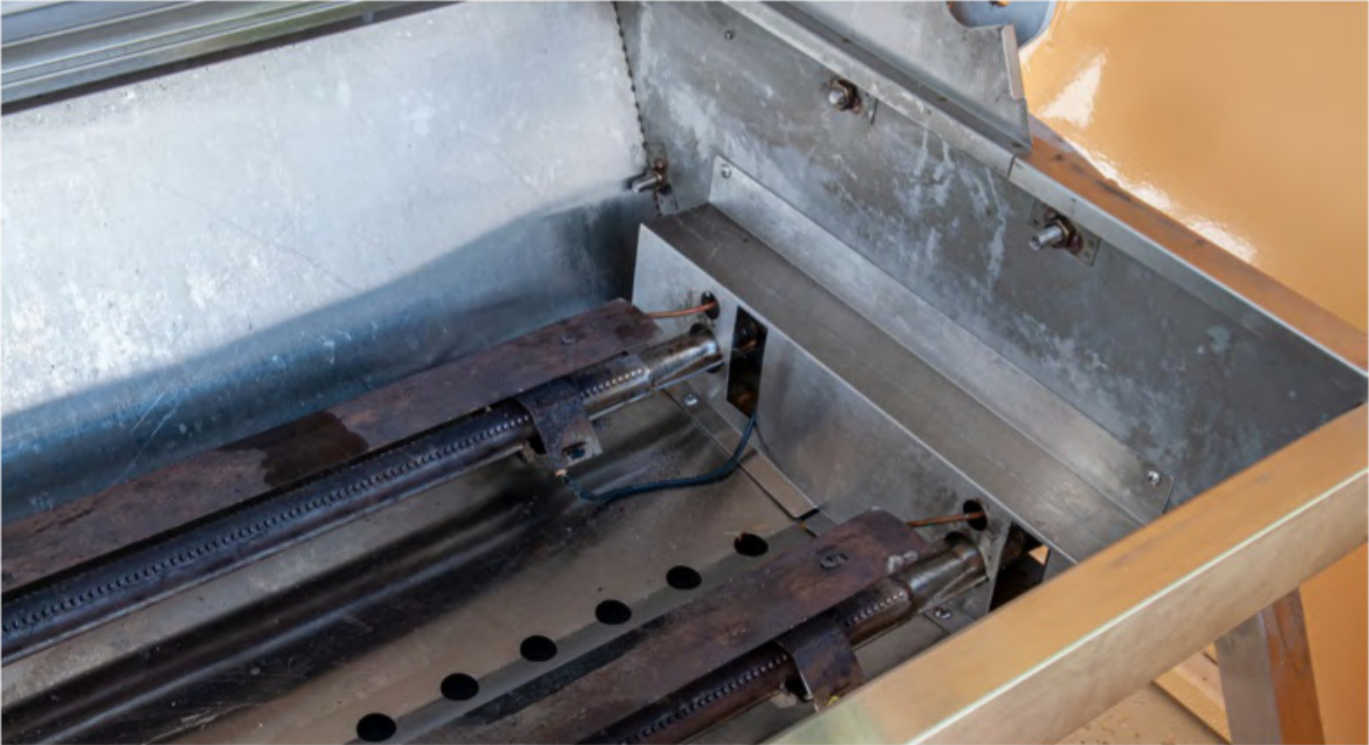
The two ribbon burners
