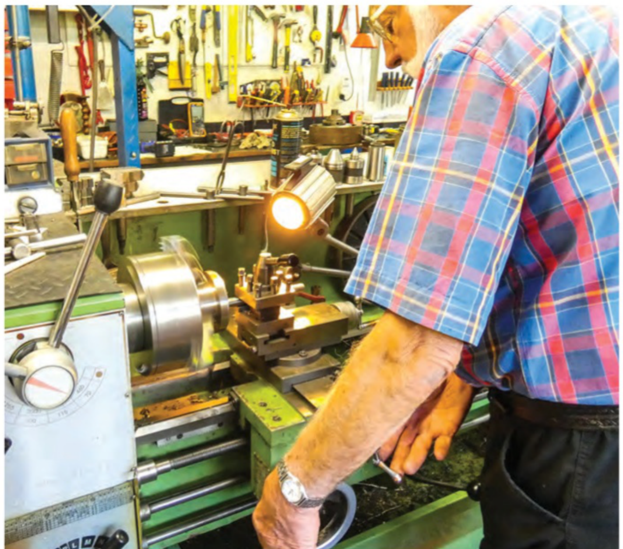
Bob taking a skim off the internal surface of the bearing holder. He relies on micrometers rather than a digital readout to determine if enough metal has been removed
