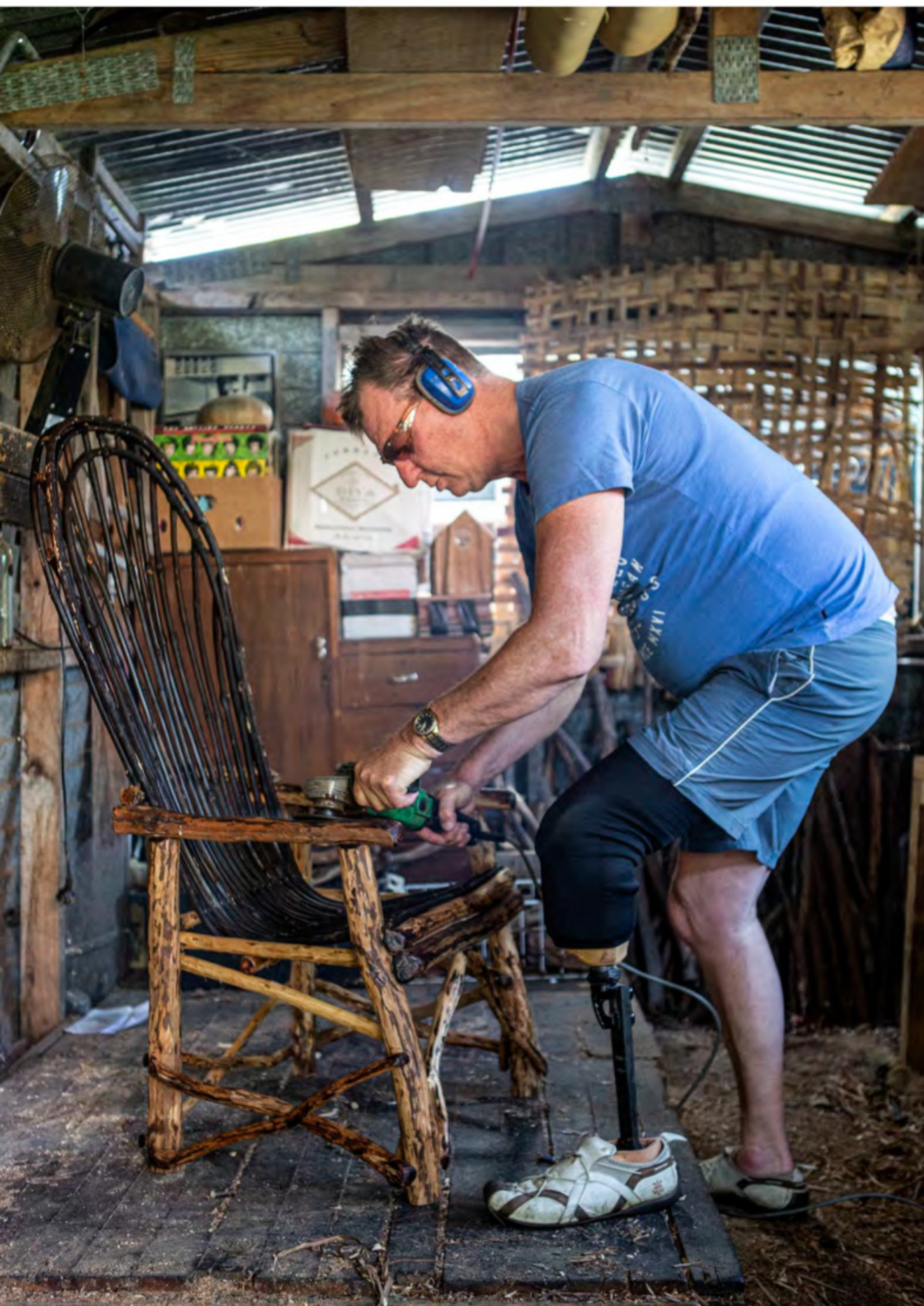
John burnishes the furniture black with an angle grinder to add character and hide the nail heads
