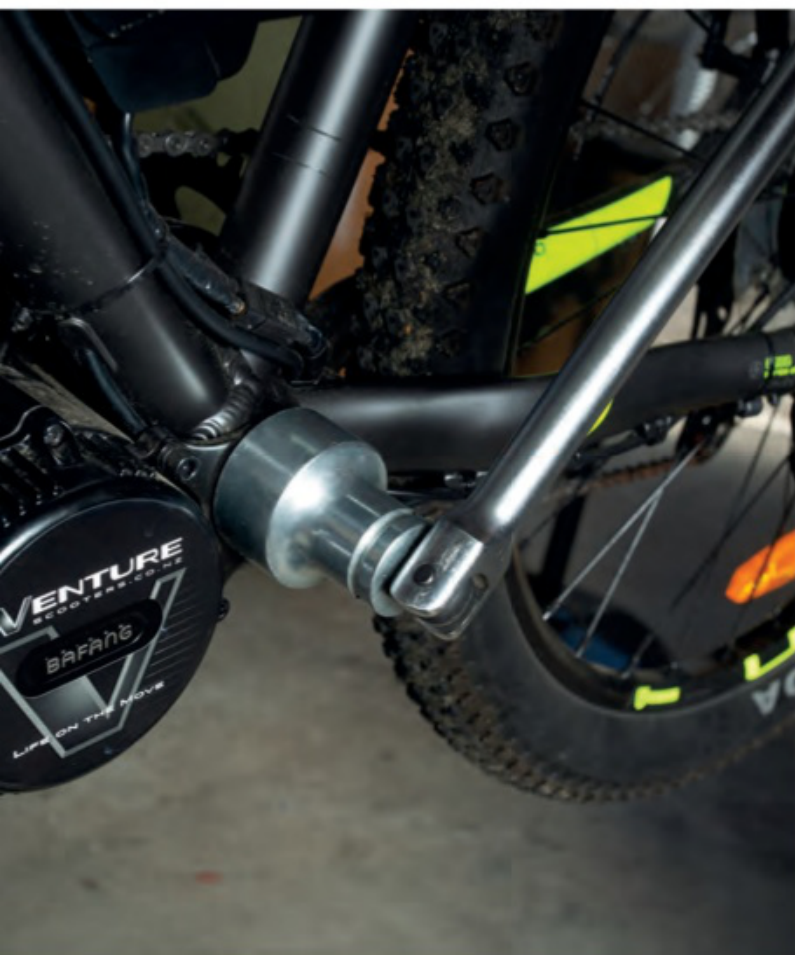
Main mounting nut needs to be tight
