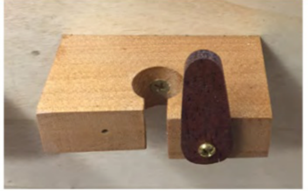
Left: The kwila clips that hold the pipes in place Below: One of the cloth flaps that acts as a valve Bottom: Pipe installation
