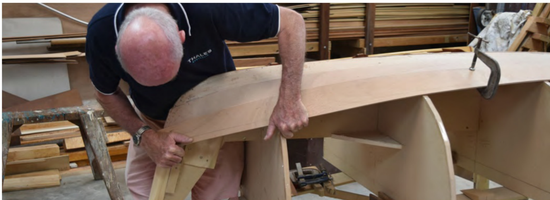
Above: Lapstrake work by Allan Hooper, overlapping planks carefully
