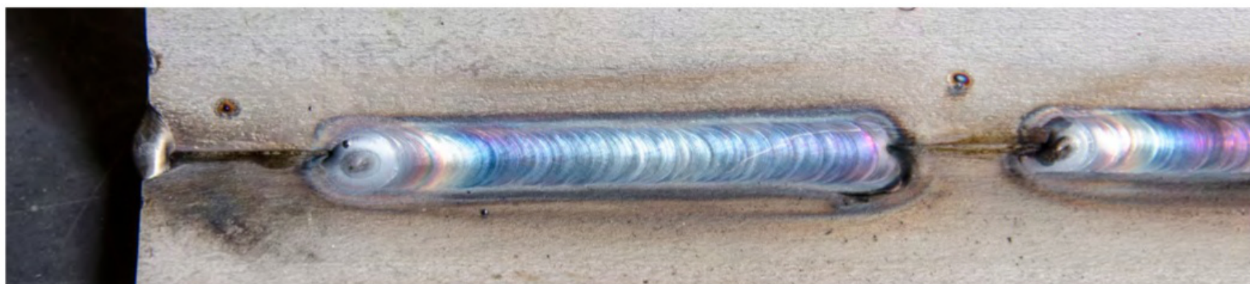
TIG weld in stainless using argon
