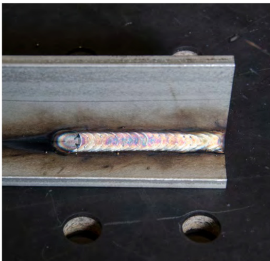
MIG weld with Stainshield Universal
