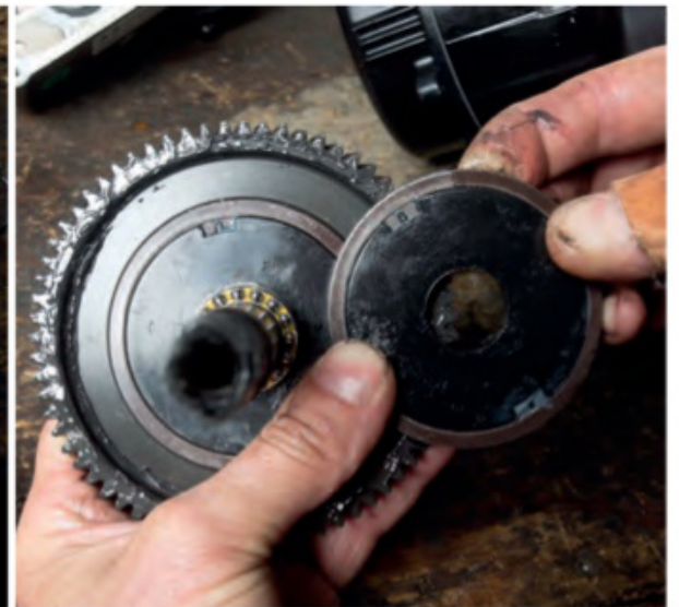
Example of cracked cadence magnet disk
