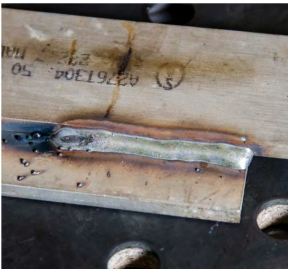
Stainless steel MIG weld using argon
