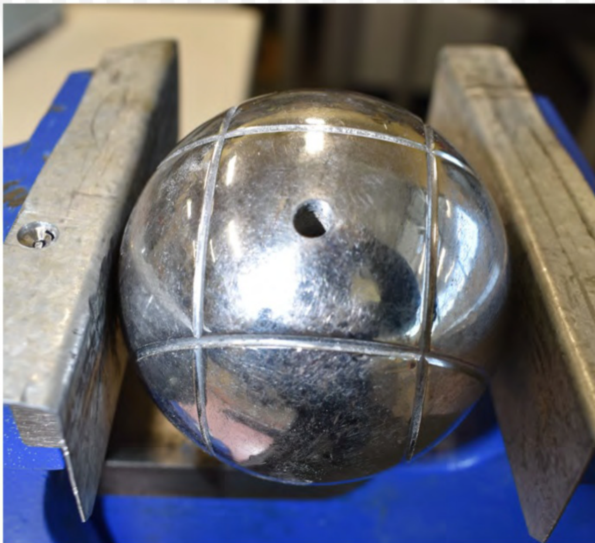
Drilling and tapping the boule ball
