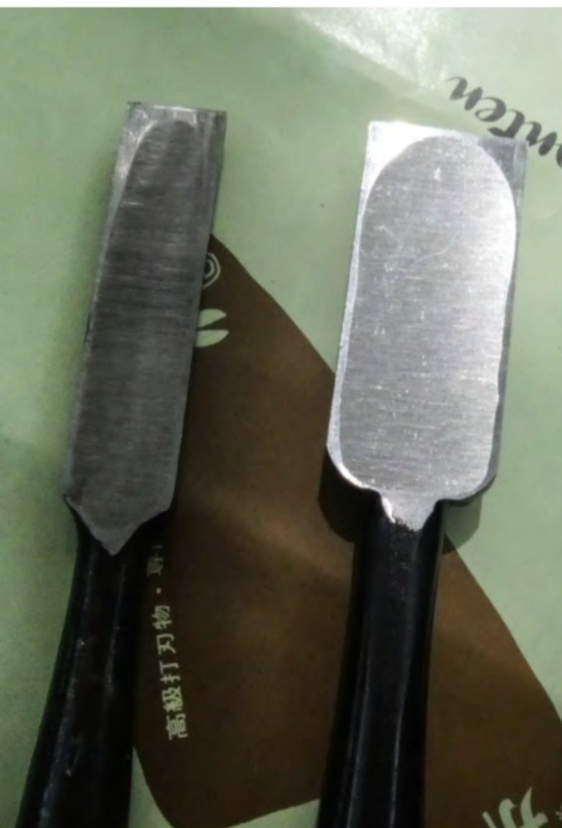
The relief ground in the back of the chisel blades makes for faster sharpening
