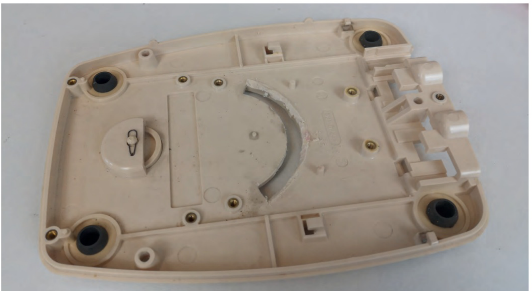
The base of the phone after the removal of the plastic support; the bottom rounded hole will be useful for cooling the Raspberry Pi after inserting it in the space behind the rotary dialler
