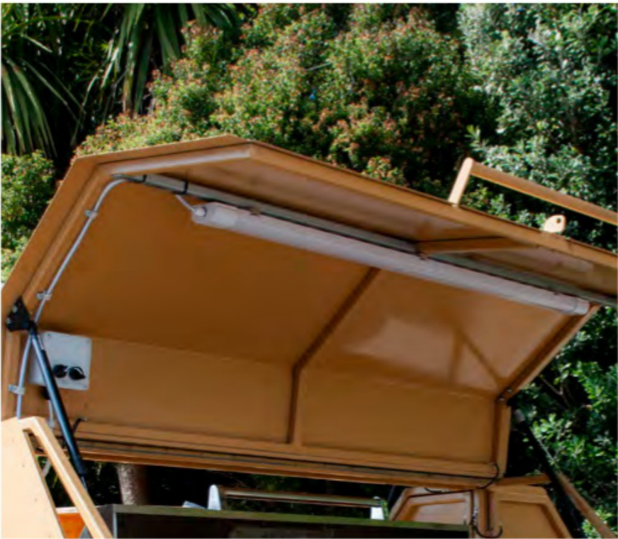
The LED strip lighting in the gull wing of the trailer
