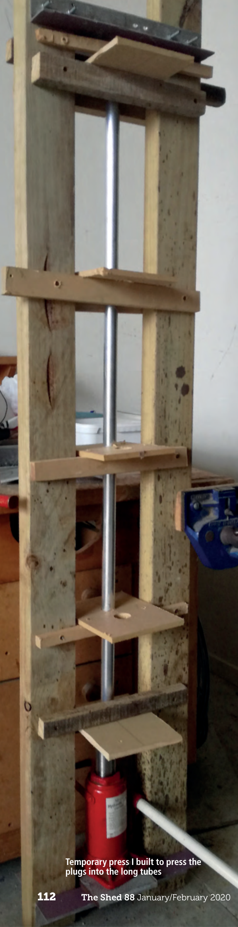
First attempt at pressing end plug — one buckled tube
