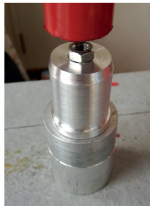
Pressing nut in end plug
