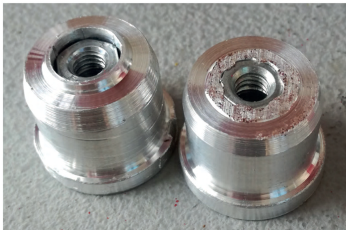
End plugs with nuts pressed in placed
