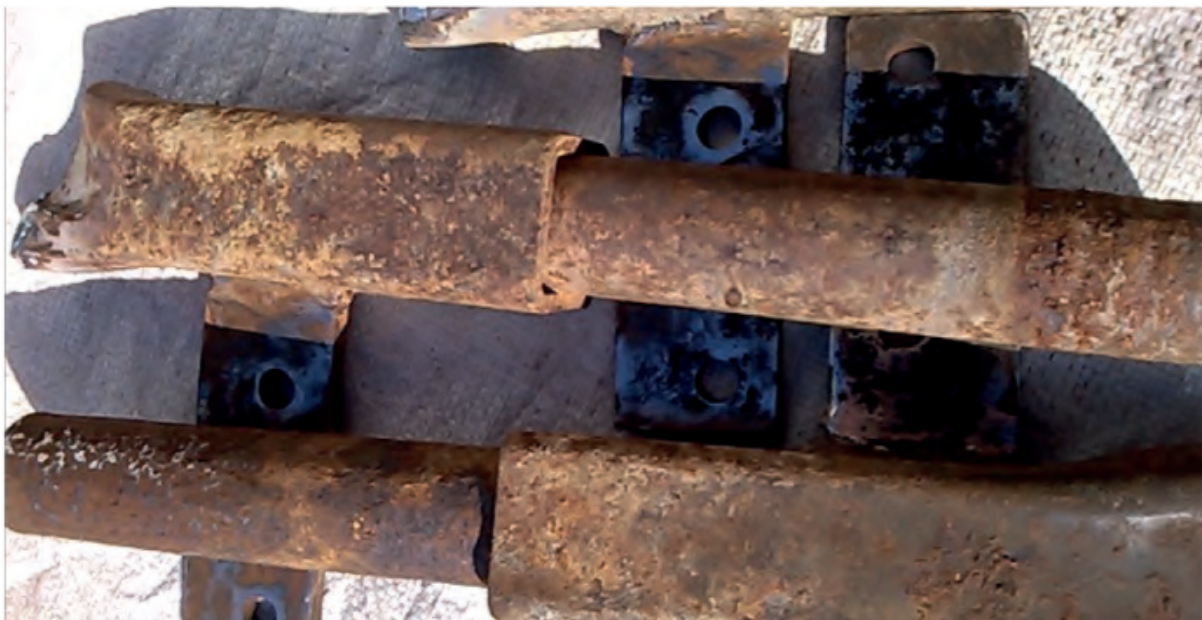
The Connor Shea direct-drill coulters before molasses treatment ...
