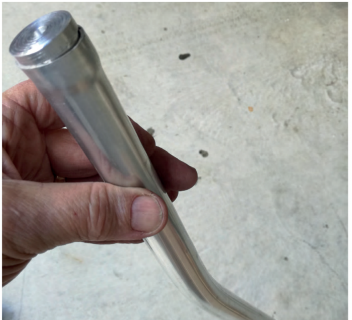
First attempt at pressing end plug — one buckled tube
