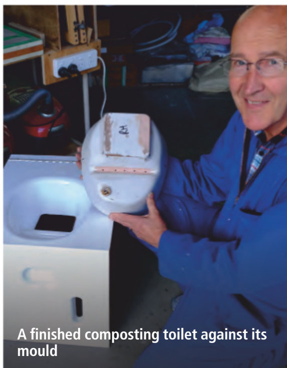
Des showing the male mould of his composting toilet next to the final product
