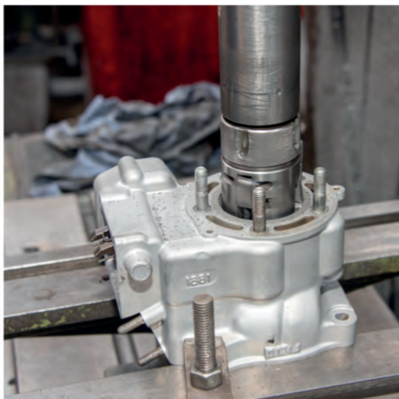
Far left: Mike Hudson and his dog Diesel Left: Re-boring a cylinder Below: A collection of old valves
