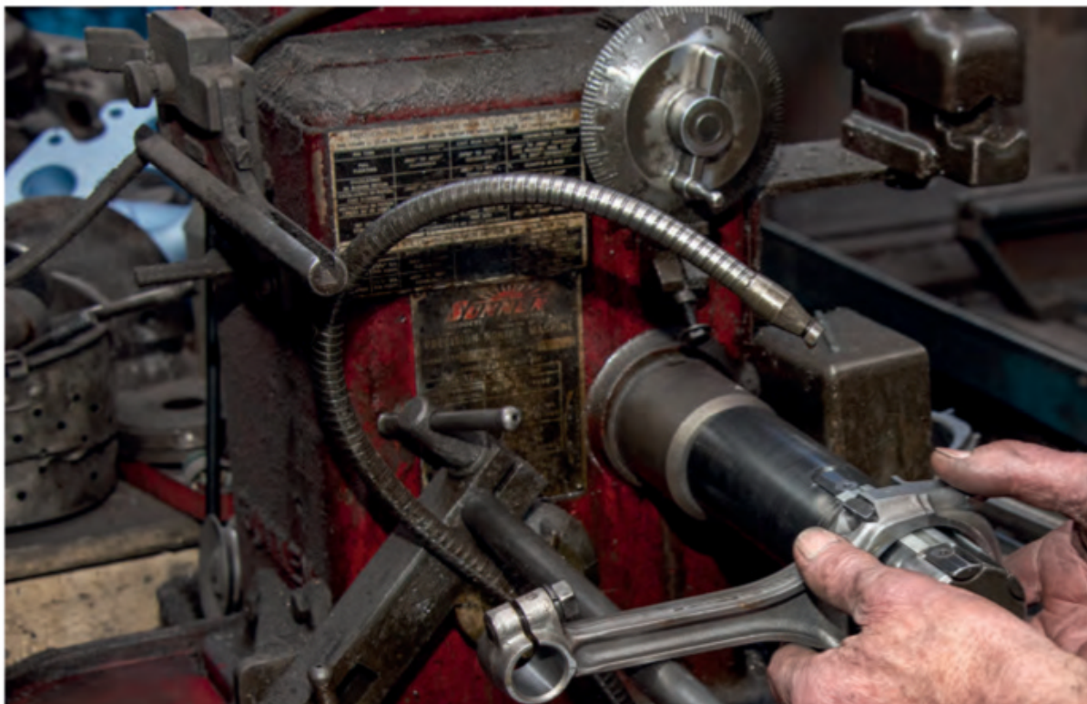
Above: Honing a con rod big end; below: Grinding journals on a crankshaft
