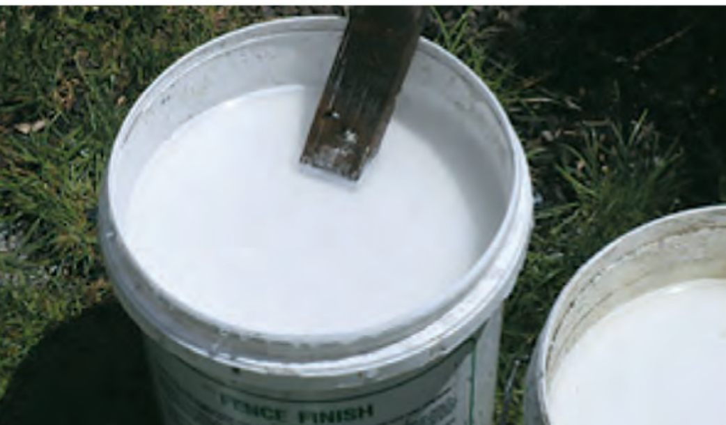
Lime soaked in water — weeks rather than days to prepare
