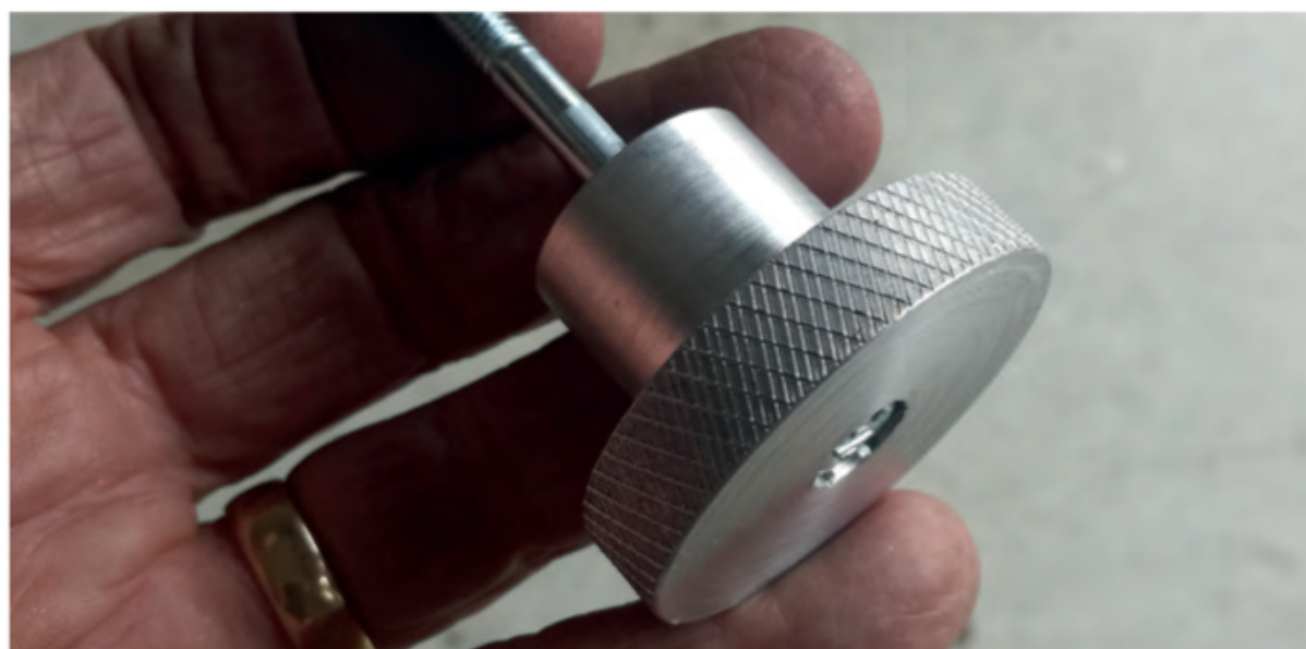
Below: Knurling a nut in the lathe. Below right: Finished knurled nut provides good grip
