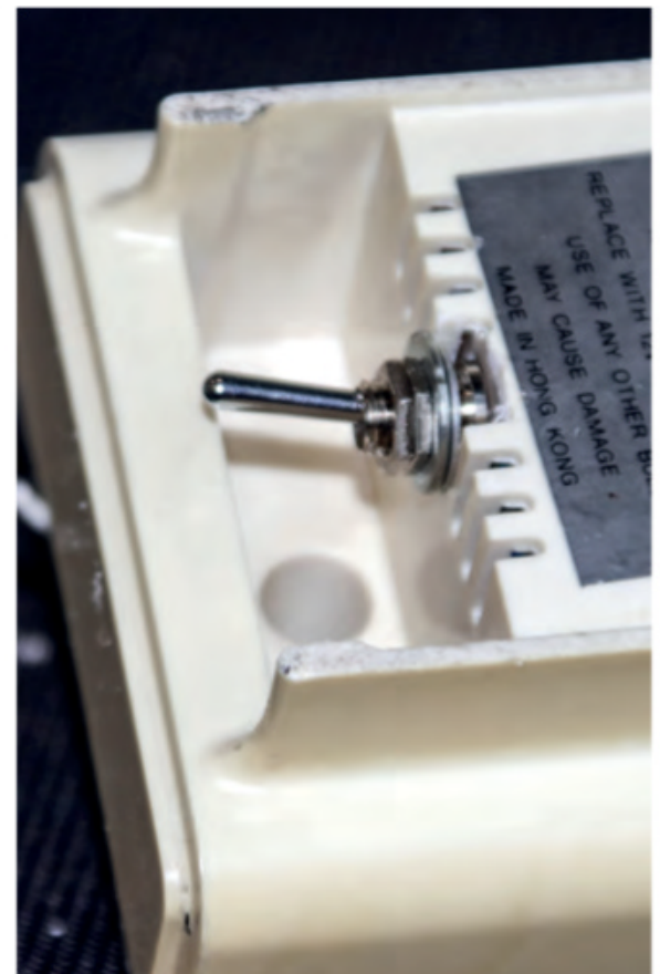
Above: After reassembling the lamp head, the slider, electret microphone, and switch were fixed inside the base box
