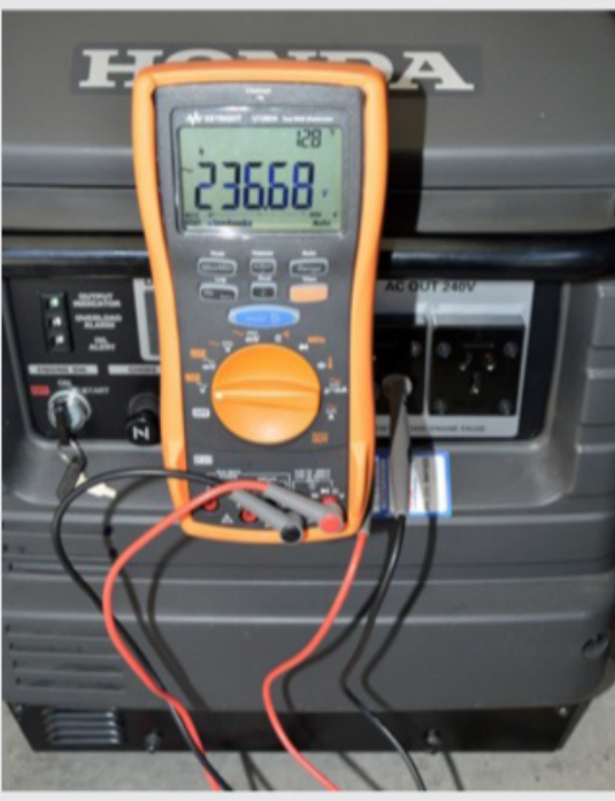
Below: Voltage (left and right) and frequency (middle) for the EU30is showing difference between loaded and unloaded voltage readings
