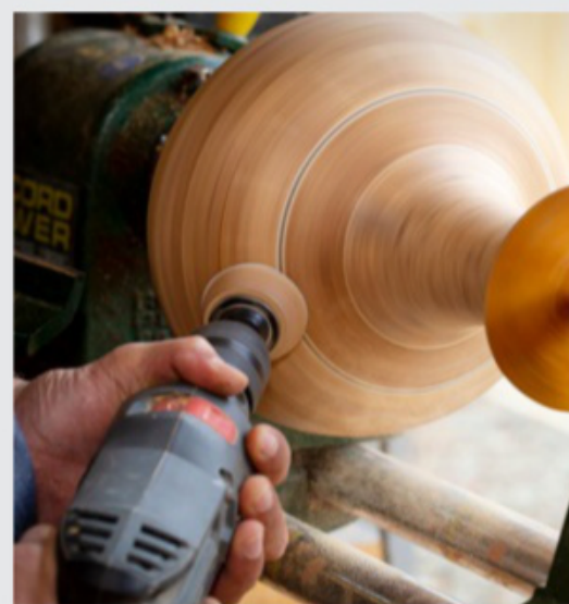
Sanding the hollow-form top using a drill with Velcro-backed sanding discs
