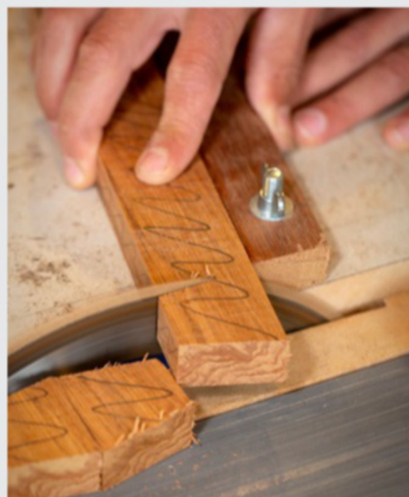
Below: Alby cuts the segments on a wedgie sled, which is set to the cut angle. There is no tolerance for inaccuracies, which would create gaps
