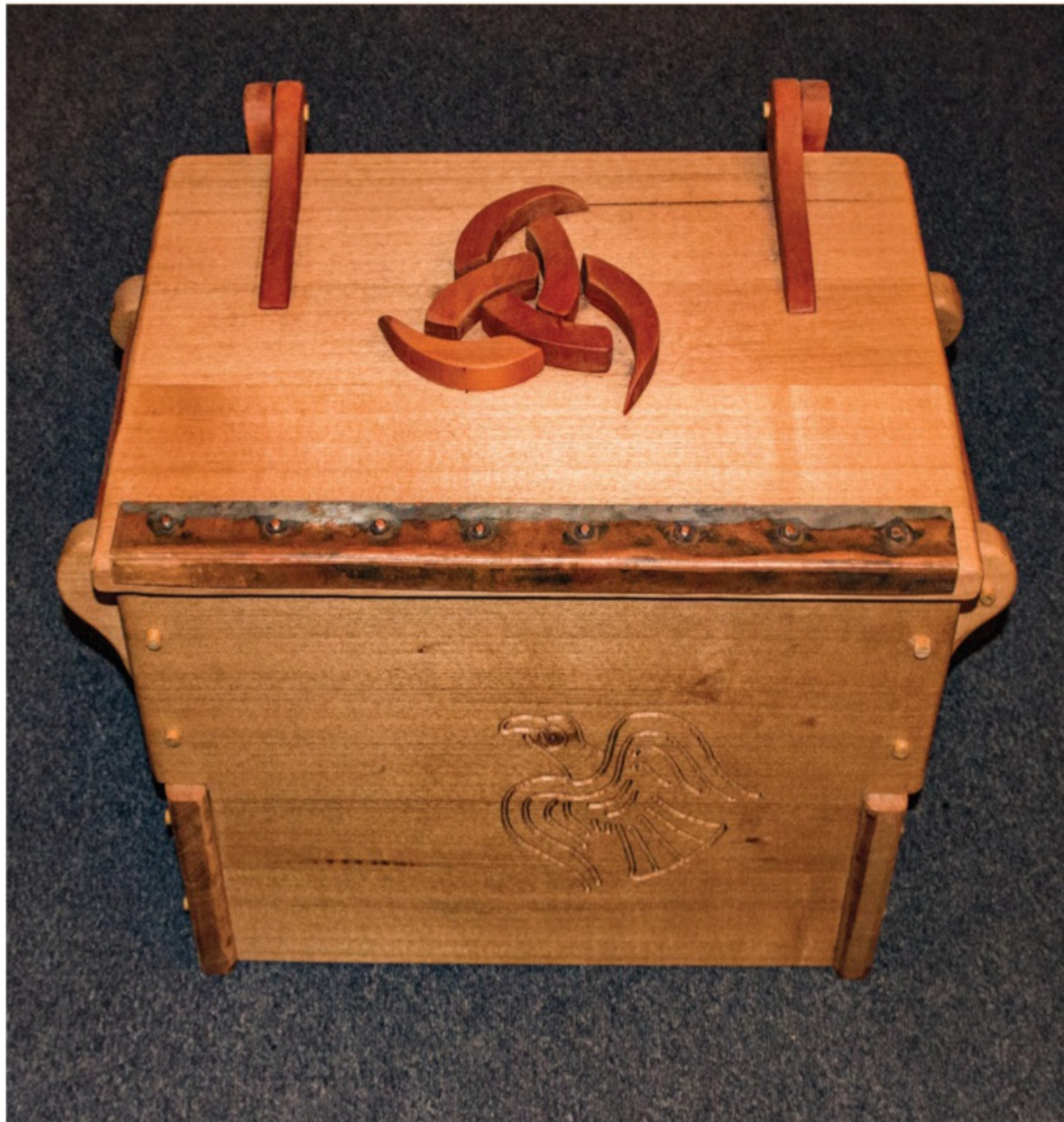
A Viking-style chest showing the dowels that hide the screws, the simple plank construction, and timber hinges in keeping with the era. Viking-style drawings have been routed in the sides and another glued to the lid from myrtle offcuts"
