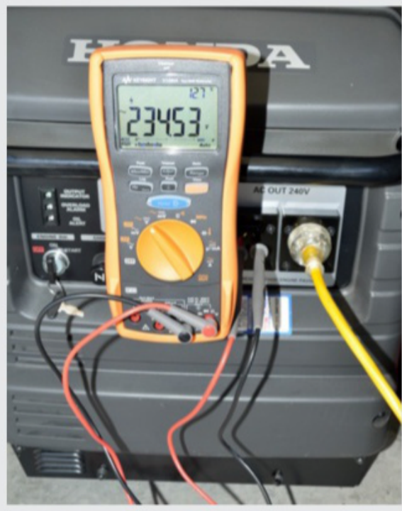
Below: Voltage (left and right) and frequency (middle) for the EU30is showing difference between loaded and unloaded voltage readings
