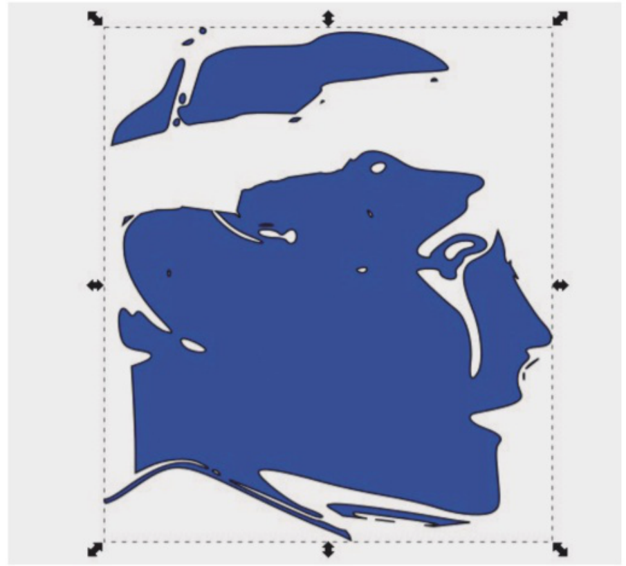
Above: The line-art conversion has been processed with Inkscape to extract the image contour. To do this (colours are only helpers for drawing), instead of exporting a bitmap the image is saved in DXF format, the portable 2D vectorial file that can be read by T2Laser and most of engraving programmes
