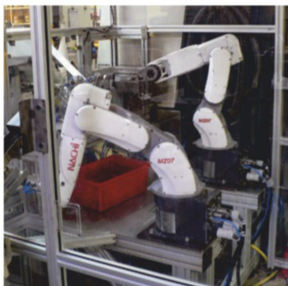
Robots placing the finished twist drills into plastic sleeves
