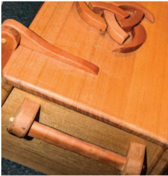
A Viking-style chest showing the dowels that hide the screws, the simple plank construction, and timber hinges in keeping with the era. Viking-style drawings have been routed in the sides and another glued to the lid from myrtle offcuts"
