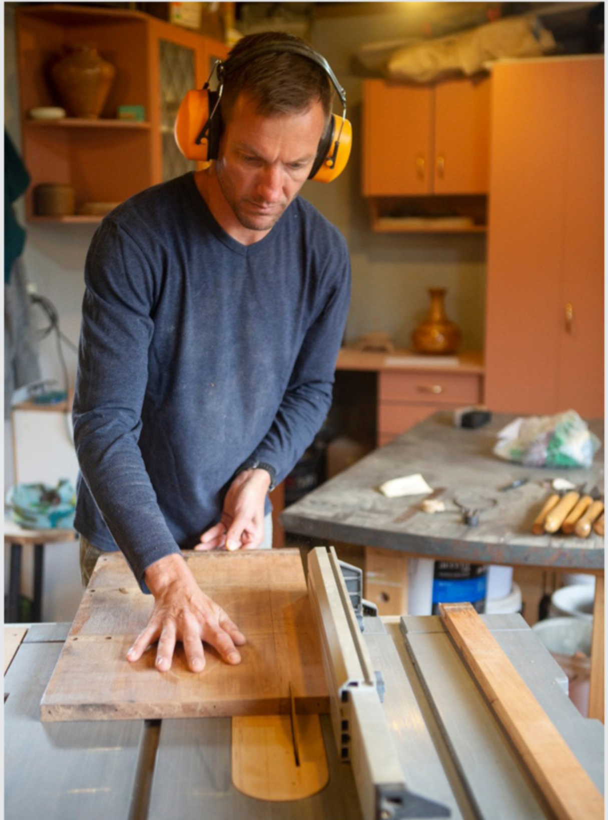
Above: Alby recycles timber, in particular New Zealand native timbers. He removes old nails and screws and rips the wood into rectangular batons about 20mm thick
