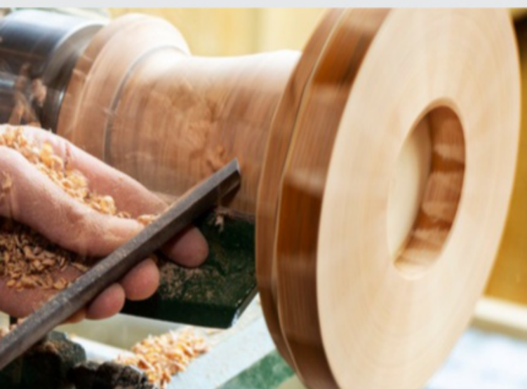
Turning the top half, initially using a gouge to cut off extra wood
