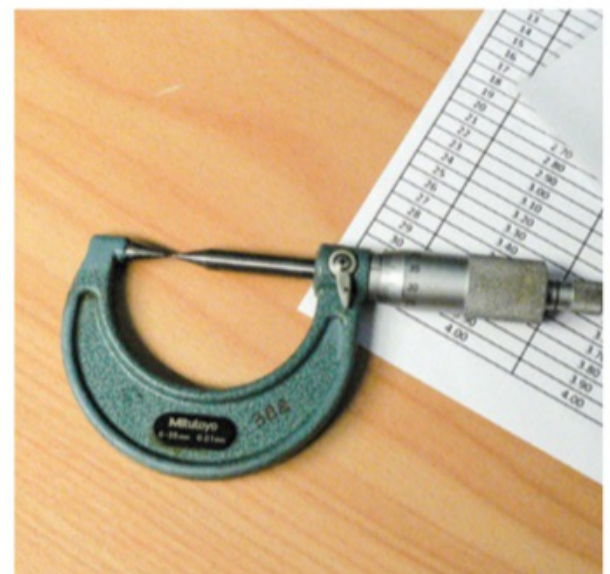
A Mitutoyo point-tip micrometer for measuring the core of a twist drill
