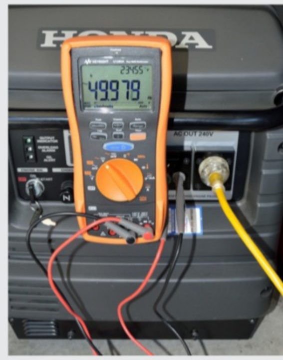
Below: Voltage (left and right) and frequency (middle) for the EU30is showing difference between loaded and unloaded voltage readings
