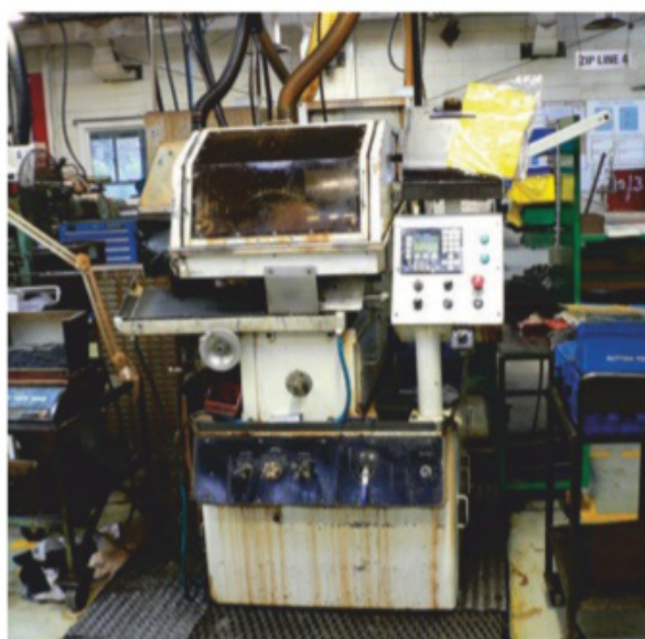
A drill-making machine in full cry. The observation window is almost completely obscured by grinding oil. The oil is delivered by the tubes above the machines
