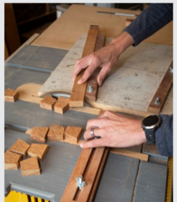
Below: Alby cuts the segments on a wedgie sled, which is set to the cut angle. There is no tolerance for inaccuracies, which would create gaps
