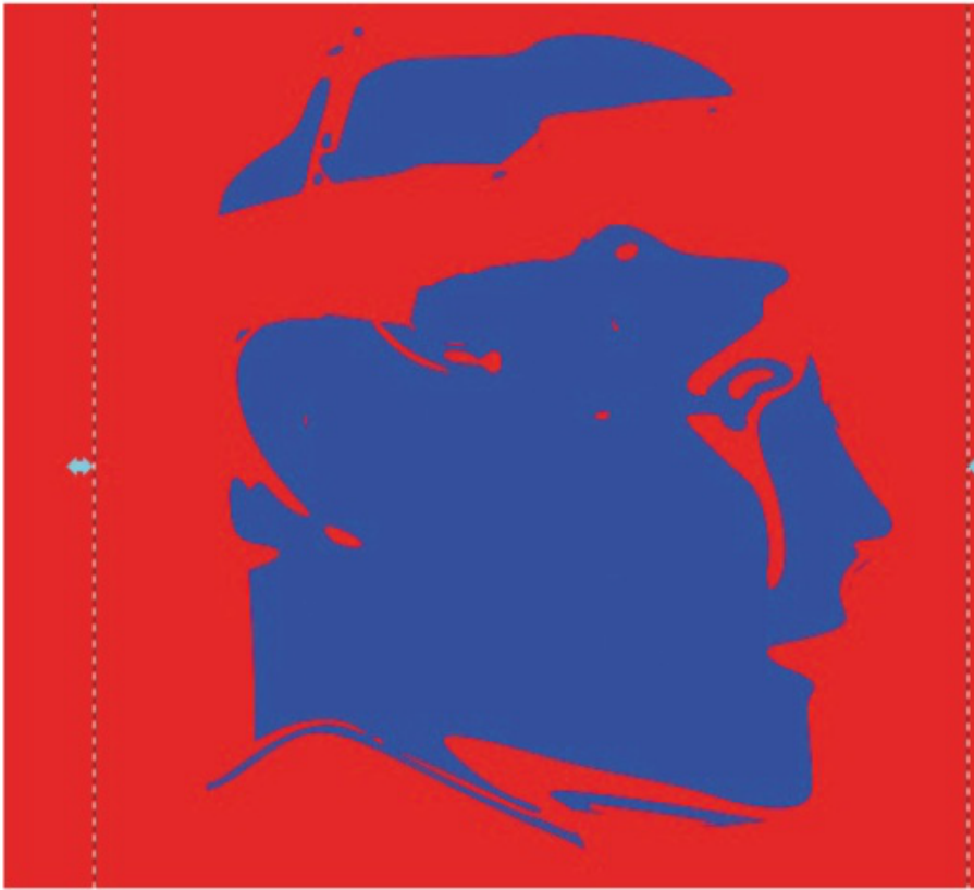
Above: The line-art conversion has been processed with Inkscape to extract the image contour. To do this (colours are only helpers for drawing), instead of exporting a bitmap the image is saved in DXF format, the portable 2D vectorial file that can be read by T2Laser and most of engraving programmes
