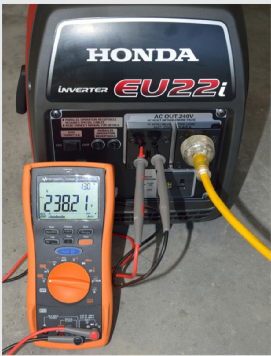
Above: Voltage (left) and frequency (right) of the EU22i
