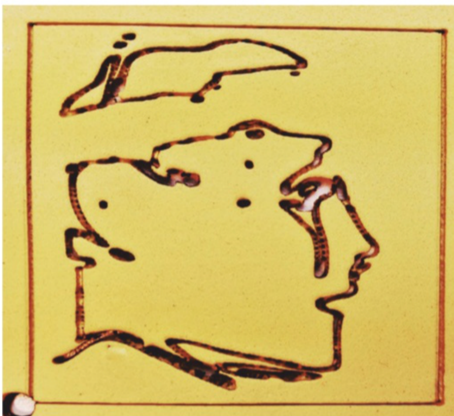
Above and below: An example of how very different effects can be created from the same vectorial image, depending on the laser speed. Engraving materials like plastic surfaces, cardboard, and leather can be an efficient method to personalize handcrafted objects with your own artwork and logos
