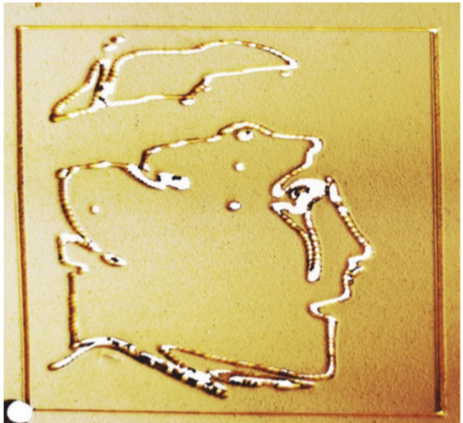
Above and below: An example of how very different effects can be created from the same vectorial image, depending on the laser speed. Engraving materials like plastic surfaces, cardboard, and leather can be an efficient method to personalize handcrafted objects with your own artwork and logos
