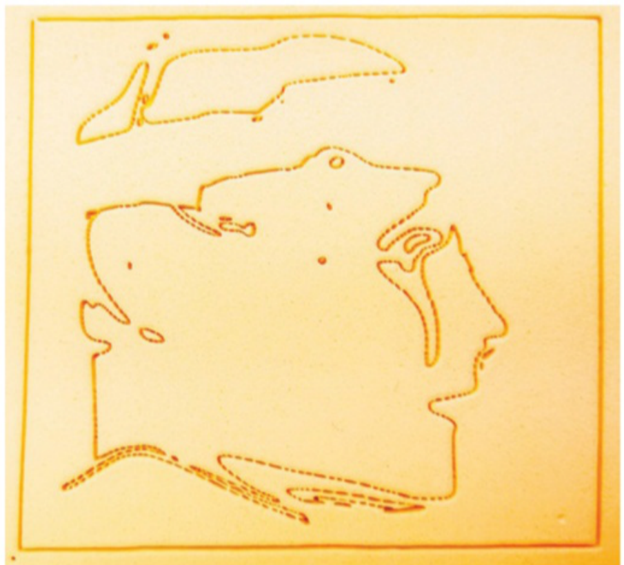
Above and below: An example of how very different effects can be created from the same vectorial image, depending on the laser speed. Engraving materials like plastic surfaces, cardboard, and leather can be an efficient method to personalize handcrafted objects with your own artwork and logos
