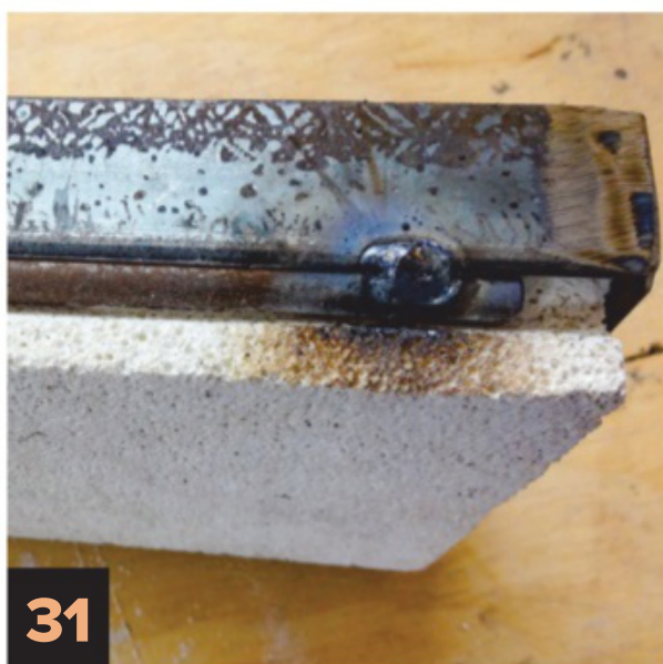
29 29-31: A 6mm round bar is fitted into the groove and tack welded in place to hold the brick into the door frame
