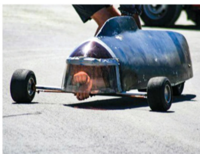
Right: Final iteration — there's a youngster lying prone behind those tiller-clutching knuckles. Fairing is a catamaran hull, inverted and travelling stern-first, aerodynamics and hydrodynamics being somewhat similar ...
