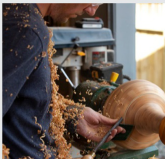
Turning the top half using a scraper to refine the surface
