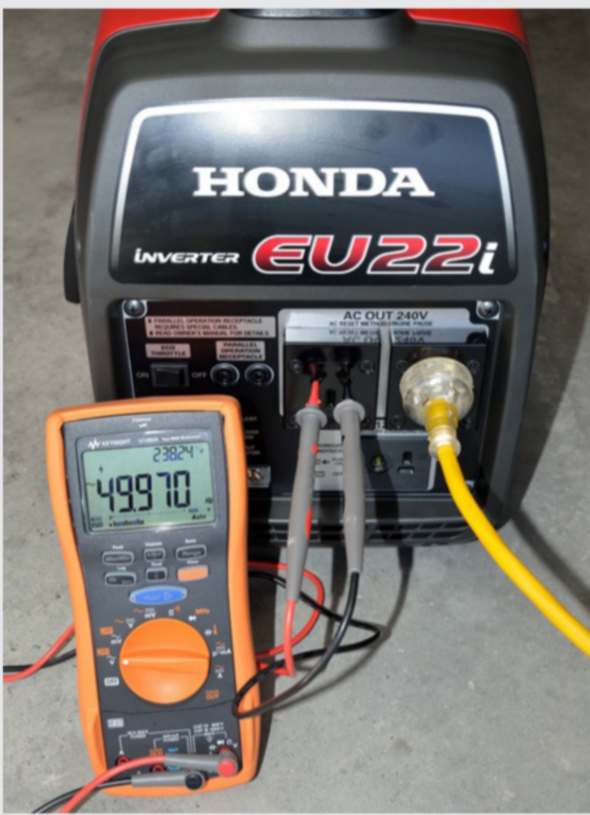
Above: Voltage (left) and frequency (right) of the EU22i
