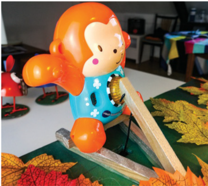
Left: The internal servo presses the monkey's belly button with a mechanical action
