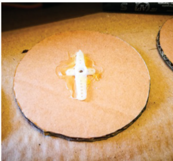
Above: Three steps in the creation of the rotating platforms for the birds, with the servo lever glued with its axis centred to the bottom of the platform
