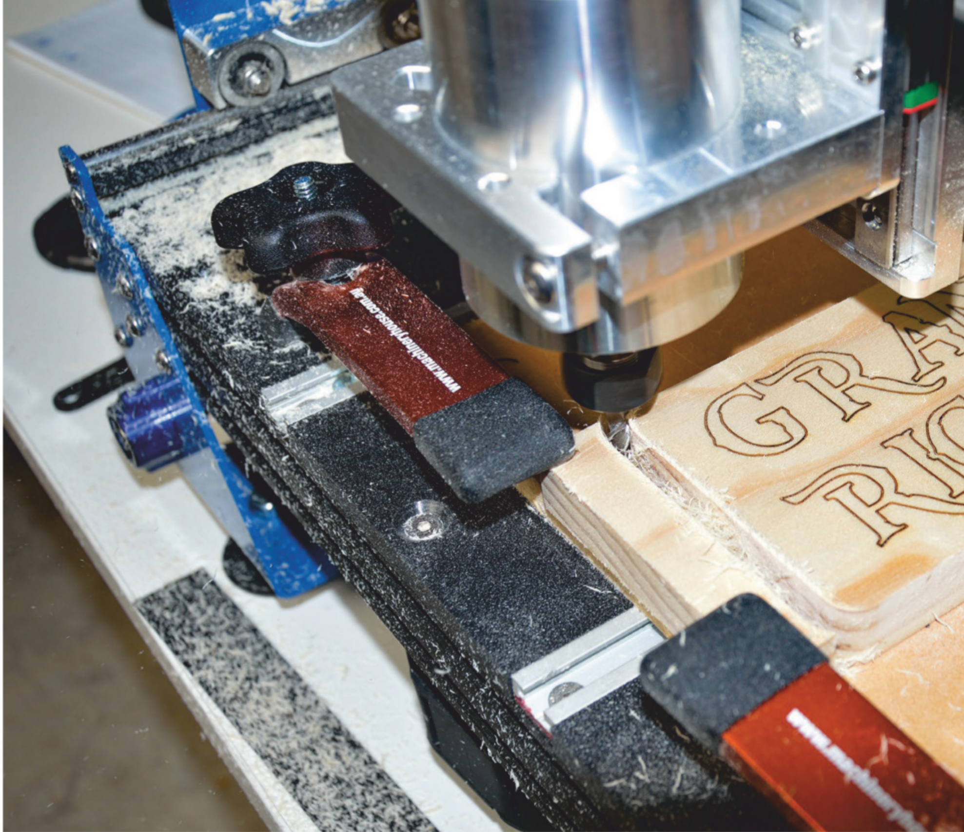
Above: Routing contour — finish is such that there is no sanding required apart from to the edge
