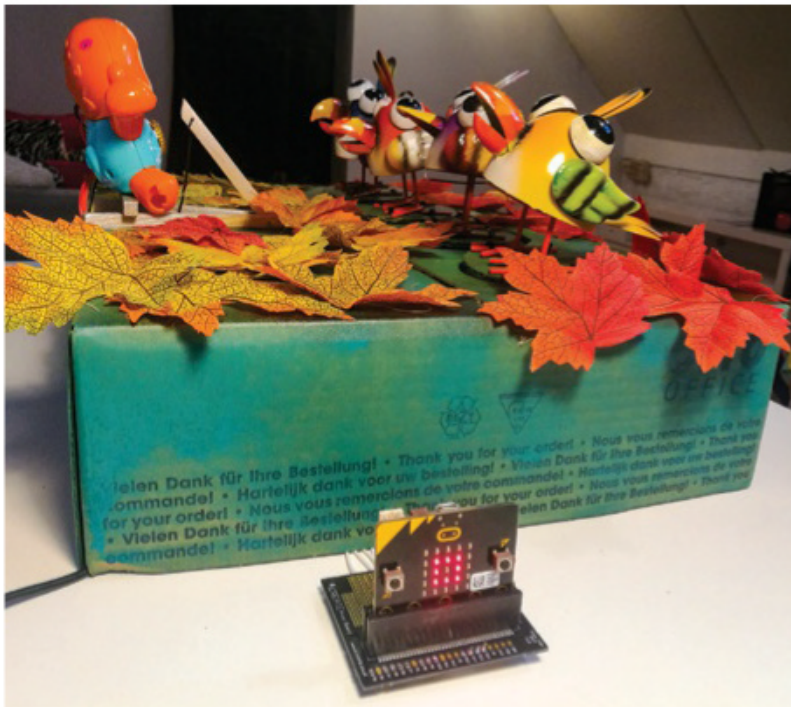
Left: While the Arduino Mega controlling the servos fits inside the box, the control wires are connected to the Micro Bit board, exposed so that the display feedback can be seen and it can be reset and paired with the smartphone via the Bluetooth connection
