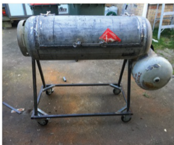
Basically the whole build was done with an angle grinder and a welder. The only real costs were for the box-section steel and the castor wheels
