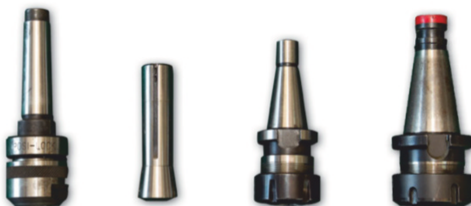
The most common spindle shanks that you will find on home workshop machines (left to right): Posilock tool holder three Morse taper shank, R8 shank tool holder, ER tool holder 30 taper shank, and 40 taper shank
