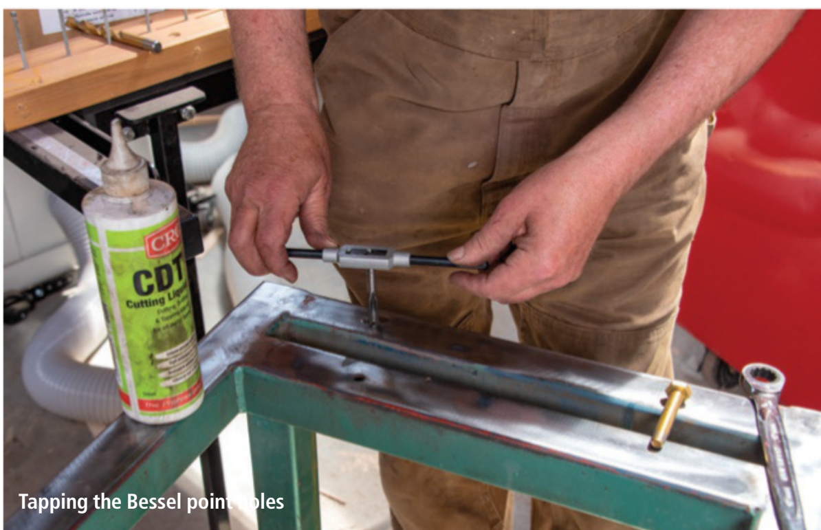
Boring the holes for the Bessel points that will support the block
