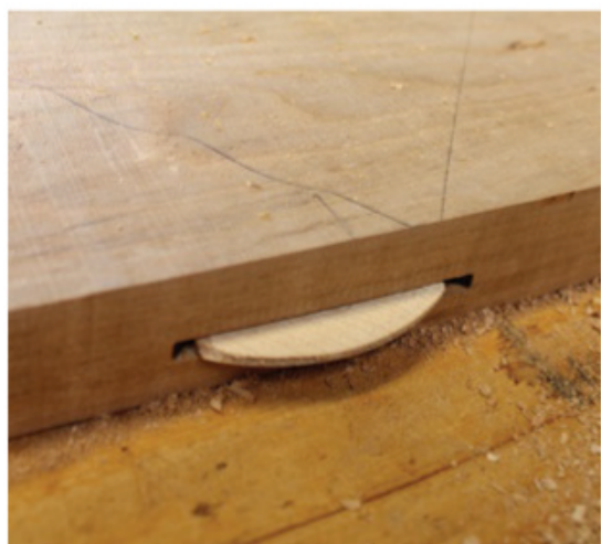
Above: Machined timber ready for the biscuit slots Left: A biscuit in place, minus the glue
