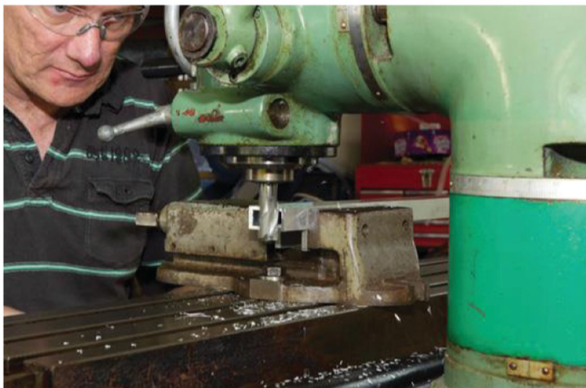
Left: End milling of a box-section workpiece
