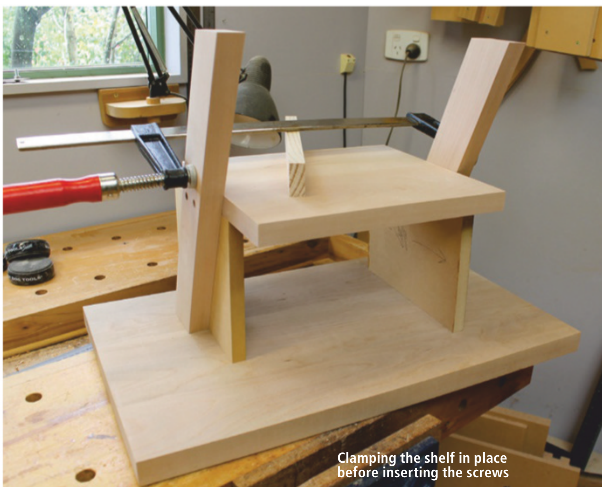
Clamping the uprights in place before screwing them in place from underneath
