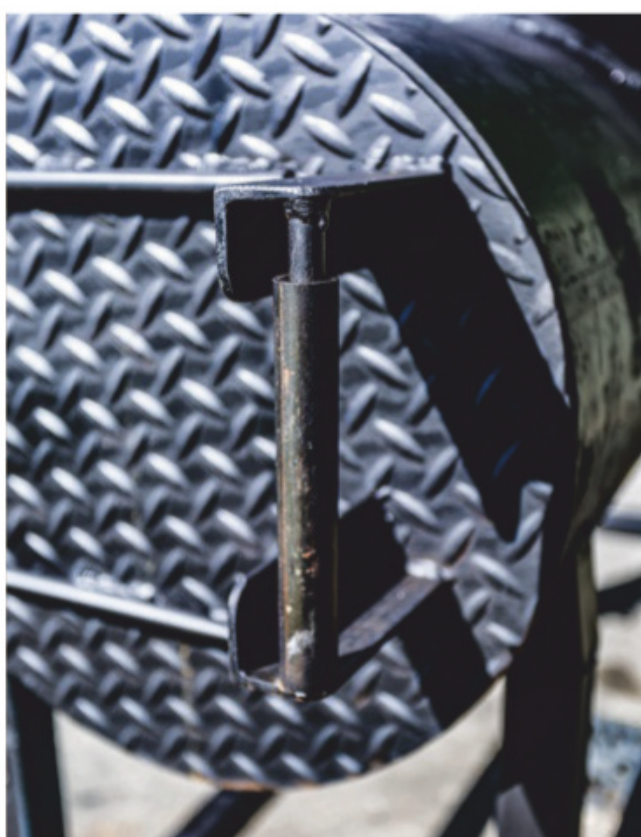
Roman used a pressurized water tank for his smoker's main body and used Feldon's BBQ Pit/Smoker Build Calculator for critical dimension advice
