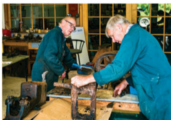
Below: Engine volunteers Graeme Murray and Ralph Paulger cleaning the dismantled Witte swing-arm log saw
