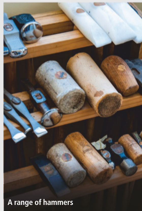
Different shaped tools for planishing and forming, with those for anticlastic raising on the middle shelf
