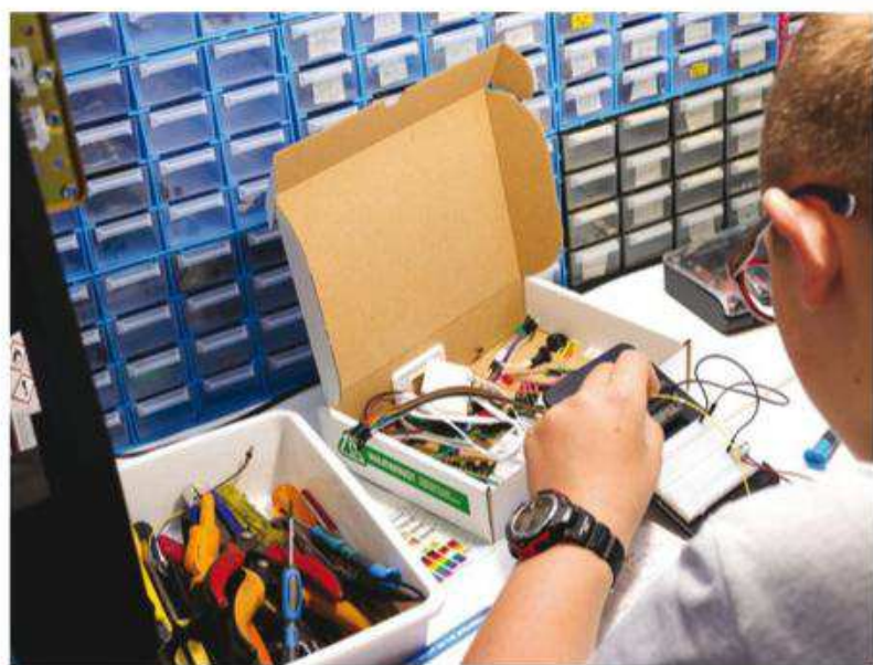
After the moving parts were assembled, using the breadboard of the micro:bit connector base, the simple circuit of the generator was wired
