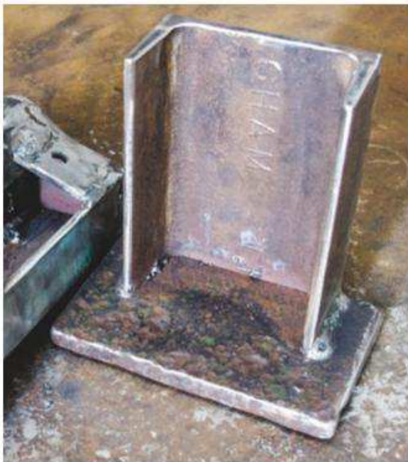
The upright channel welded to baseplate
