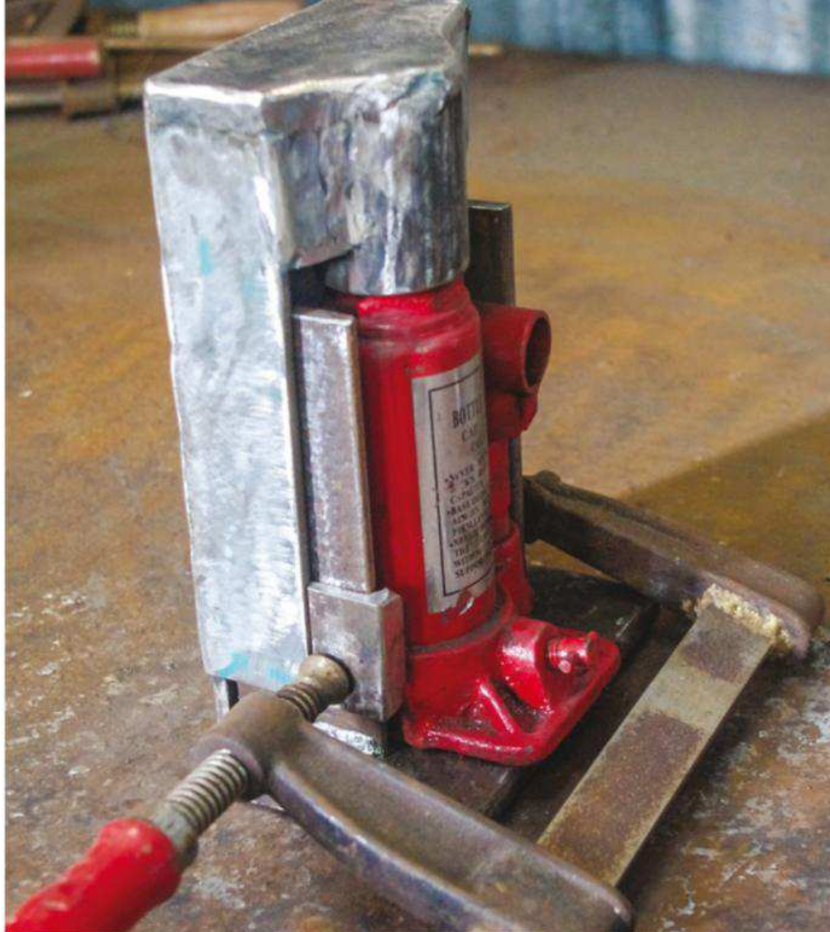
Left: The angle on rear of the carriage Below: The tongue welded to the front of the carriage Bottom: Once the baseplate extensions are welded on, the jack is finished
