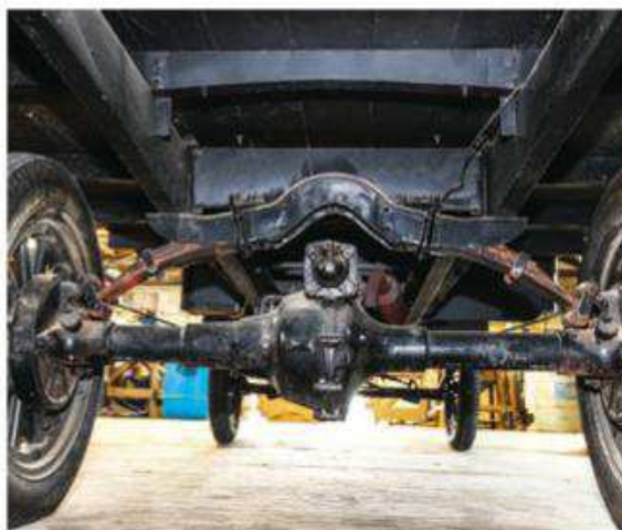
Above: The completed bus — seen as one to add to the series rather than a replica Below: The project took Max Laver and Mark Carter eight months to complete. Note the rear traverse springs — they make the ride a bouncy one
