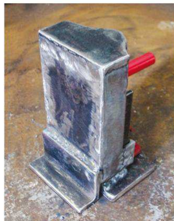
Left: The angle on rear of the carriage Below: The tongue welded to the front of the carriage Bottom: Once the baseplate extensions are welded on, the jack is finished
