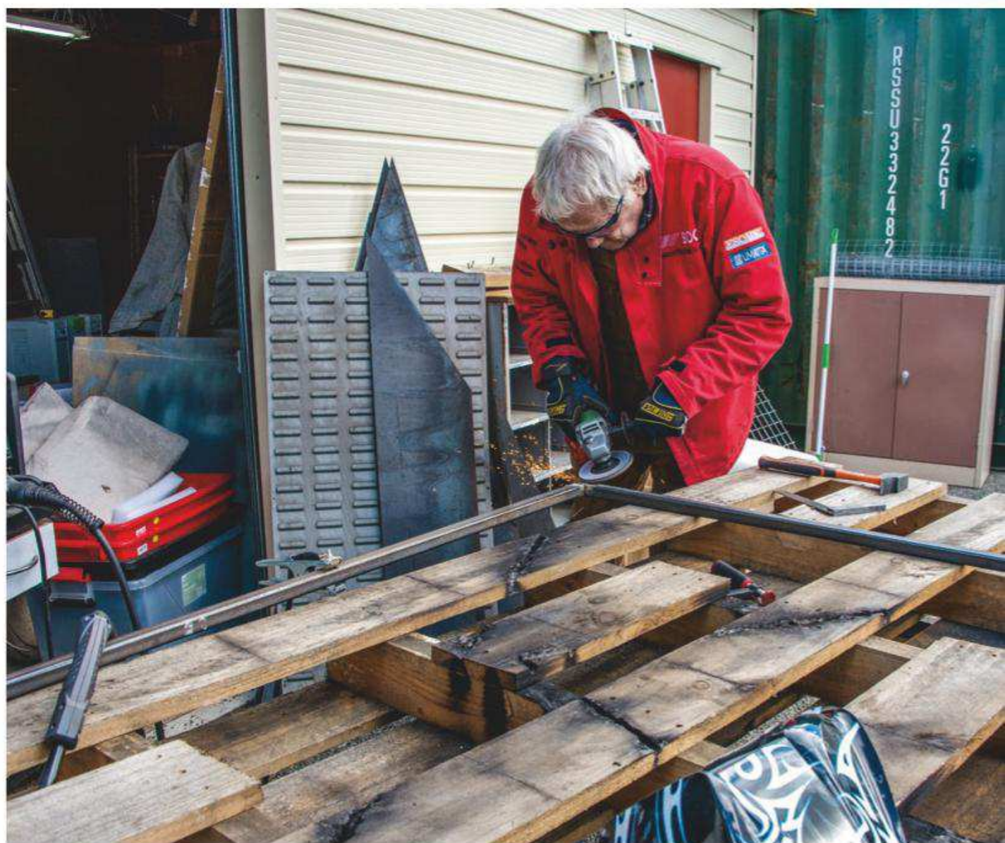
Above: Cleaning off the welds
