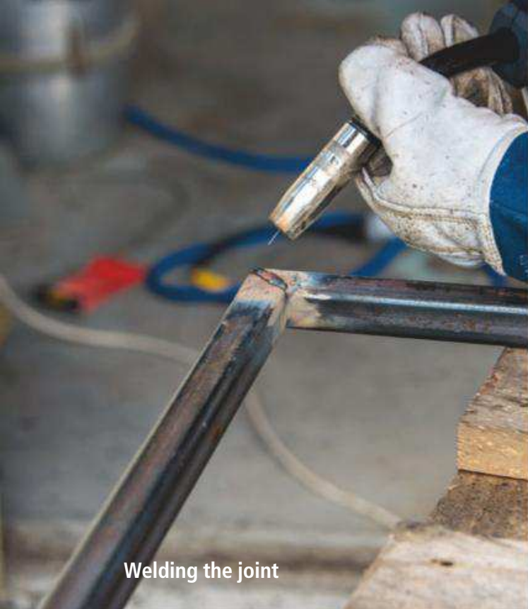
Gasless wire weld. Apart from the shielding material the weld is quite clean
