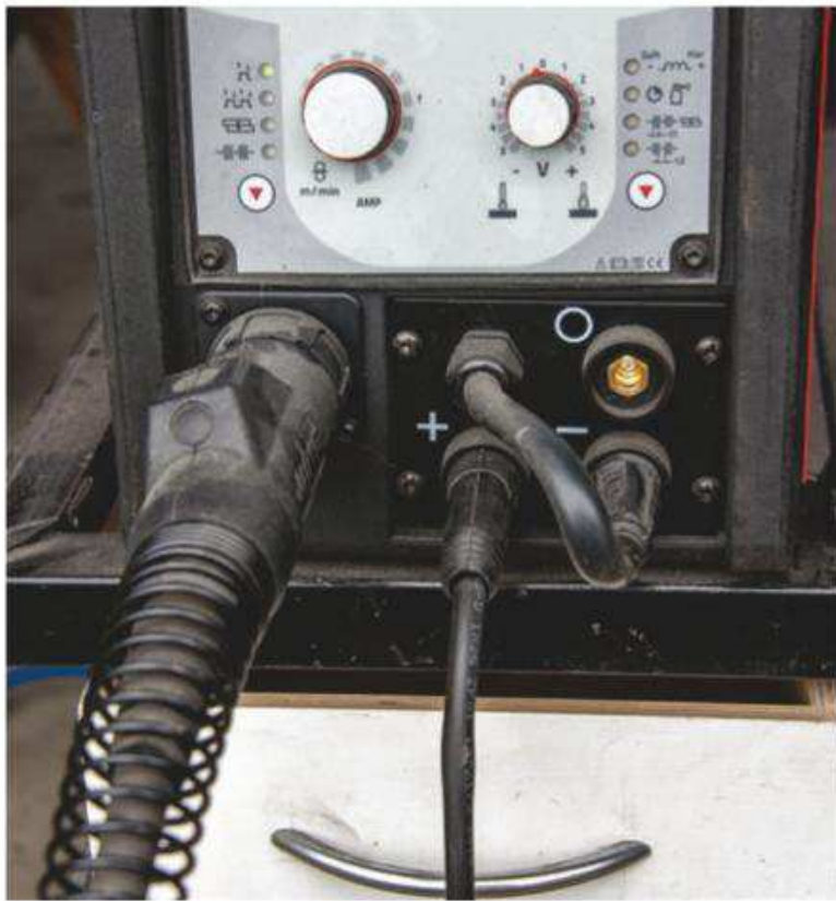
Above: Changing the polarity. The earth lead is switched to positive and the electrode to negative
