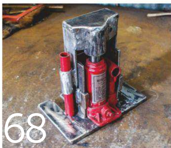
Make a toe jack Gotta do some heavy lifting and not a lot of leverage to work with? Here's a solution
