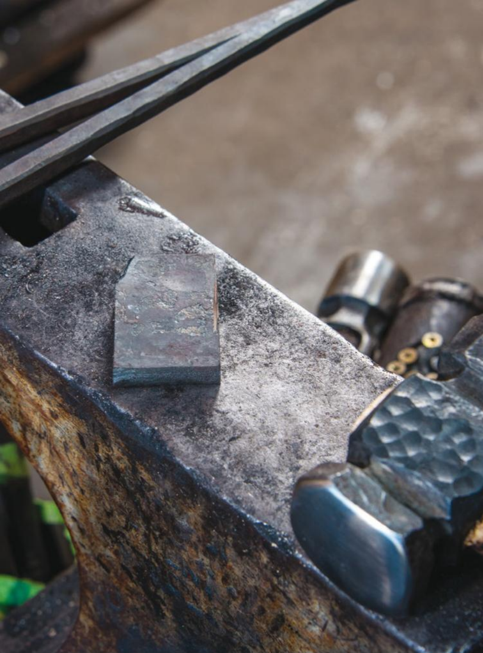
The billet of Damascus steel that Shea forged
