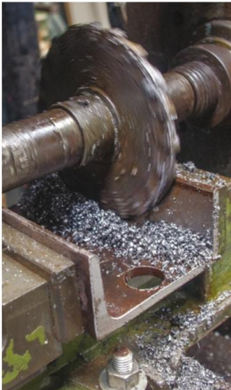
Above and below: Milling the sides of the channel Right: Drilling the axle holes
