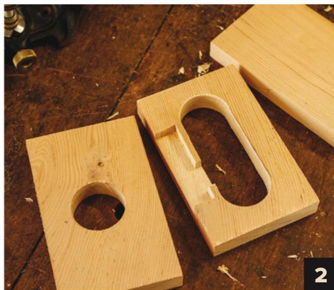
1. A drill press fitted with a 40mm diameter, carbide-toothed, Forstner-style bit was perfect for the job. This gave a smooth and clean hole that required minimal clean-up 2. Three pieces of wood prepared and ready to glue up
