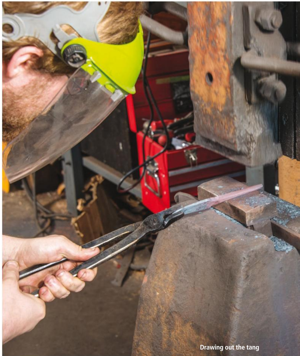
The anvil and hammer are still necessary to get the shape right
