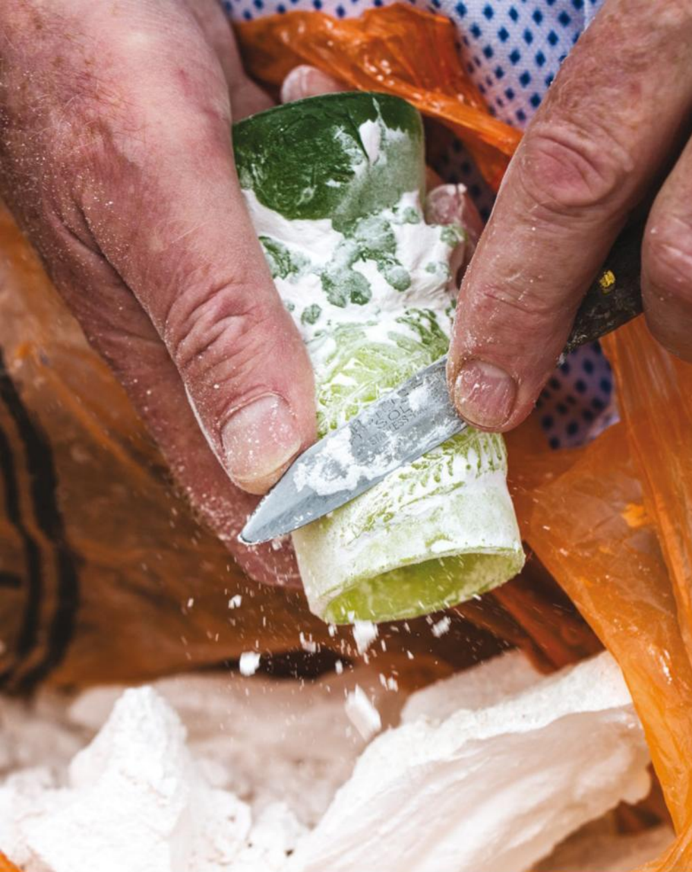
Using a peeling knife to gently remove the plaster mould from around the glass after kiln firing
