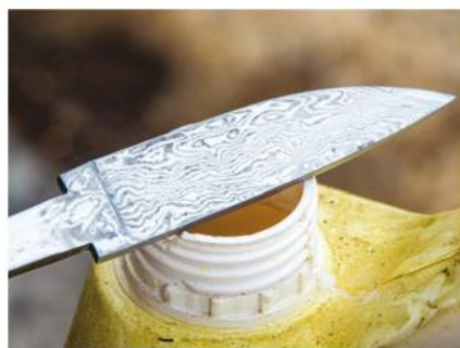
Clockwise from top left: Grinding the first of a succession of grinds; the blade after successive grinds up to 240 grit; the etched blade showing the Damascus pattern
