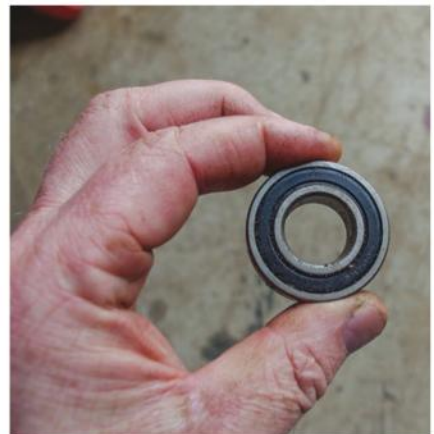
Left: Welded frame Below: 6004RS bearings Bottom: Axle assembly
