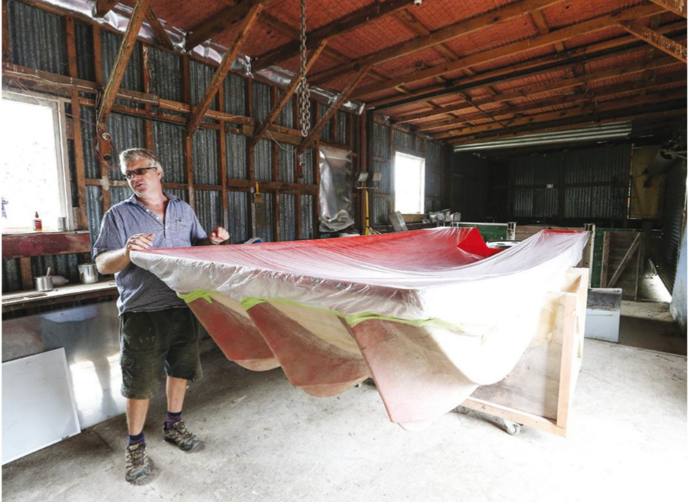
Another extension of the fibreglass side of boat building is this 4.2m trimaran that Max is developing as a fishing motorboat. It is made from two pieces — a hull and a deck. He says it will compete in the aluminium boat market
