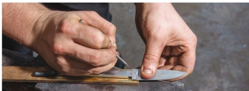
Far left: Etching in acid Left: Cutting out the slot to fit the tang Below: Marking the position of the tang for the first bolster
