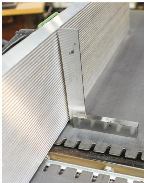
Top: The 12-inch Moore and Wright sitting on parallel blocks, ideal when an extra bit of height is required Above: Checking the fence on the planer
