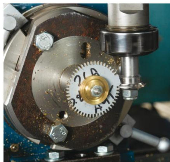
Left: A completed skeleton clock Right: The home-made tooth cutter at work
