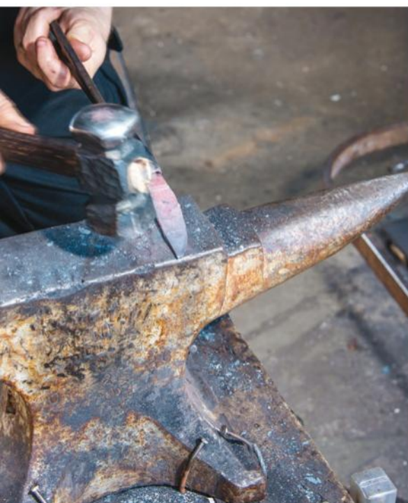
Above: Reheating the knife blank Below: The knife taking shape from the hammer
