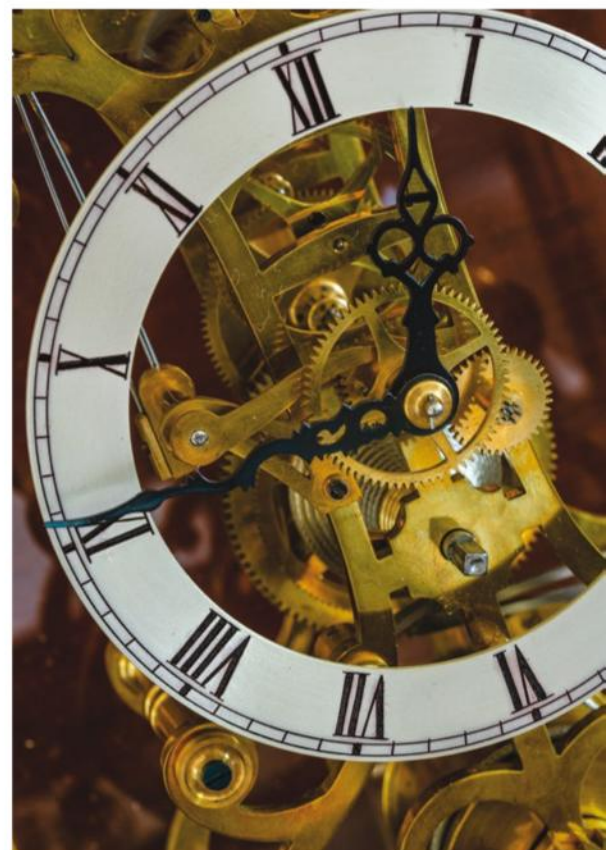
The inner working of a skeleton clock that David has made from scratch
