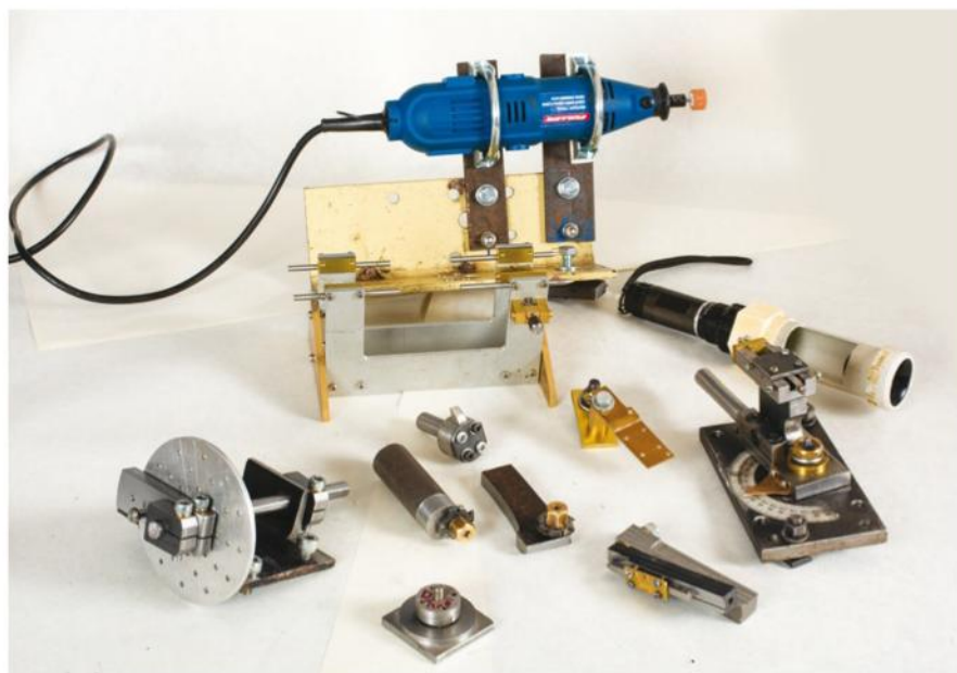
Above: A selection of tools that David has made to machine clock parts Right: A gear-tooth cutting tool ready for work Below: Details of skeleton clocks give an idea of the patience required to build one
