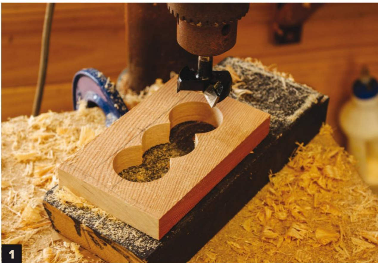
1. A drill press fitted with a 40mm diameter, carbide-toothed, Forstner-style bit was perfect for the job. This gave a smooth and clean hole that required minimal clean-up 2. Three pieces of wood prepared and ready to glue up
