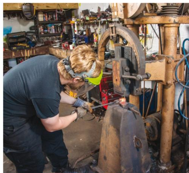
The power hammer saves time when drawing out the hot steel
