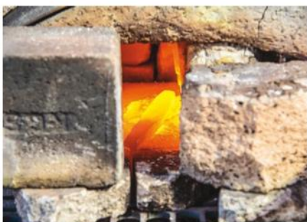
Above: Reheating the knife blank Below: The knife taking shape from the hammer
