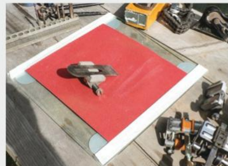
A Stanley 60½ plane cutter in an Eclipse 36 sharpening jig
