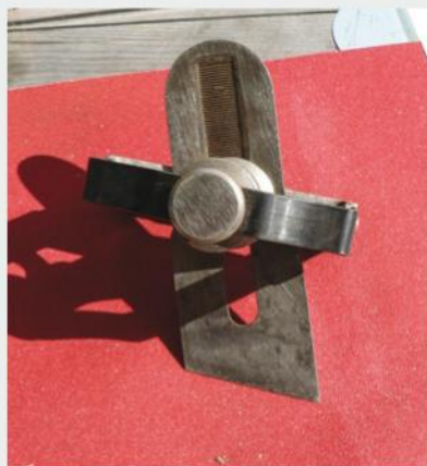
A Stanley 140 plane cutter in a Millers Falls 240 sharpening jig, which allows the edge to be sharpened at an angle
