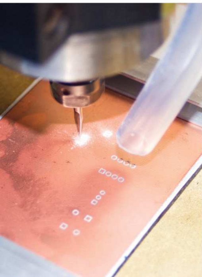
Below: the electronic circuit is engraved with a 300x300mm mill machine
