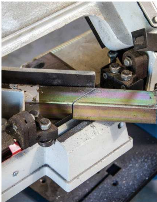
Cutting the parts of the frame
