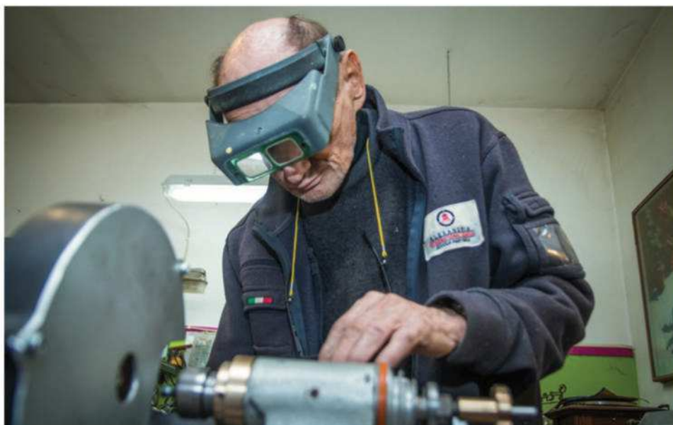
Above: Jewelry stones are about 140 times harder than metals. Over 60 years ago companies that specialized in building tools for extra hard metal machining, started building synthetic diamond tools for hard jewelry stones machining. Nowadays we can choose using both sinterized or electrodeposited machining tools.
