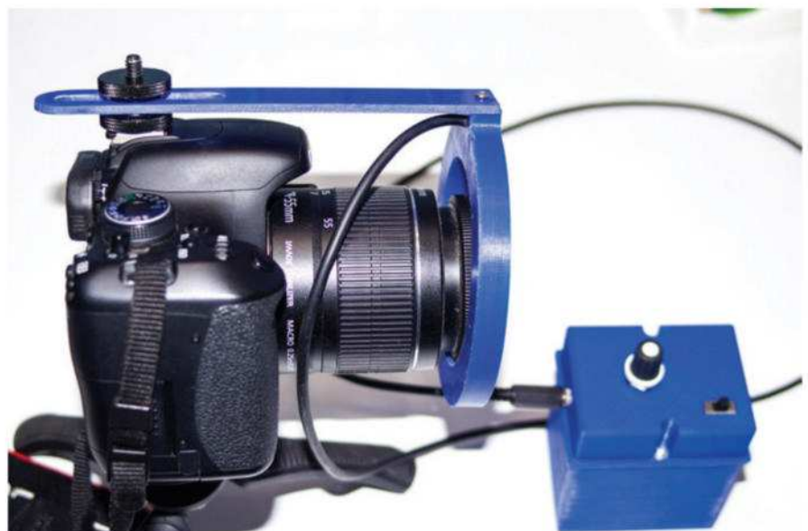
Right: this is a primitive version of the iris locking system that need some other modifications to work fine
