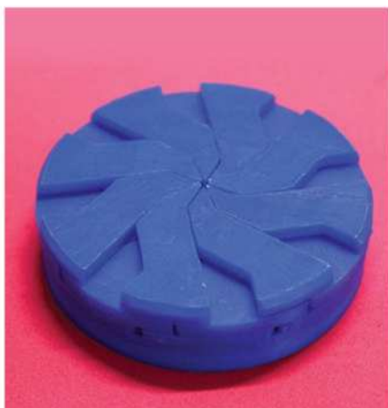
The first version of the modified iris box by Brien Allison ( www.myminifactory.com/users/Brien%20Allison ) that will lock the LED ring directly to the lens body
