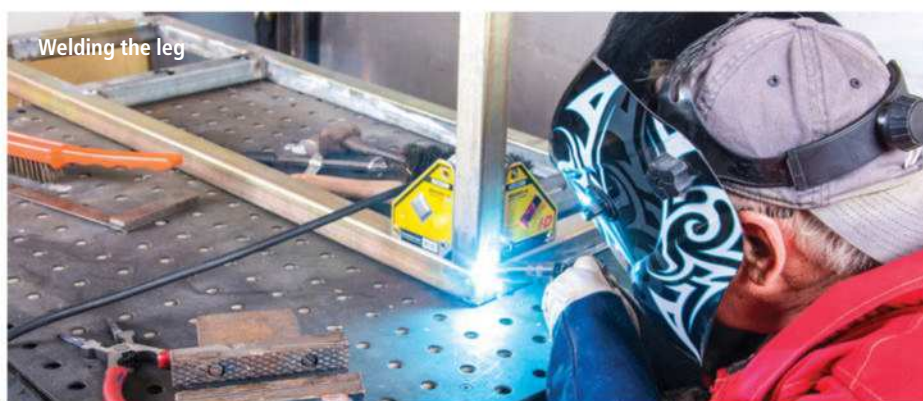
Welding a cross member to the legs. Note the timber support
