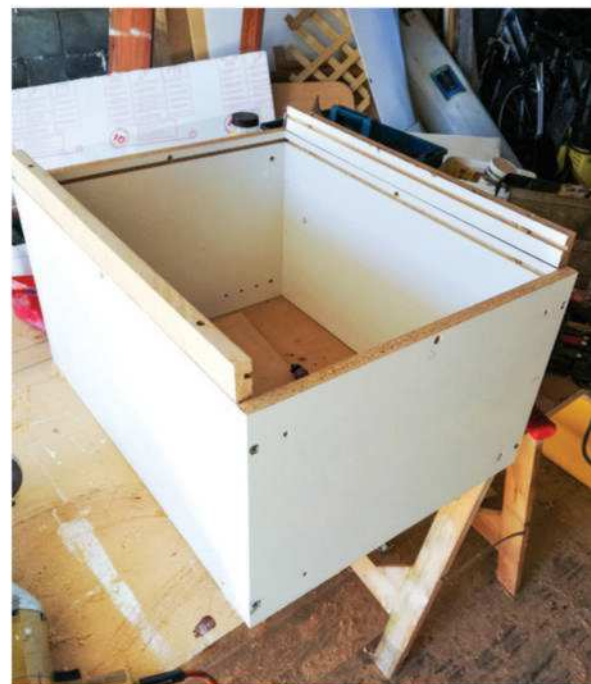
Making the cabinets deeper. The 40mm wide strips are dowelled, glued, and screwed in position. The slot to locate the rear panel has been moved 40mm back, and the original slot filled
