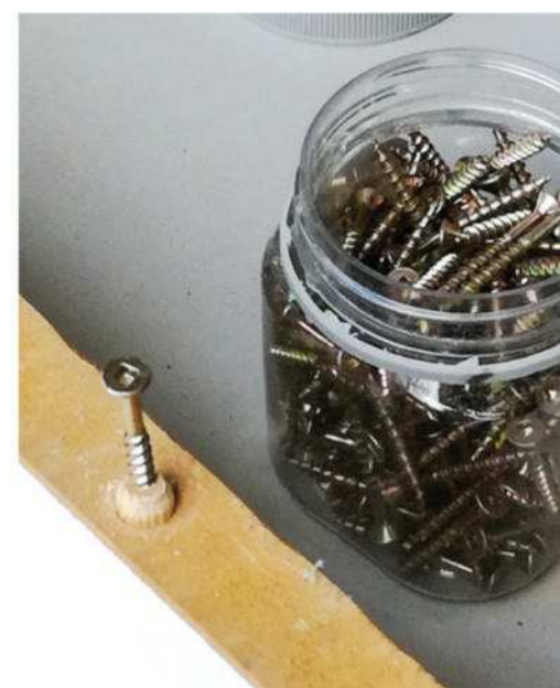
Below left: drilling holes for shelf support pins in the new bookcase space. Below right: sometimes you overdrill the dowel holes and have to retrieve the dowel before you glue them.
