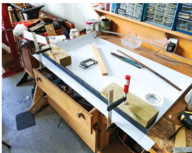
Folding the stainless steel base on my workbench. I used a folder to do the two ends, clamped the base to the workbench, and the peened the front edge down over a length of angle iron and used the same technique to fold up the rear edge
