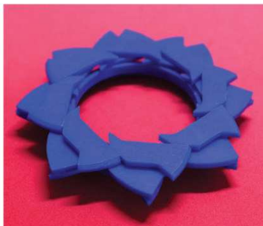
The first version of the modified iris box by Brien Allison ( www.myminifactory.com/users/Brien%20Allison ) that will lock the LED ring directly to the lens body
