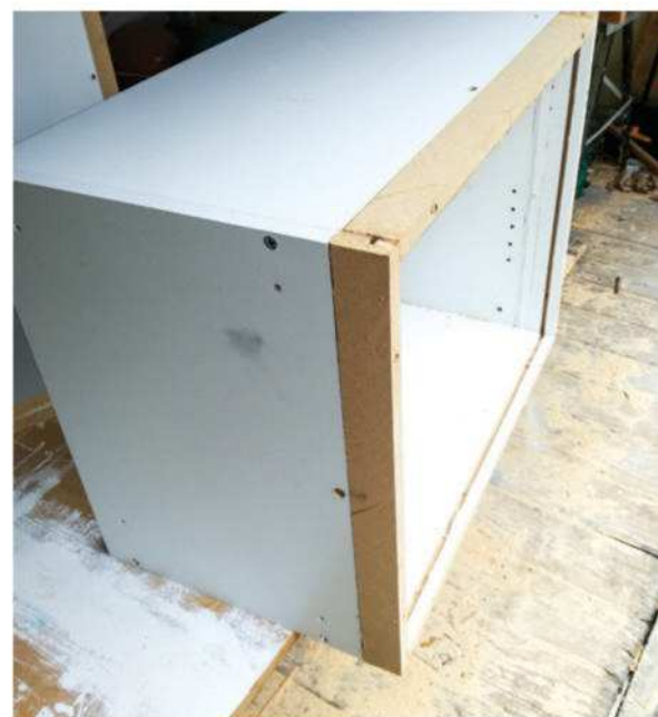
Making the cabinets deeper. The 40mm wide strips are dowelled, glued, and screwed in position. The slot to locate the rear panel has been moved 40mm back, and the original slot filled
