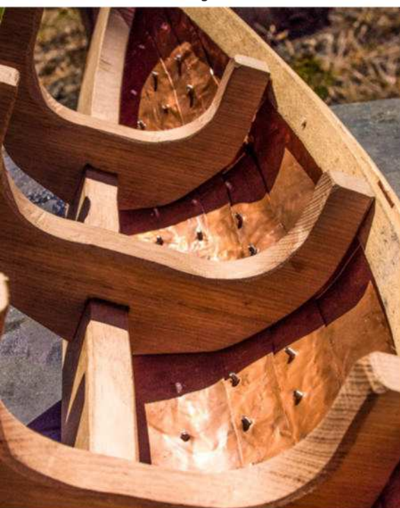
Below: The hull under construction, showing the keel and frames
