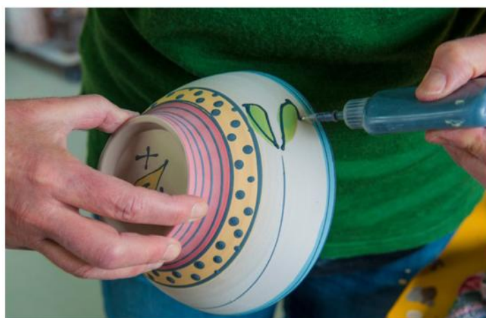
The application of decorative colours by brush. After this, the raised slip is squeezed on from a plastic bottle
