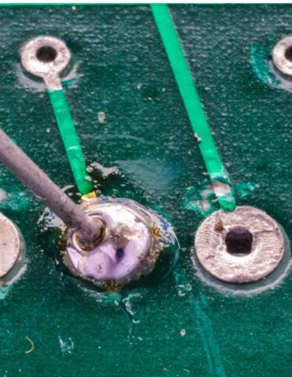
Here the solder has not adhered to the component lead either due to oxidation or use of the wrong technique
