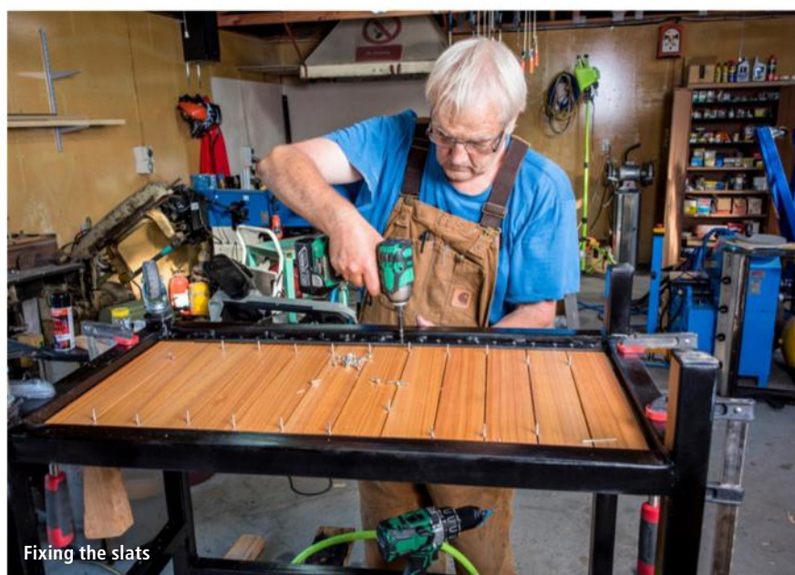
Drilling the screw holes for the lower shelf
