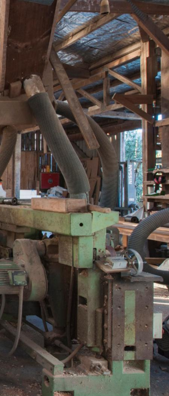
Above: Lloyd makes all the knife steels by hand, cutting new ones to specific profiles if they are not already in his collection. It takes a good eye and a fair bit of maths to replicate the negative detail of samples to be copied. He has 200 little patterns and drawers of curved knives and set-up gauges in the workshop
