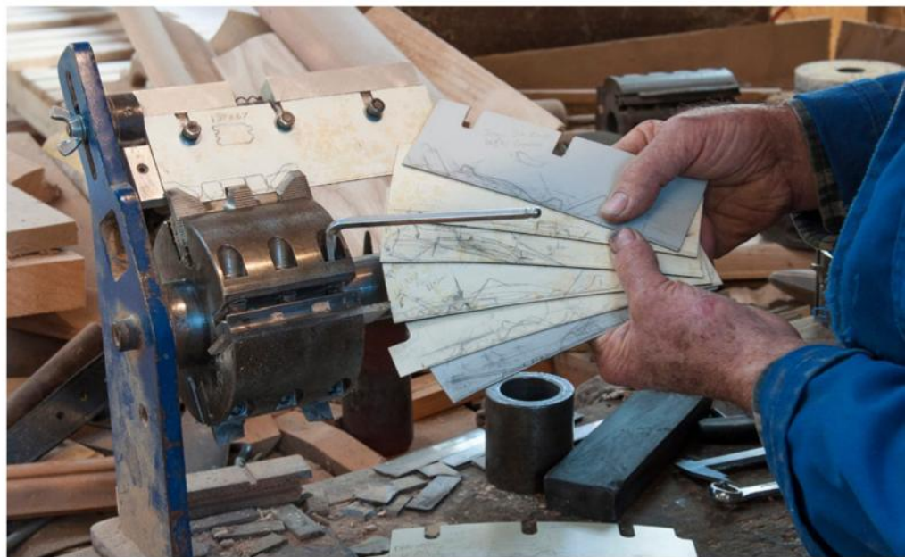
Above: Lloyd makes all the knife steels by hand, cutting new ones to specific profiles if they are not already in his collection. It takes a good eye and a fair bit of maths to replicate the negative detail of samples to be copied. He has 200 little patterns and drawers of curved knives and set-up gauges in the workshop
