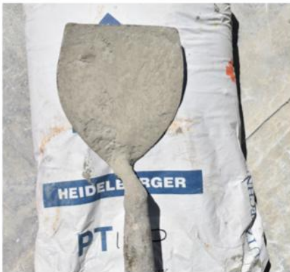
Above and below: The flick coat can be applied with a cut down block layer's trowel
