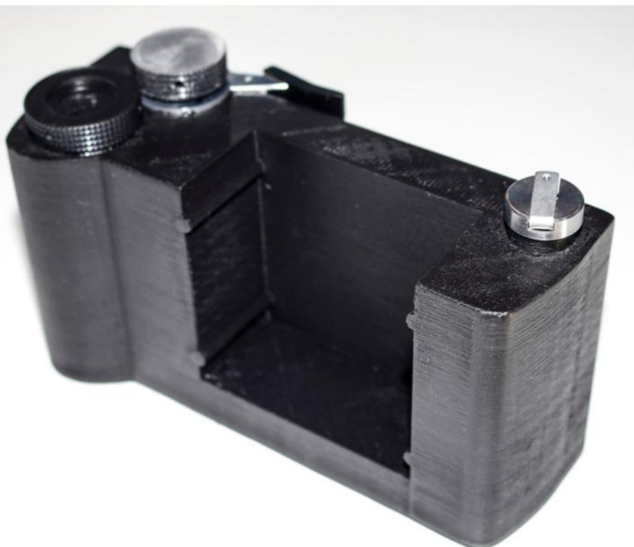
The finished model of the camera body (above) with the Aluminium M43 ring for the lenses and the finished analog back model (below).
