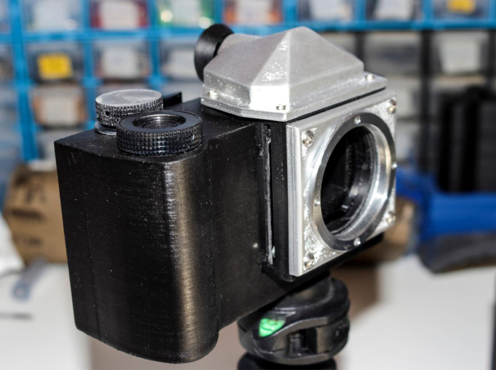
The finished model with a lens mounted on it. This should be the camera skeleton structure. The industrial designer's crew will start from this model to "dress" the object with the final plastic components like the hand grip, external texture, protection parts and connector closures
