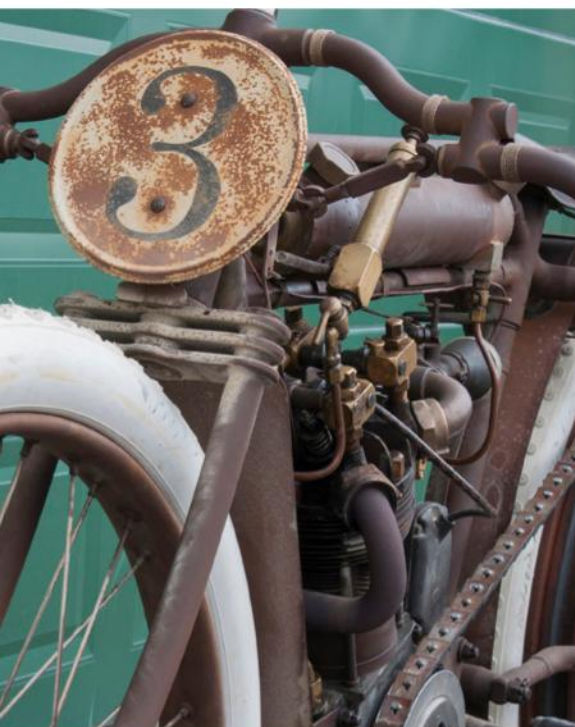
The reproduction racing number was made from an old biscuit tin. The rods controlling the throttle can also be seen
