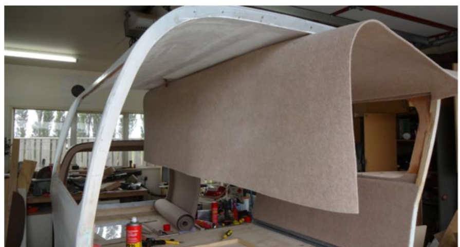
Gluing the upholstery fabric to the pod interior
