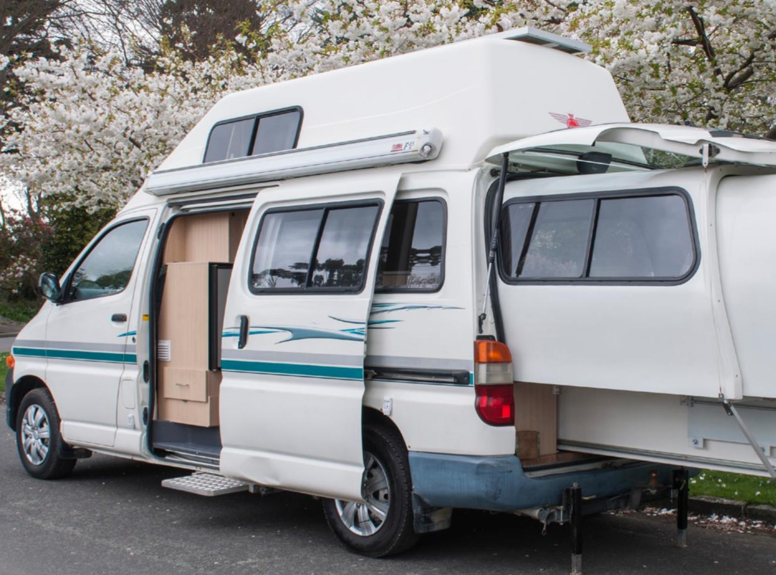
The fully expanded camper van with telescopic pod supported by jacks and legs
