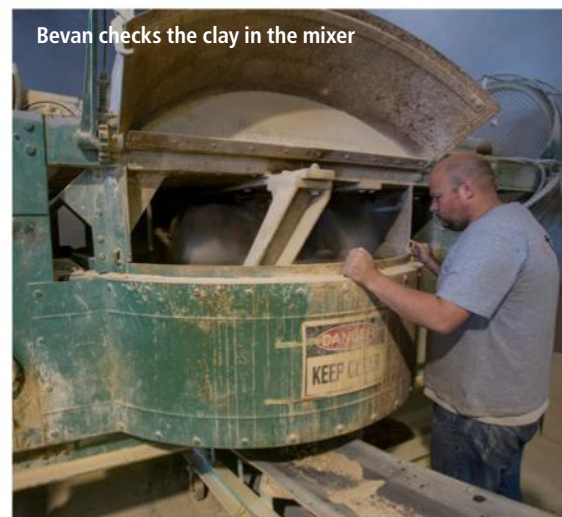
Final check of the mixed clay to ensure the correct consistency
