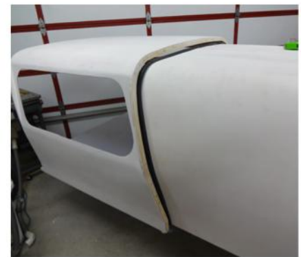
First coat of paint
