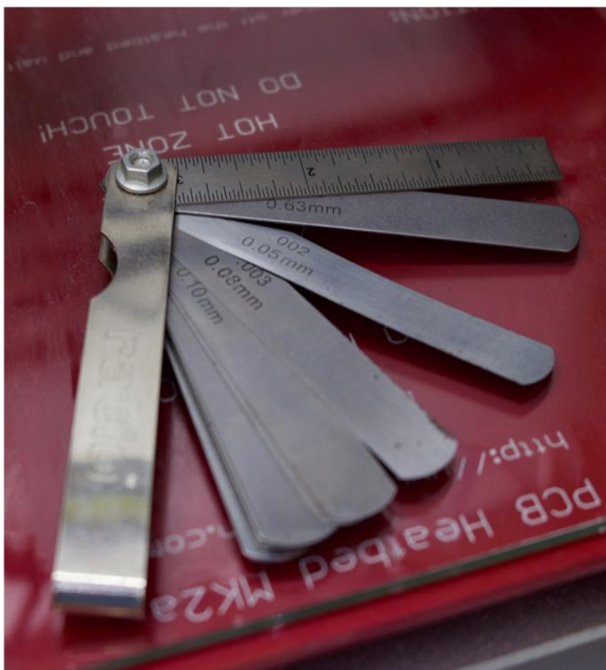
Above and below: The mechanical feeler used in the bed calibration process
