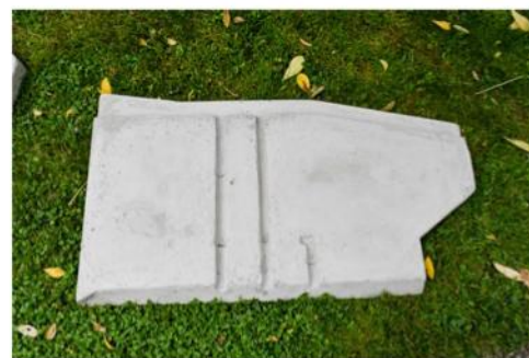
The side and bottom firebricks of the firebox
