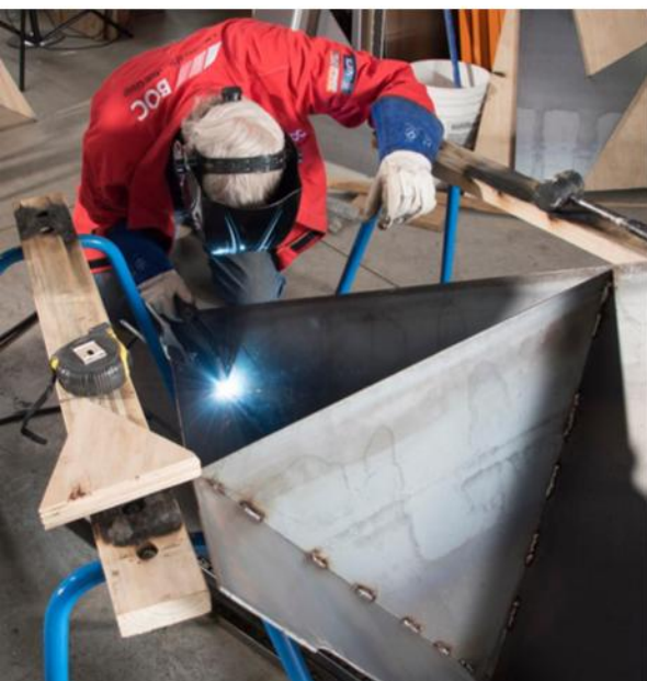
Below left to right: Welding the sides from the inside The sides and shelf welded Forcing the sides to fit
