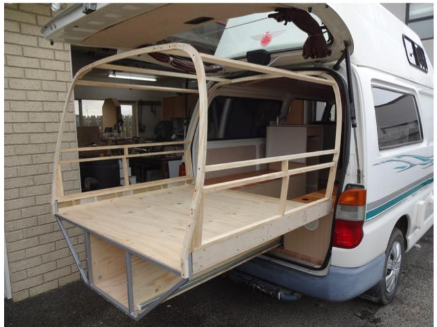
The second pod ready for the installation of the bendy ply
