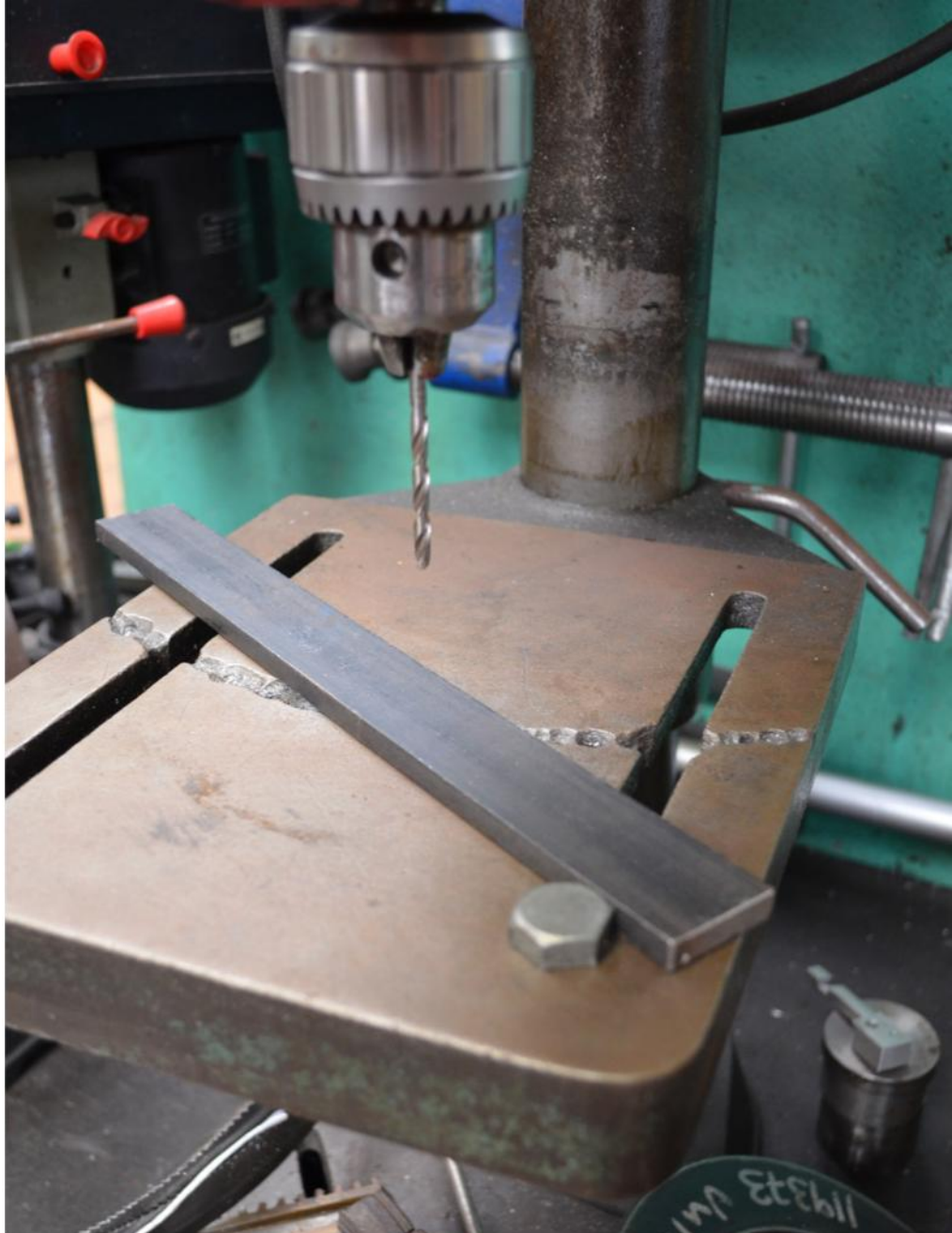
Right: The job is held against a bolt put in the drill-press-table slot
