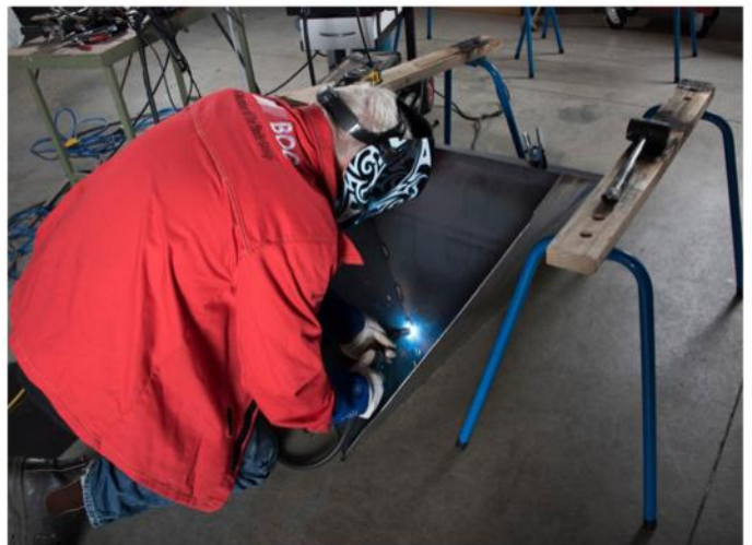
Tacking the sides. The lack of a flat plane made clamping awkward
