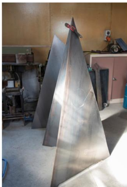
Sides clamped in place
