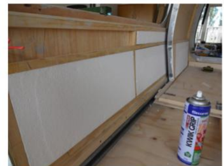
Gluing the upholstery fabric to the pod interior
