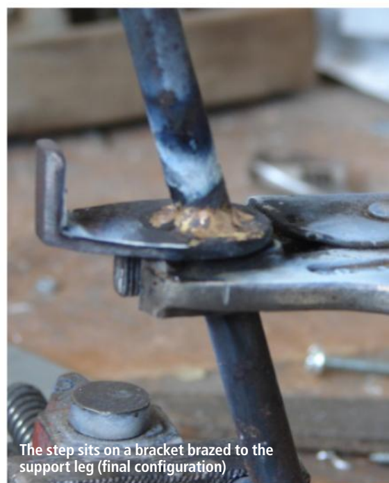
I heated the support legs with a gas torch and bent them round a jig
