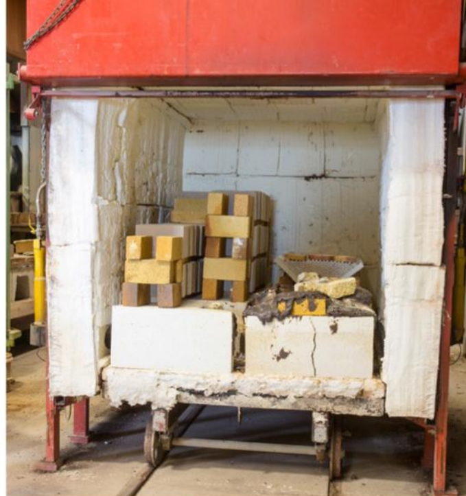
The bricks are loaded into the furnace for firing. The furnace is capable of holding two tonnes of bricks per fire
