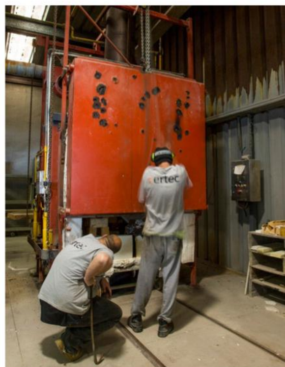
The bricks are loaded into the furnace for firing. The furnace is capable of holding two tonnes of bricks per fire
