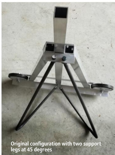
Setting up the diagonal supports which hold the vertical tube in position
