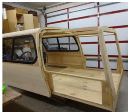
The second pod ready for the installation of the bendy ply
