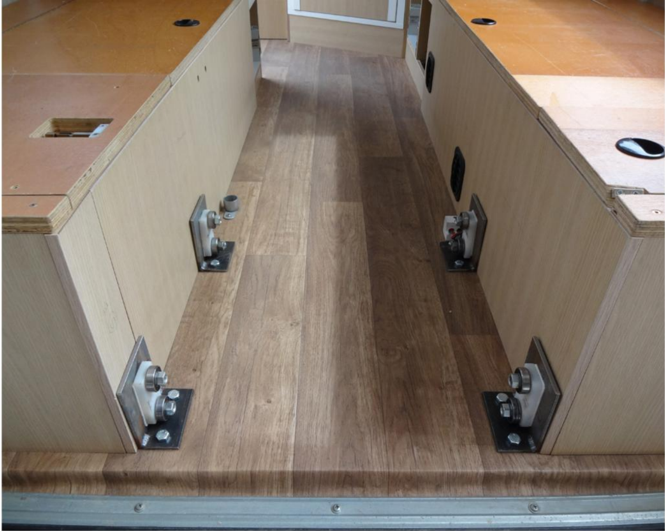
Eight ball bearings mounted on steel brackets support the slide-out
