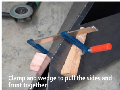
Shaped timber to align the sides to the front
