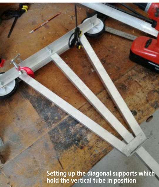
Original configuration with two support legs at 45 degrees
