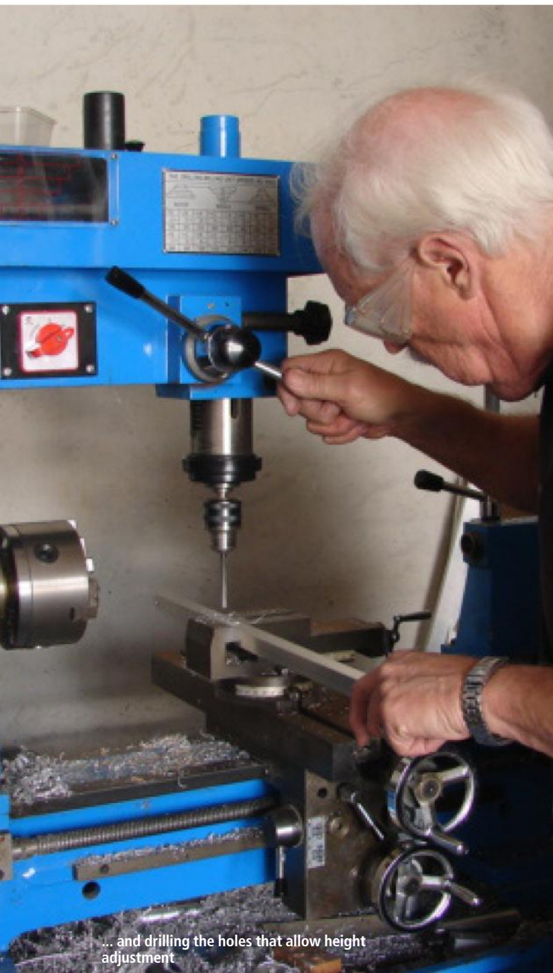
The step support bracket taking shape
