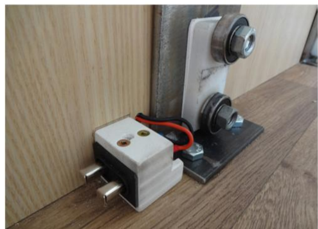
When fully extended, the pod makes electrical contact for the LED lights
