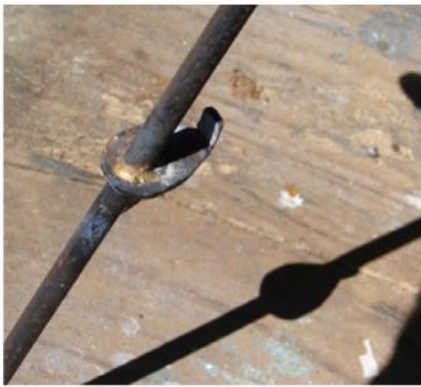
The step support bracket brazed in the right place at the correct angle ...
