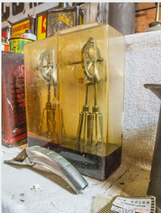
Below: The heavy-duty oil stabilizer is a two-chambered clear plastic container with an egg beater in each compartment to whisk the motor oil to prove which was the best lubricant and had the best clinging power
