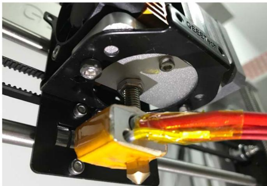
Bottom view of the 3D printer extruder, design reviewed by the producer. Credit: geeetech.com
