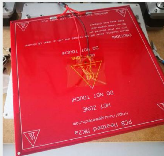
Below: Hot bed PCB bottom side. Note the thermocouple positioned around the middle of the surface
