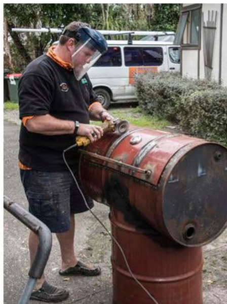
Cleaning up the welds
