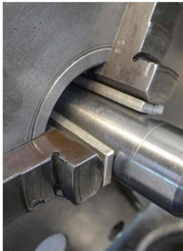
Aluminium strips protect against chuck jaw marks
