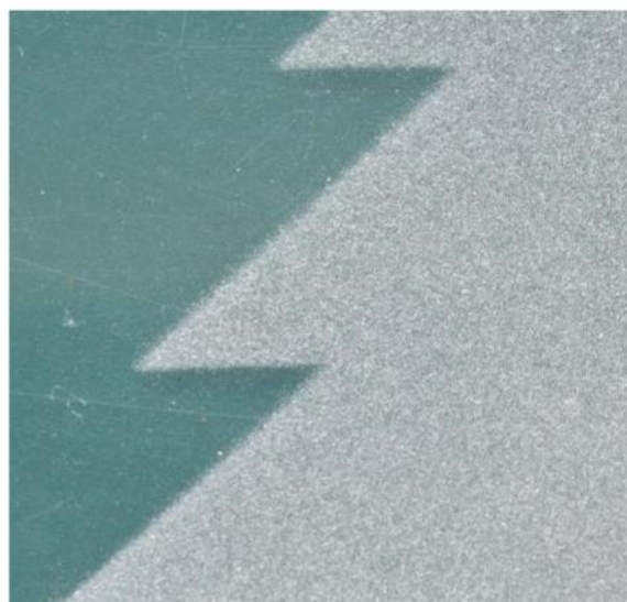
Edge definition after blasting
