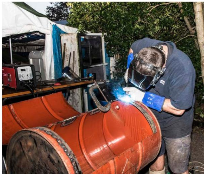
Above: Plug welding the edge pieces Left: Punching the holes for the plug welding Below: Joggler and punch plier
