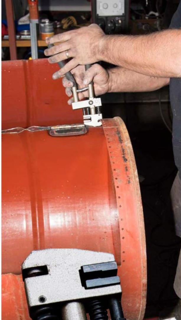
Above: Plug welding the edge pieces Left: Punching the holes for the plug welding Below: Joggler and punch plier
