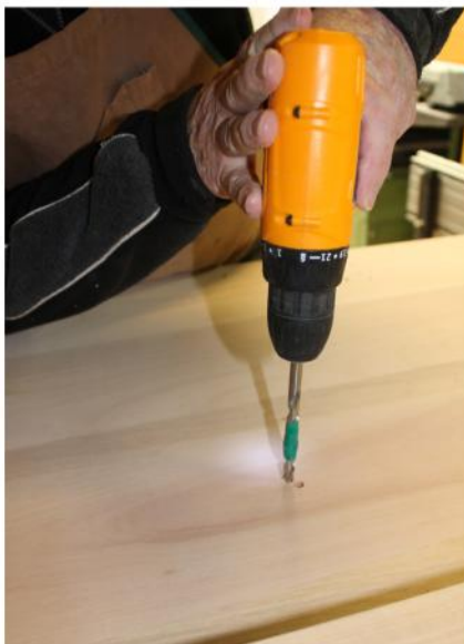
Drilling for and fitting the threaded inserts
