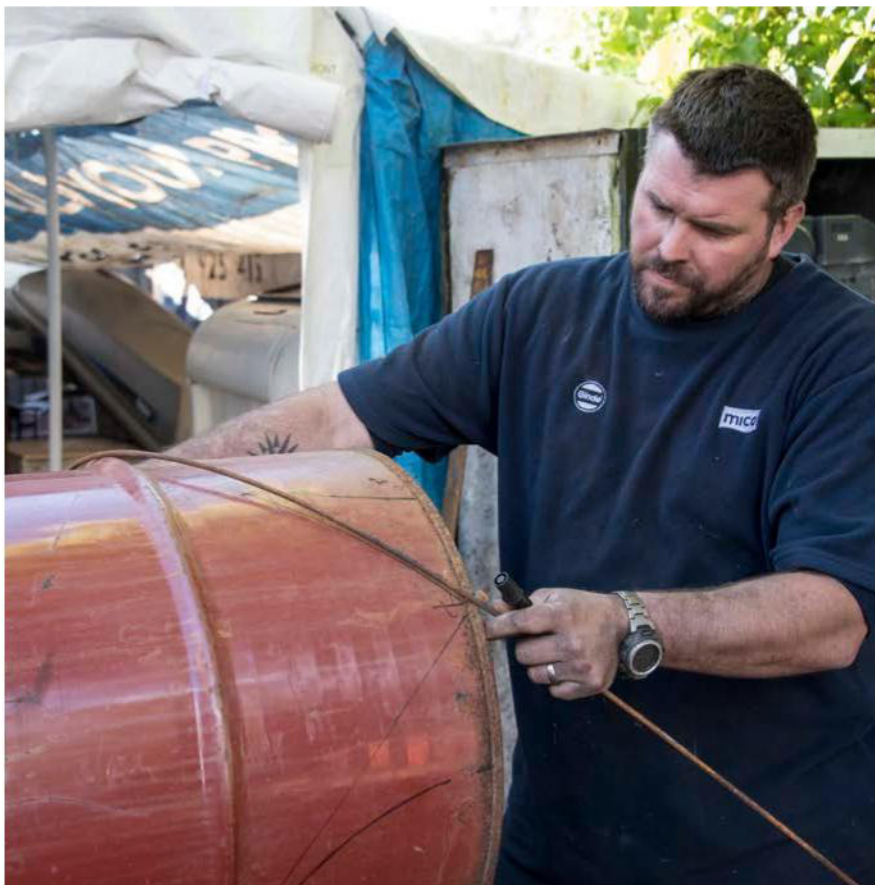
Evan Wade laying out the shape of the two-barrel joint
