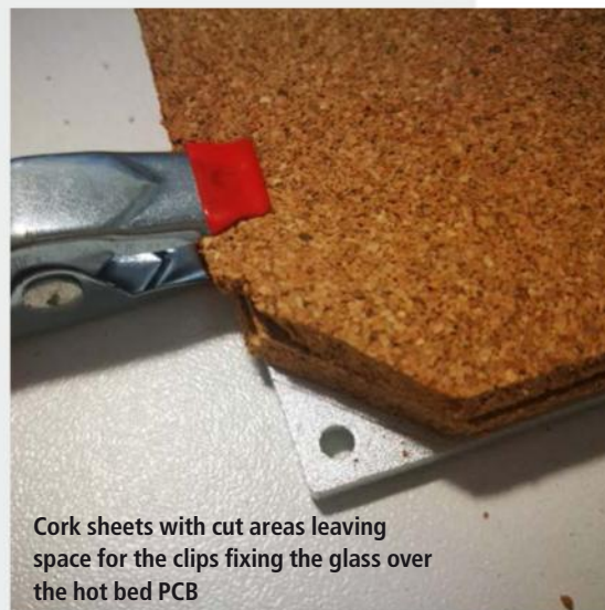
Below: Cork sheets with cut areas leaving space for the clips fixing the glass over the hot bed PCB
