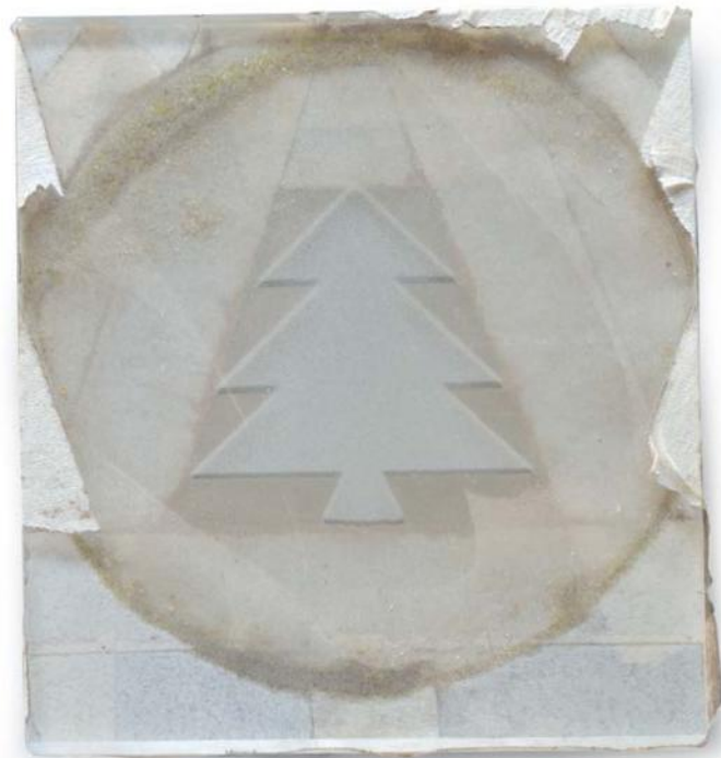
After sandblasting. Note how much media got under the stencil
