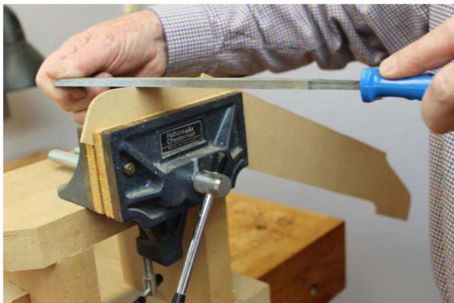
Finishing the base template
