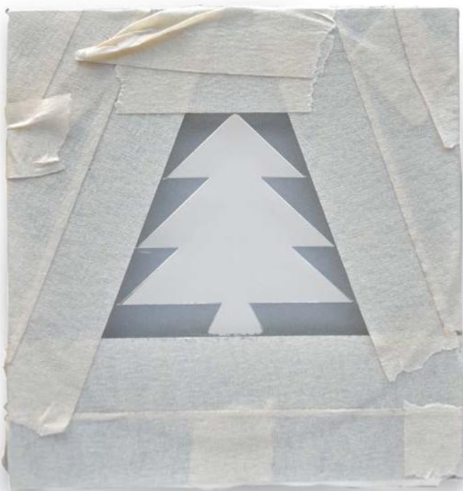
Sandblasting using a stencil
