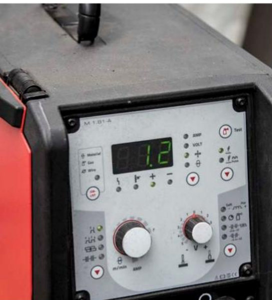
Thickness setting for attaching the two drums
