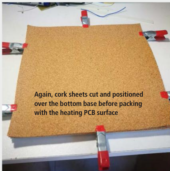
Below: Cork sheets with cut areas leaving space for the clips fixing the glass over the hot bed PCB
