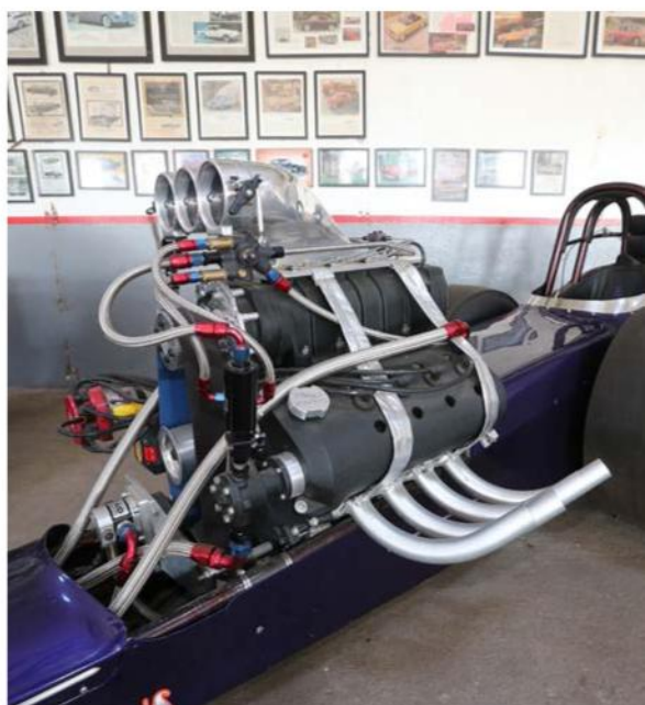
Below: Parked up in the factory is Phil's brother Dave's rail drag car. It is driven by a 5.4 litre Ford Falcon BA 330
