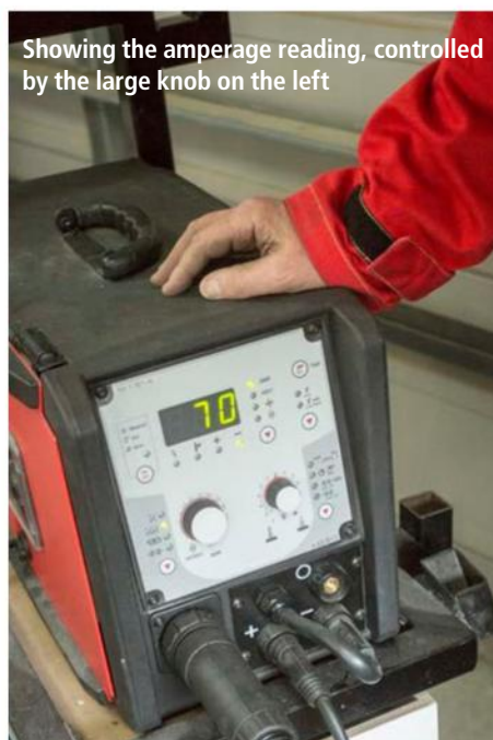
Setting up the BOC Smootharc Elite for TIG is simply a matter of selecting the job (127 for TIG)
