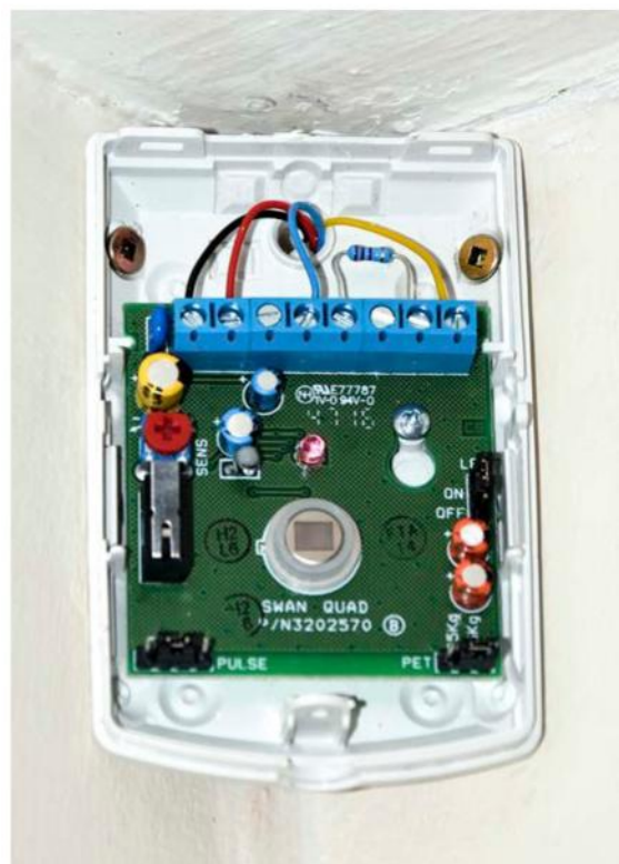
Wiring the PIR at ground level then fitted in the corner leaving clearance at the top
