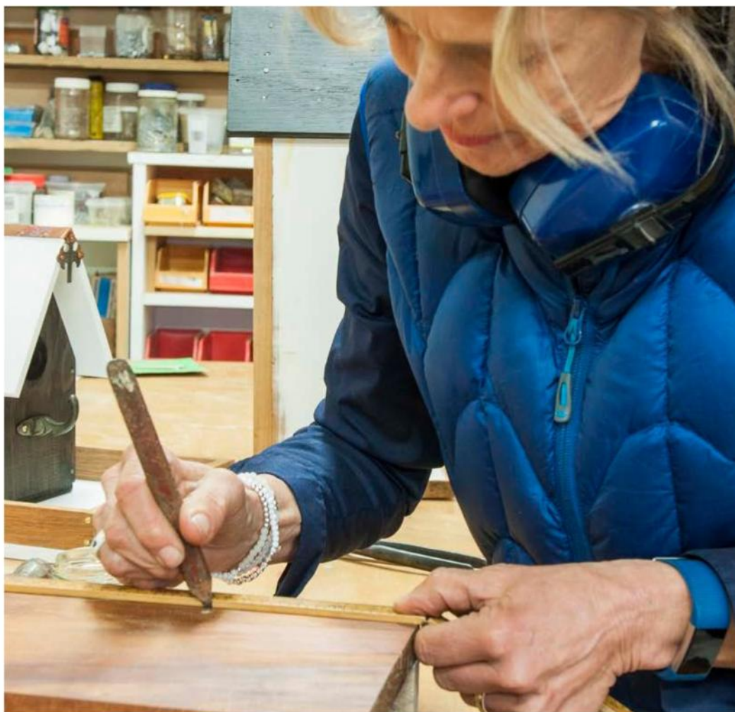
Megan marks the screw holes carefully before drilling
