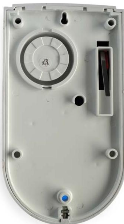
Unit is designed to be mounted vertically, evident by the moisture guard around the cable hole in the centre ( ... but they have left a hole above the tamper switch guard)
