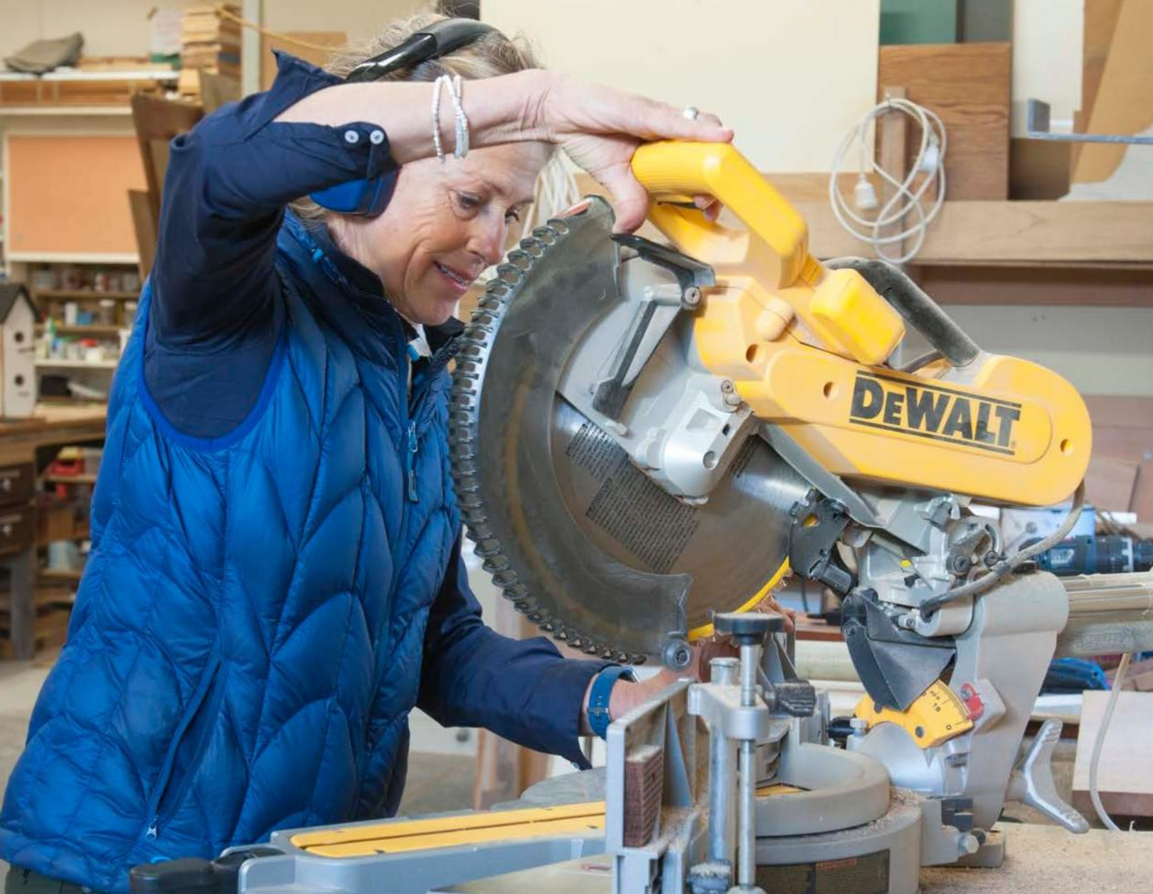
Megan uses the Dewalt drop saw to cut her mitred roof angles Below: Plenty of tools on hand in this community shed
