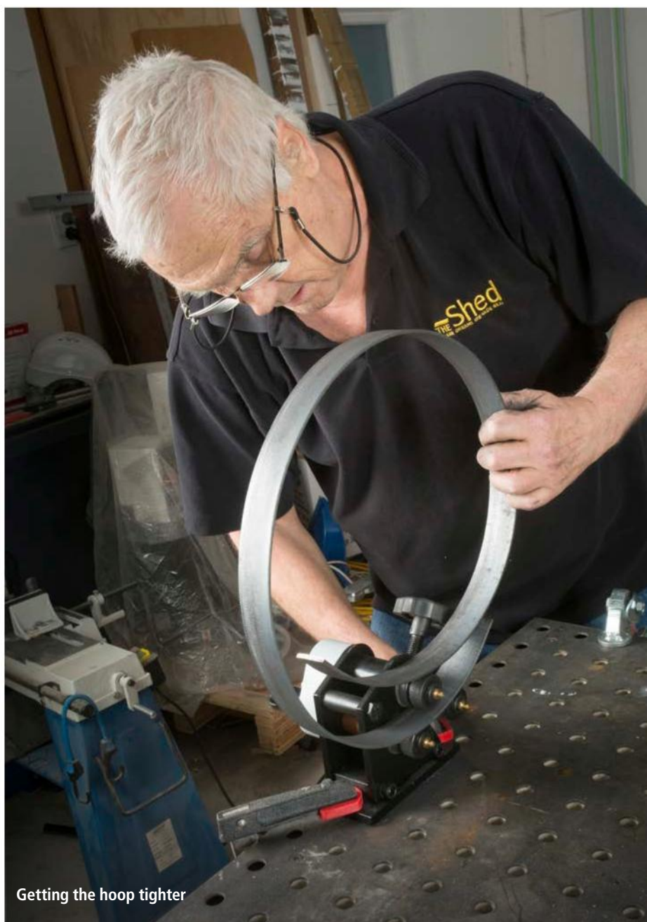
Rolling a flat bar for the seat ring
