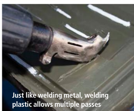
Using the Mark 2 Speed Welder
