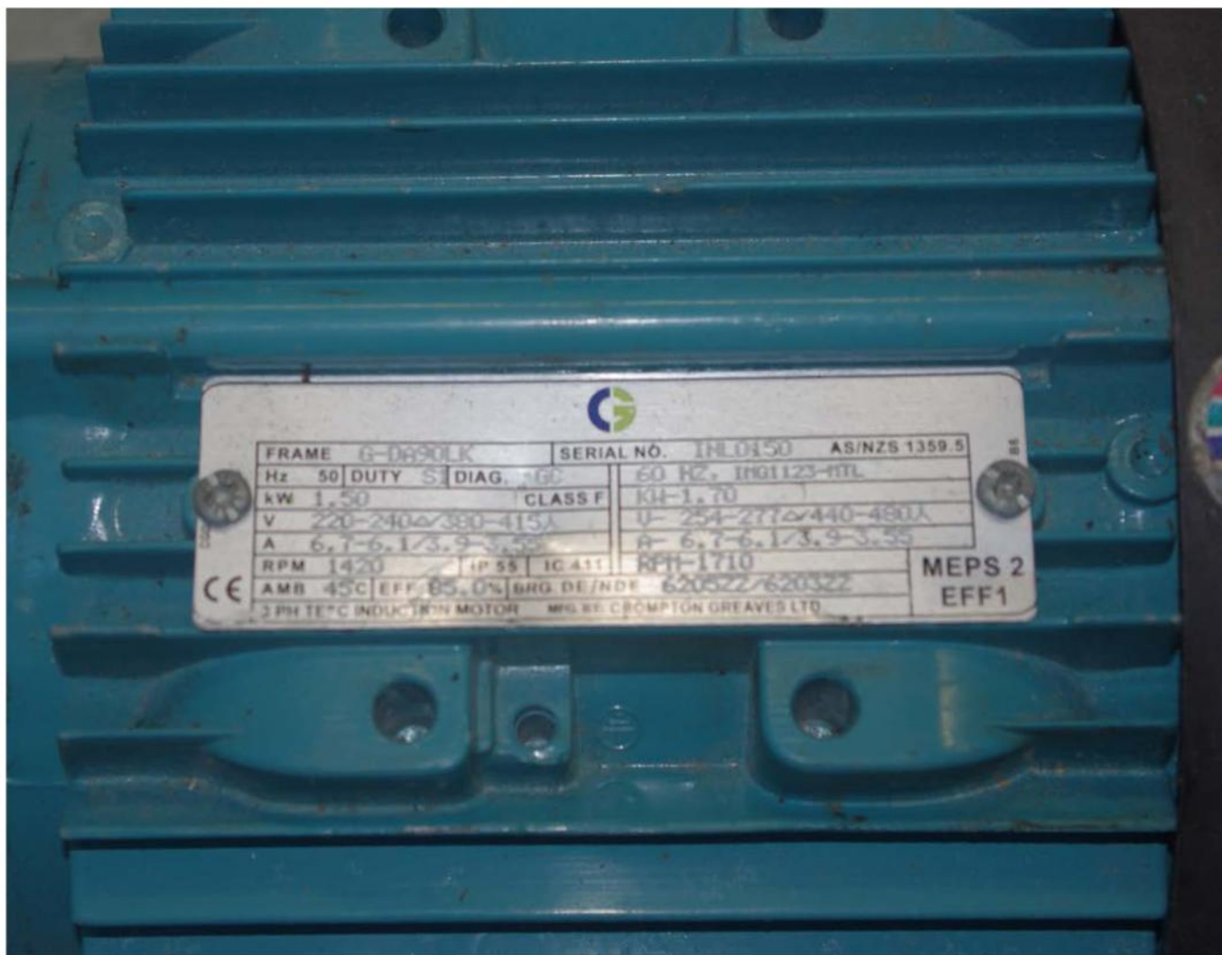
Motor name plate — dual voltage figures show this motor can be wired star or delta
