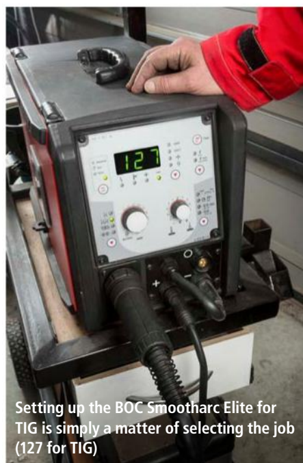
Showing the amperage reading, controlled by the large knob on the left
