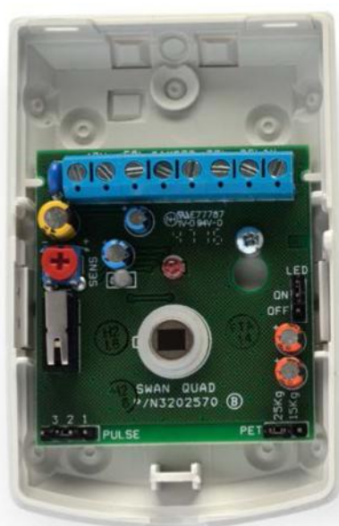
PIR and Cover. Note jumpers for settings and tamper switch on left
