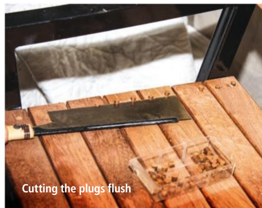
Cutting plugs for the screw holes
