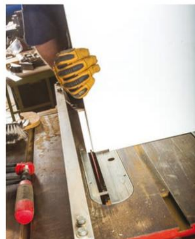
Cutting a rebate in the fixed shelf disguises the end of the rebate and makes the shelf look seamless
