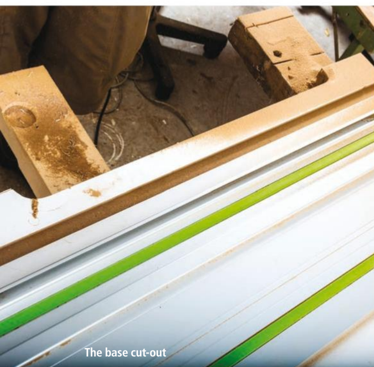
Cutting out the rebate for the fixed shelf; note the stop clamped to the piece
