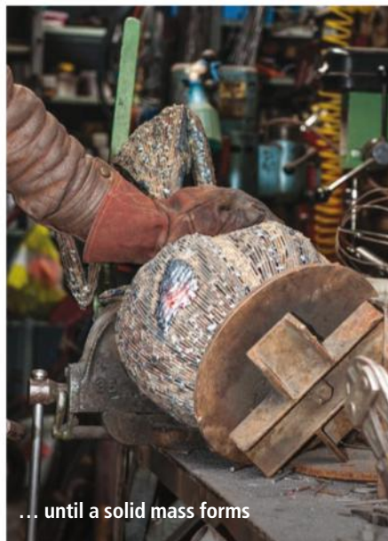
A figure showing the built-up mass of wires and tack welding
