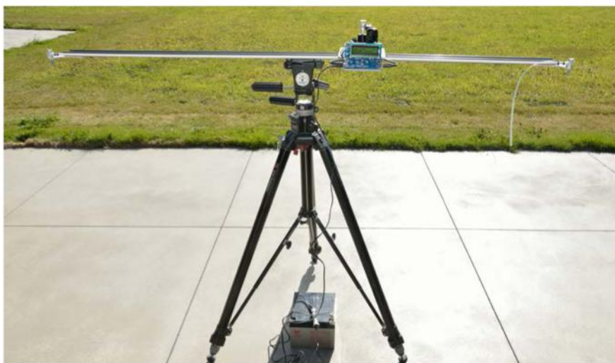
The rail and carriage assembly. Note the excess belt
