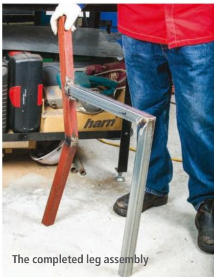
Welding the back leg
