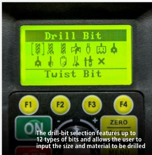
The Pilot Hole mode and Tapping Mode are accessed via the LED screen
