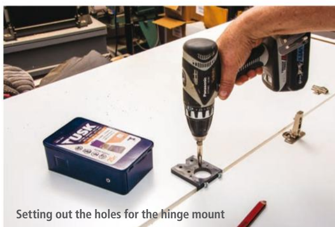
Reaching the right depth (12.5mm)
