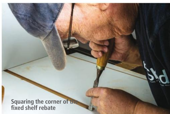
Cutting a rebate in the fixed shelf disguises the end of the rebate and makes the shelf look seamless
