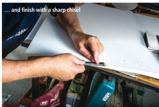
Trimming the edge tape. I usually start with a small plane ...
