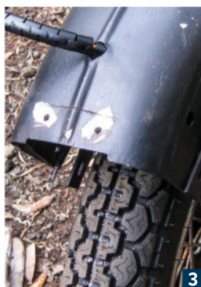
3. Remains of an old hinge ground off from the rear mudguard. 4. Finally attached; the switch wires can be seen in the headlamp shell
