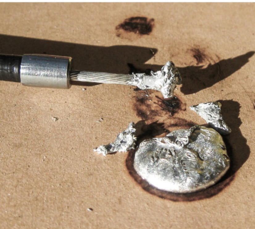
Above: Melting off the entire barrel anchor on the new Bowden cable. Right: The chopped end of the new cable is visible at the bottom; hammer, cold chisel, and vice also visible, and Sellotape to stop the inner cable from disappearing into the sheath
