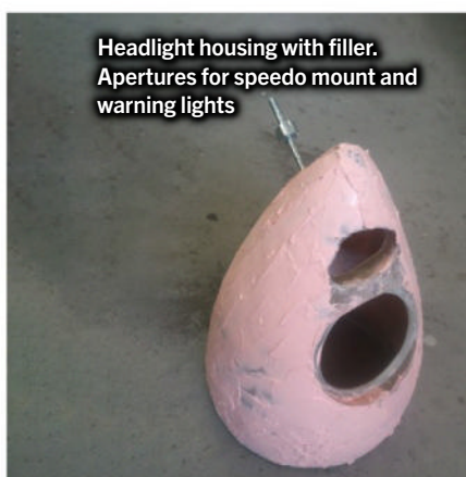
Headlight housing during application of primer-surfacer
