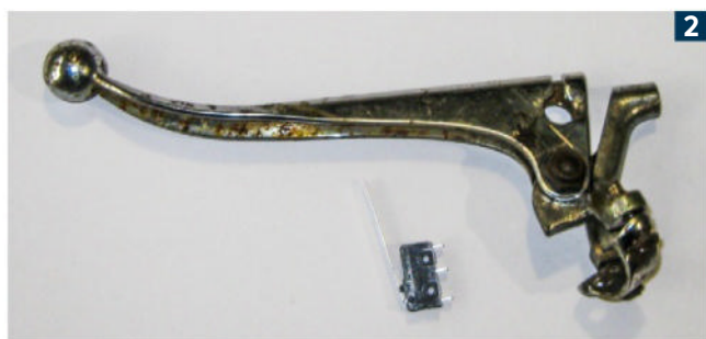
1. The hand (front) brake lever; easier to fit a switch on this rather than down by the wheel. 2 and 3. An SPDT miniature switch from Jaycar easily handles 6V and milliamps of current for the brake light – positioned here with the hand lever
