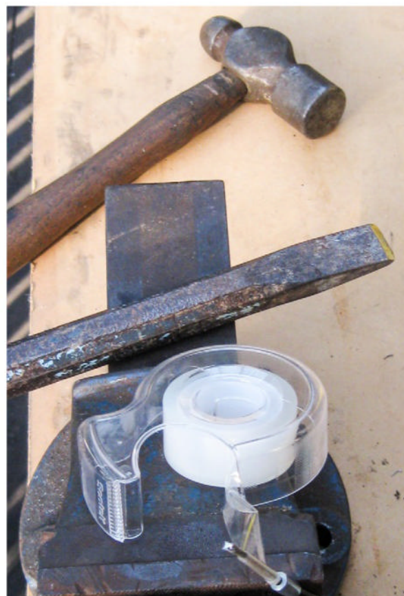
Above: Melting off the entire barrel anchor on the new Bowden cable. Right: The chopped end of the new cable is visible at the bottom; hammer, cold chisel, and vice also visible, and Sellotape to stop the inner cable from disappearing into the sheath
