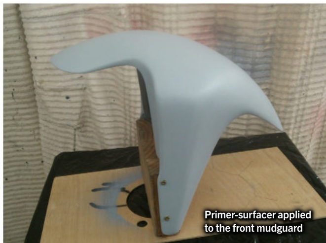
1998 RS125 race bike front mudguard mould being used to make the foundation section for the CGR916
