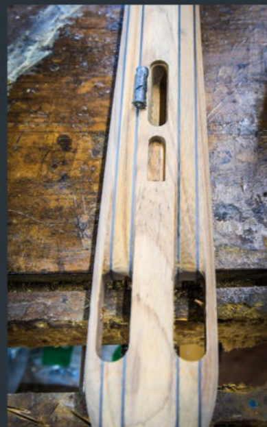
A lead slug ballast beside the cavity housing to complete the buoyancy calibration
