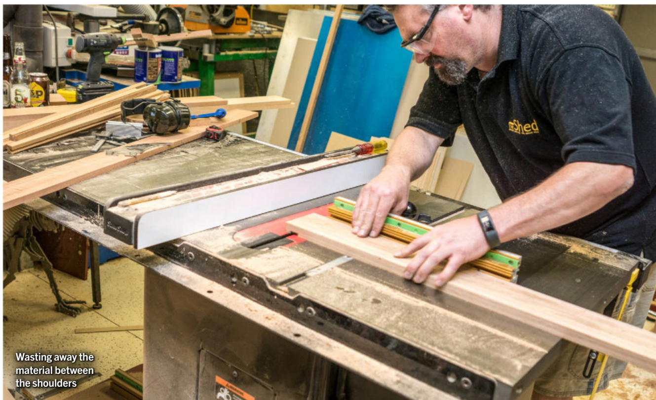
Cutting the tapered box front of the tapered boxes on the table saw
