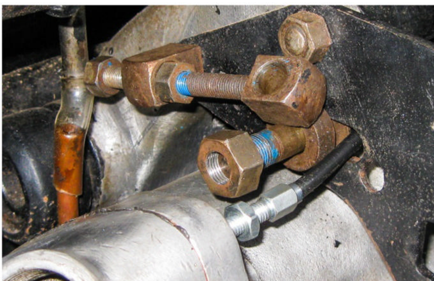
The cable adjuster screws into the gearbox shell: instead of the small hole in the frame plate, the cable goes through the adjustment slot for less kinking. Bowden fittings would still have had to be removed
