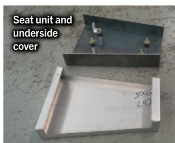
Bench mock-up of under-seat electrical equipment
