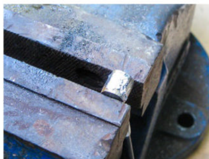
The anchor for the new cable soldered in place
