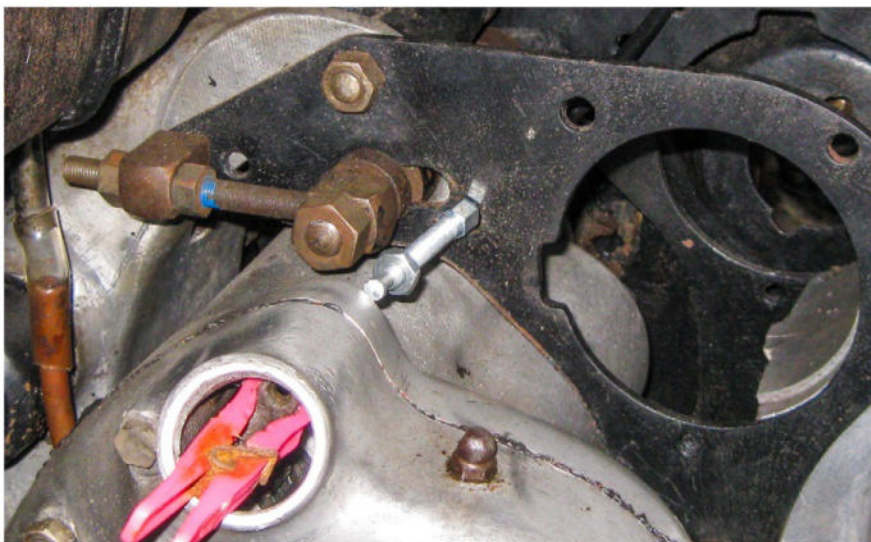
The clutch cable threaded through the small hole in the frame plate. The barrel anchor is to go up at the handlebar control lever. The pink peg holds the clutch lever
