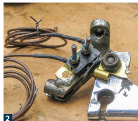
1. The switch is also bolted, double-nutted, and threads fingernail polished to give security; the switch lever is cut back, and another piece of brass hinge makes a trigger; blobs of solder lock the trigger in place relative to the handle. 2. Wiring soldered, and heat shrink insulation over the joints – this view is the underside of the handle
