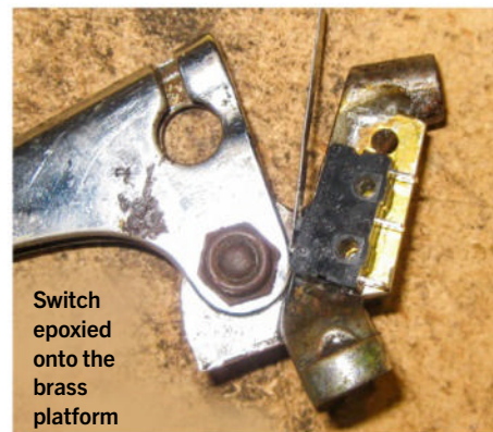
The brass platform has been soldered and epoxied onto the brake lever pillar. The switch fits on
