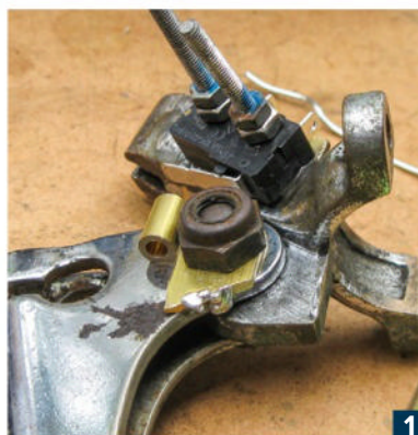
1. The switch is also bolted, double-nutted, and threads fingernail polished to give security; the switch lever is cut back, and another piece of brass hinge makes a trigger; blobs of solder lock the trigger in place relative to the handle. 2. Wiring soldered, and heat shrink insulation over the joints – this view is the underside of the handle
