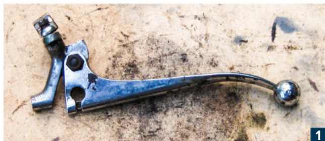
Bits of outer removed, the ferrule pushed back on, and no sign of any damage to the inner
