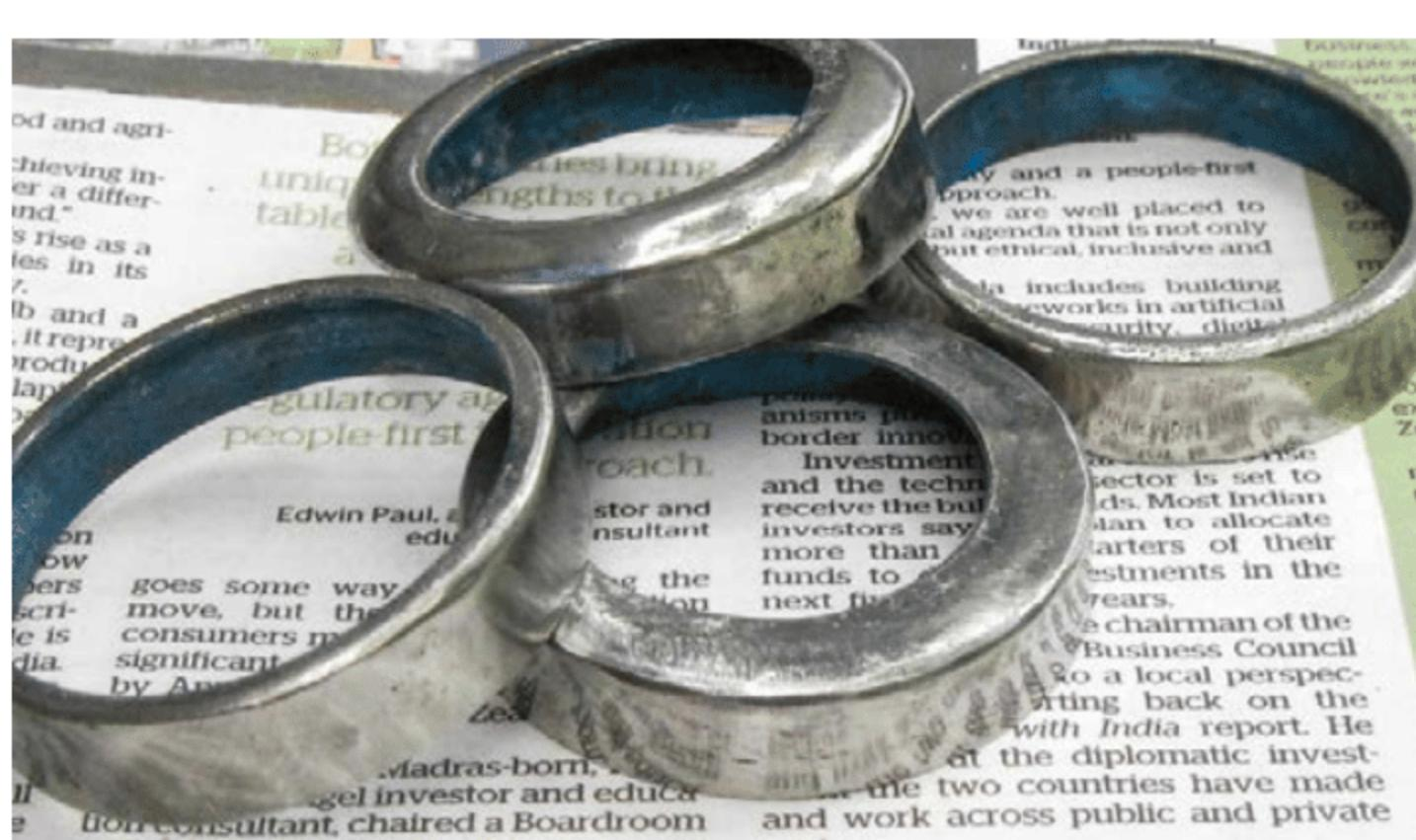
The rings for the headlamp tubes have been plated with nickel
