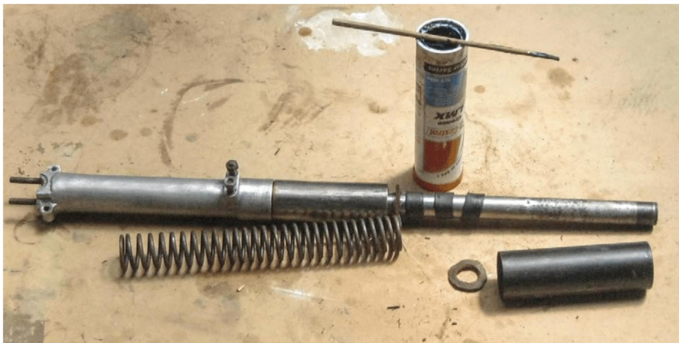
One leather washer in place for the mainspring, and three rubber rings
