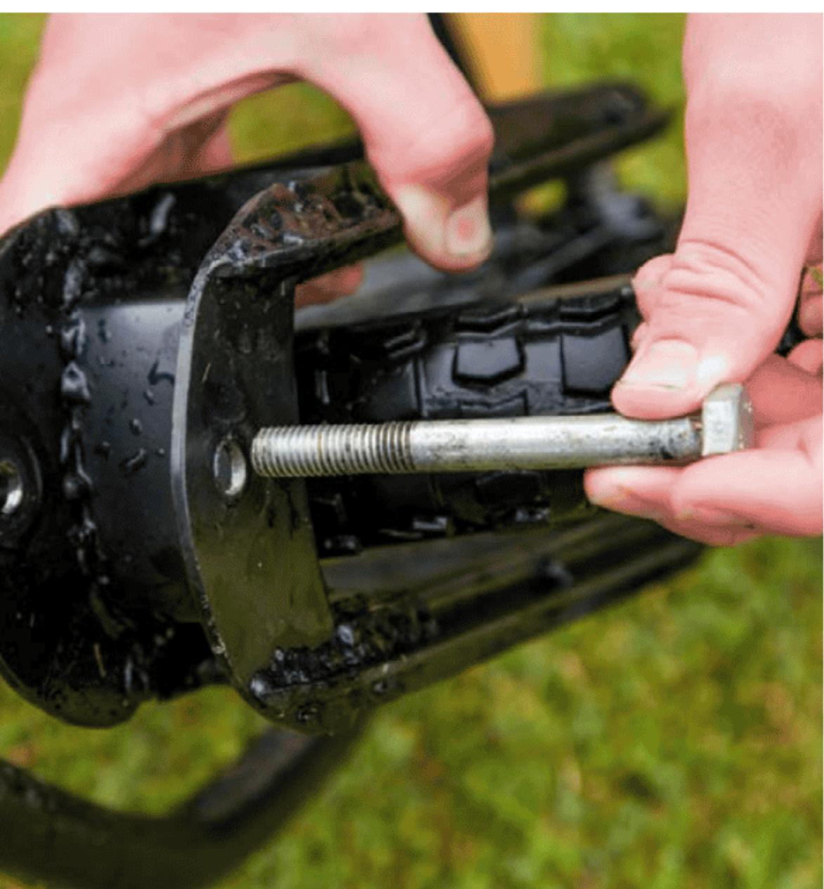
Swing arm attaches through bearing
