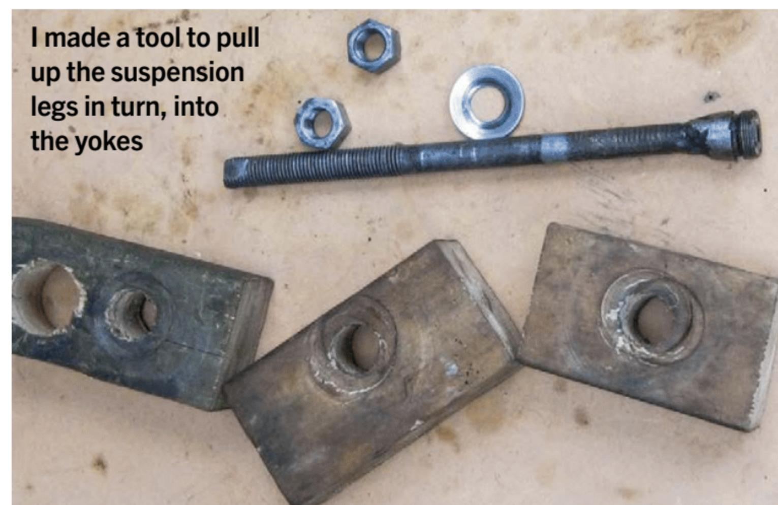
I made a tool to pull up the suspension legs in turn, into the yokes
