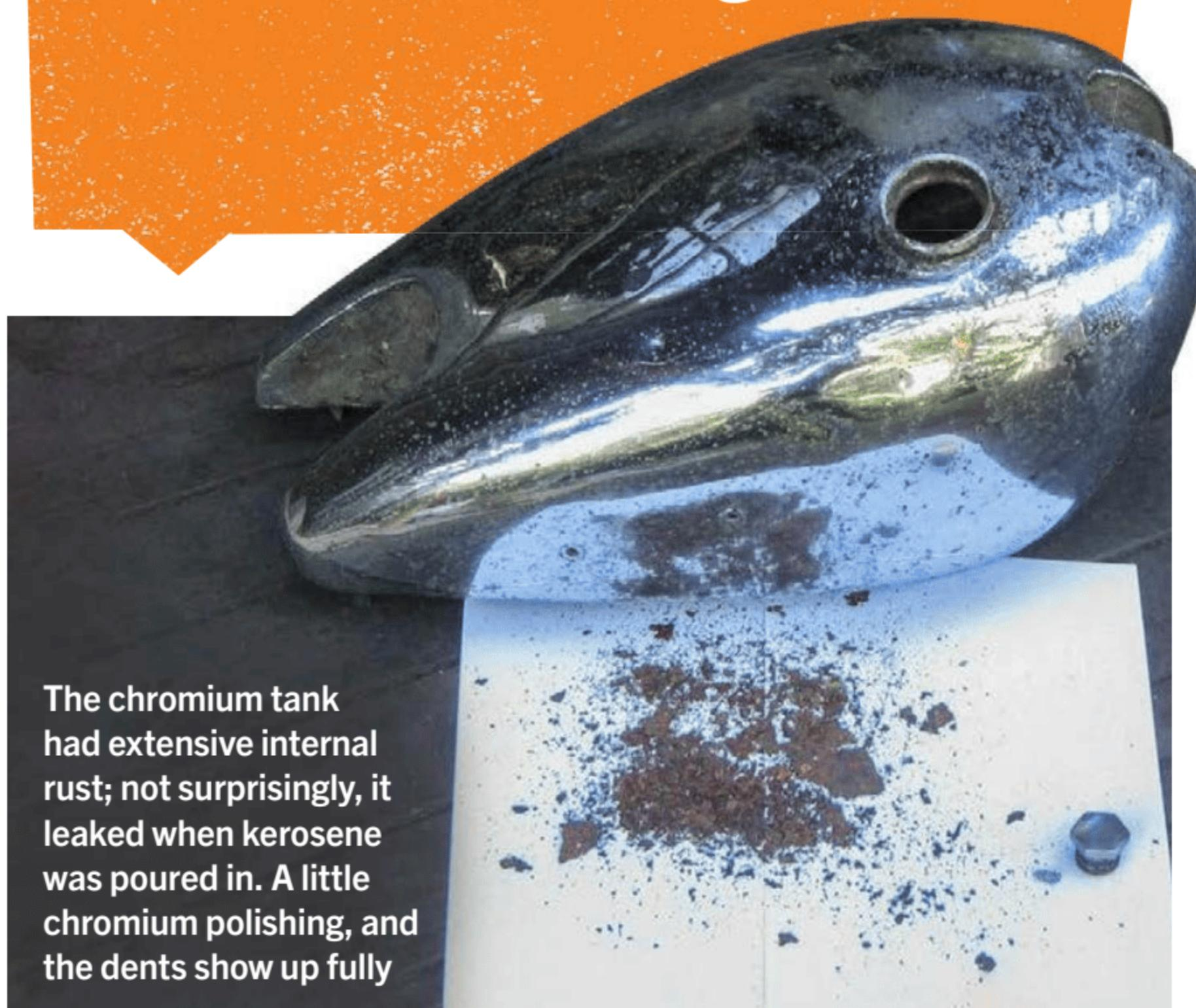
The chromium tank had extensive internal rust; not surprisingly, it leaked when kerosene was poured in. A little chromium polishing, and the dents show up fully
