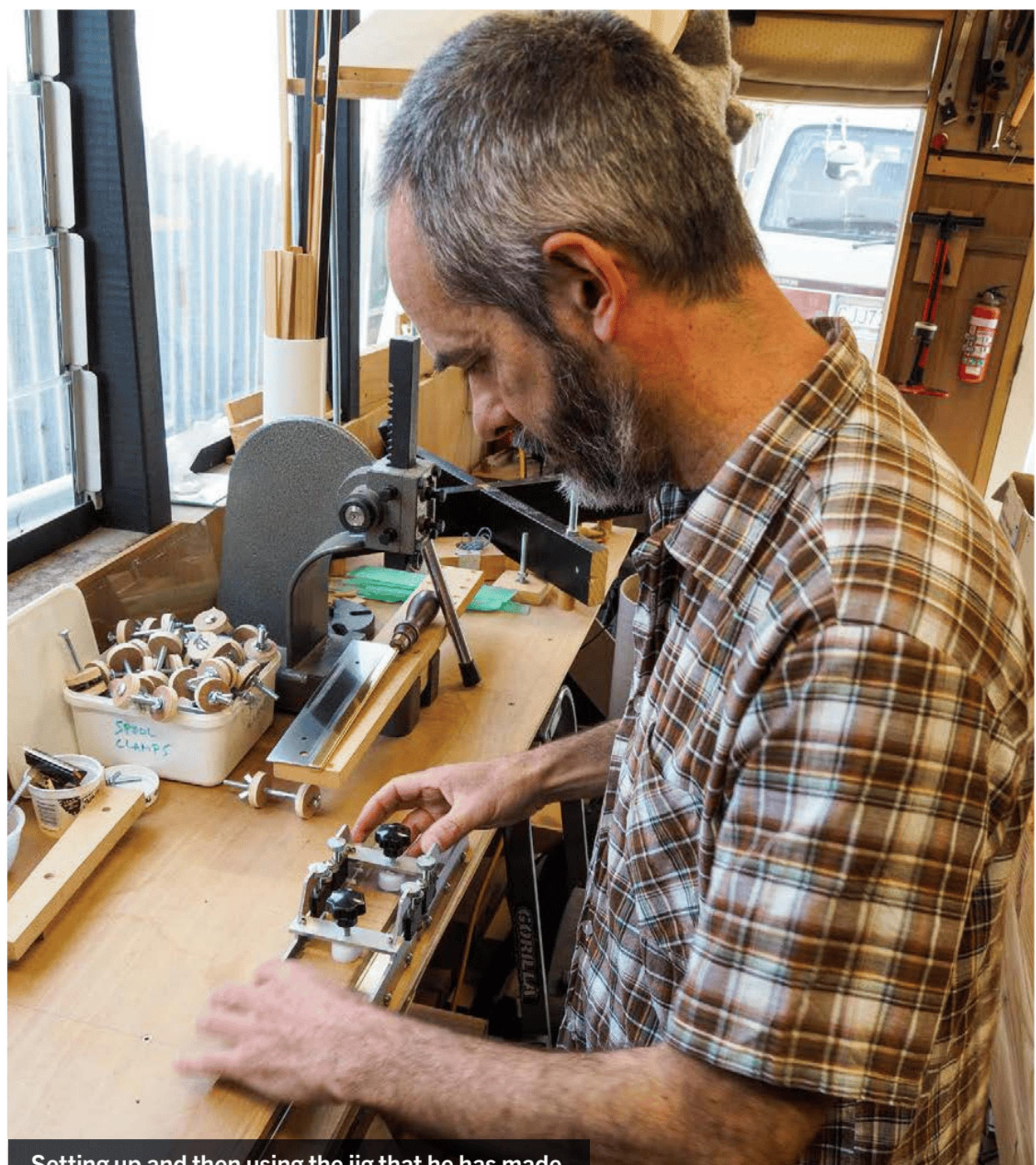
Setting up and then using the jig that he has made for cutting the slots for the nickel-plated-steel frets
