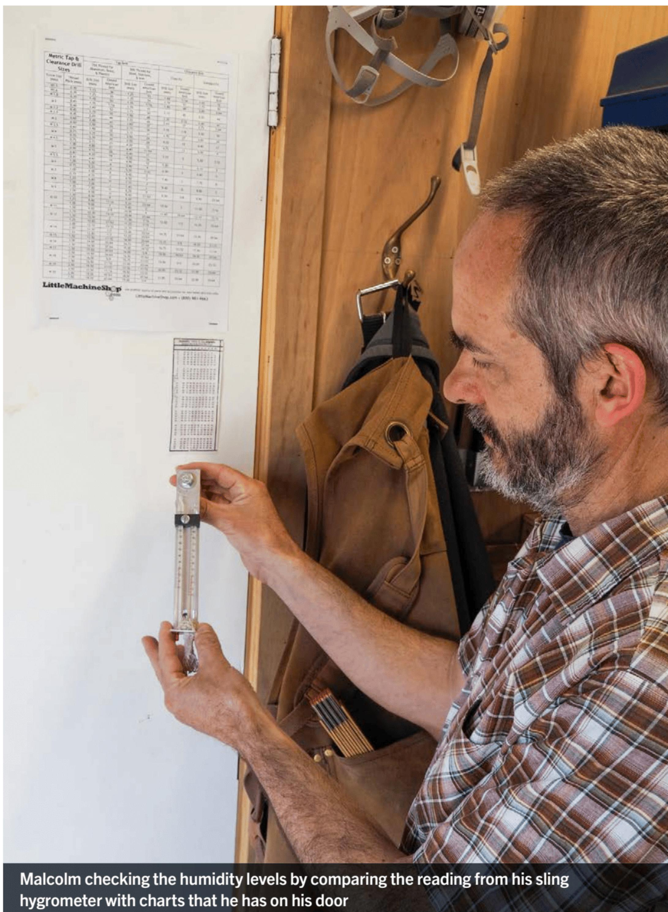
Malcolm checking the humidity levels by comparing the reading from his sling hygrometer with charts that he has on his door
