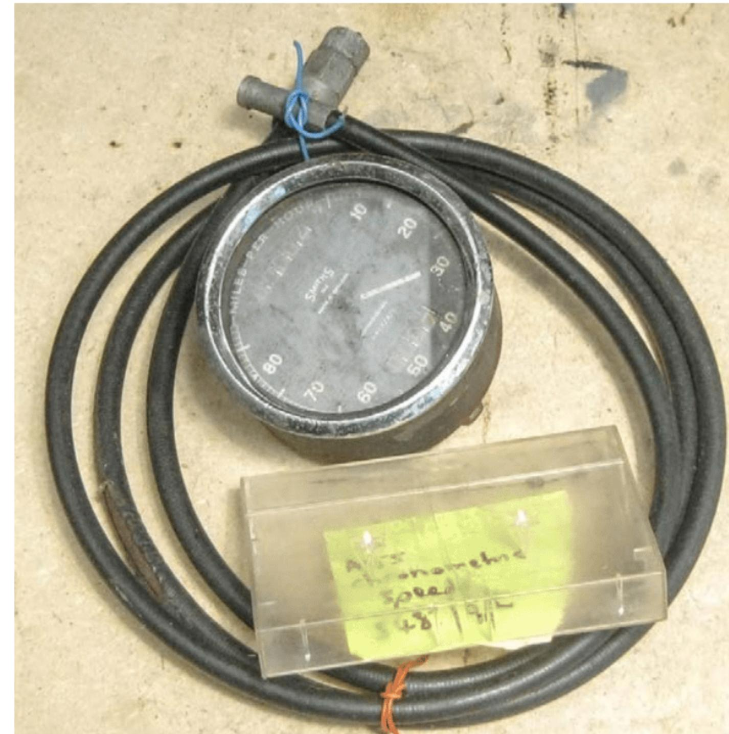
The chosen speedometer with its drive cable
