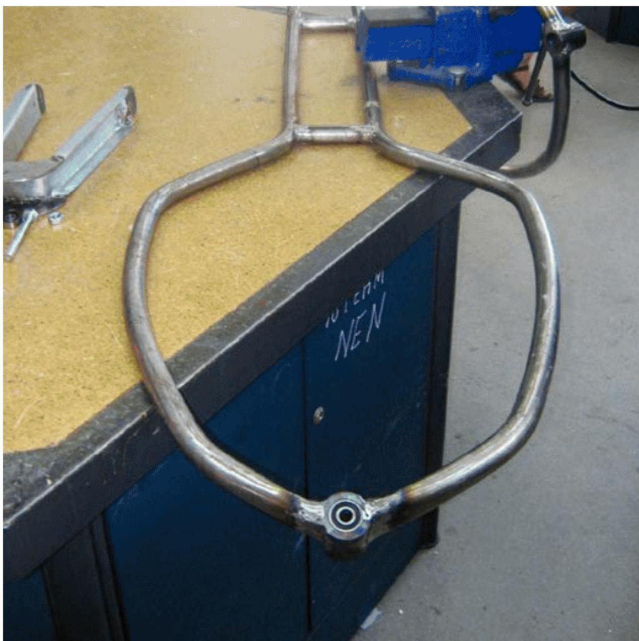
Bearing set-up welded
