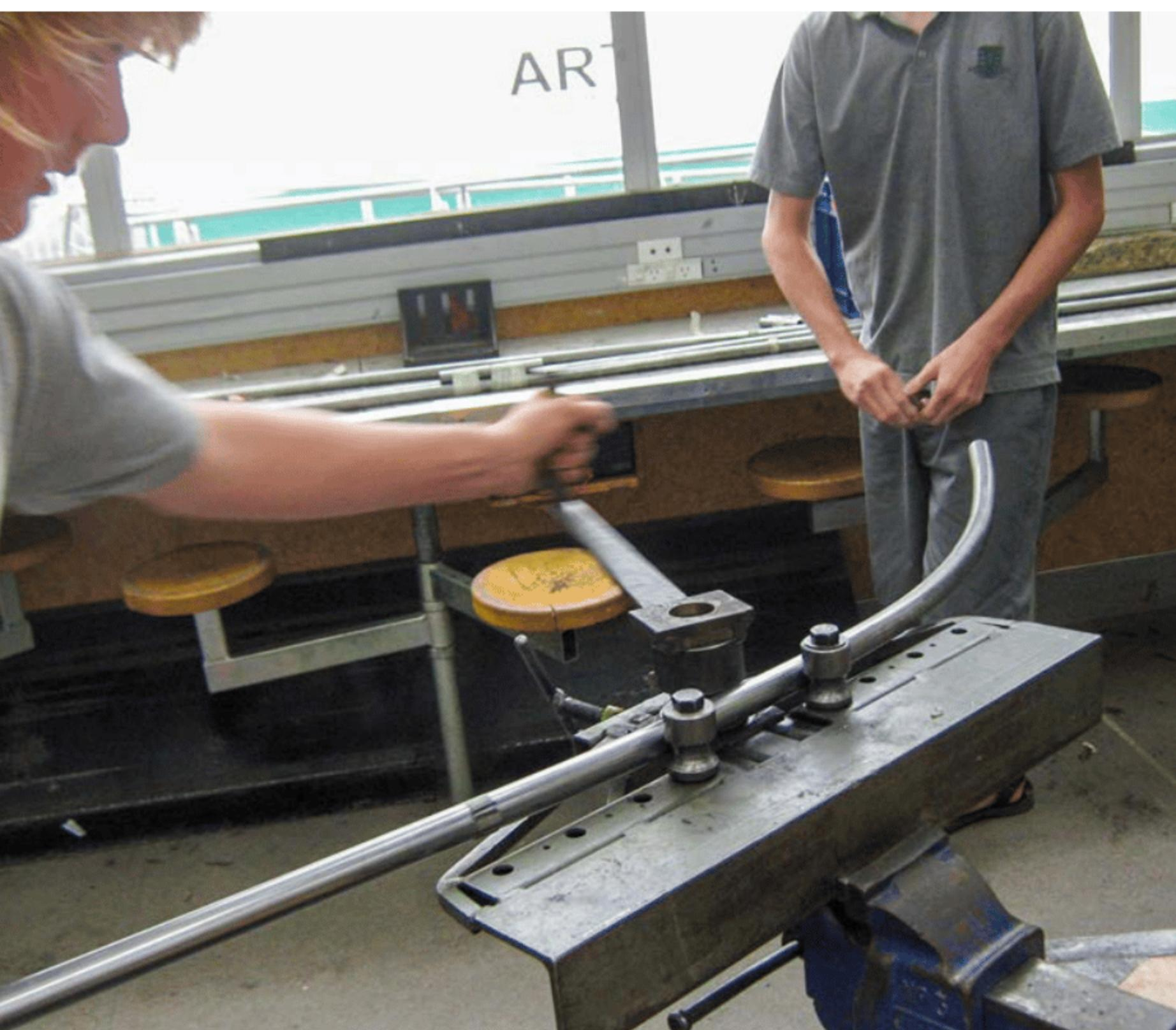
Bending the steel tube
