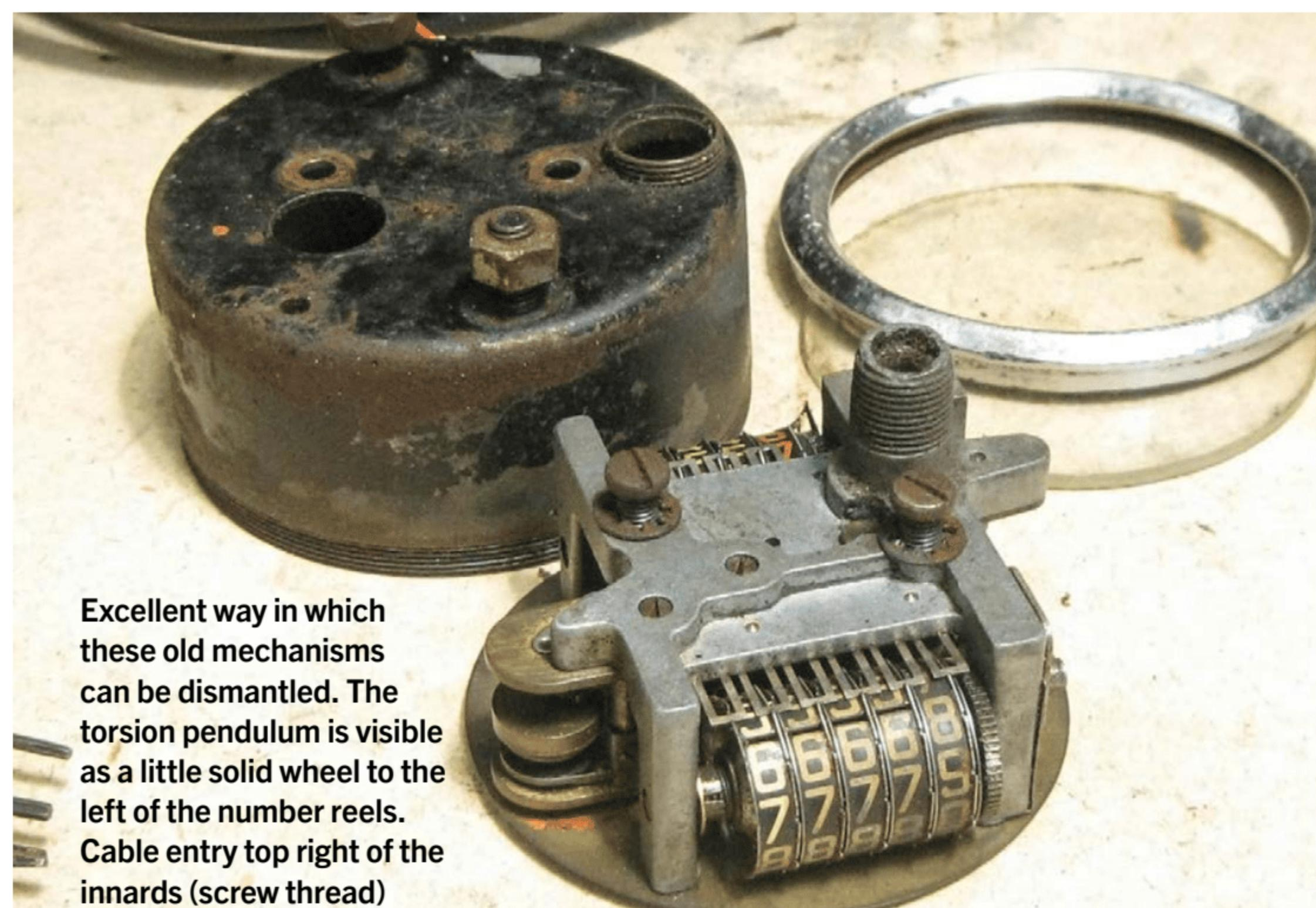
Excellent way in which these old mechanisms can be dismantled. The torsion pendulum is visible as a little solid wheel to the left of the number reels. Cable entry top right of the innards (screw thread)
