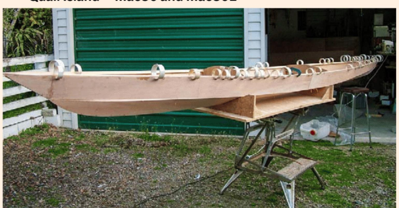
Sides not glued on. C-clamps on the upper interior wood strip
