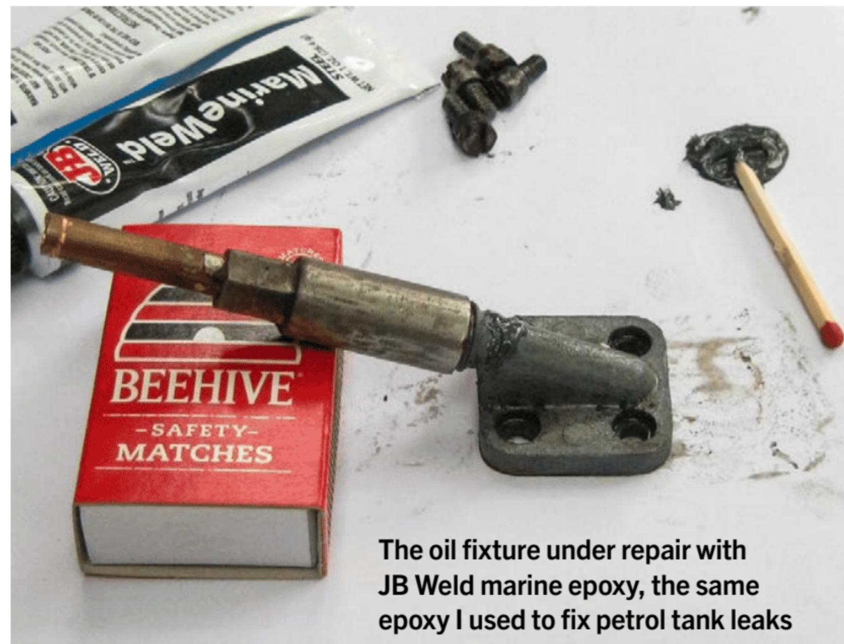
The oil fixture under repair with JB Weld marine epoxy, the same epoxy I used to fix petrol tank leaks
