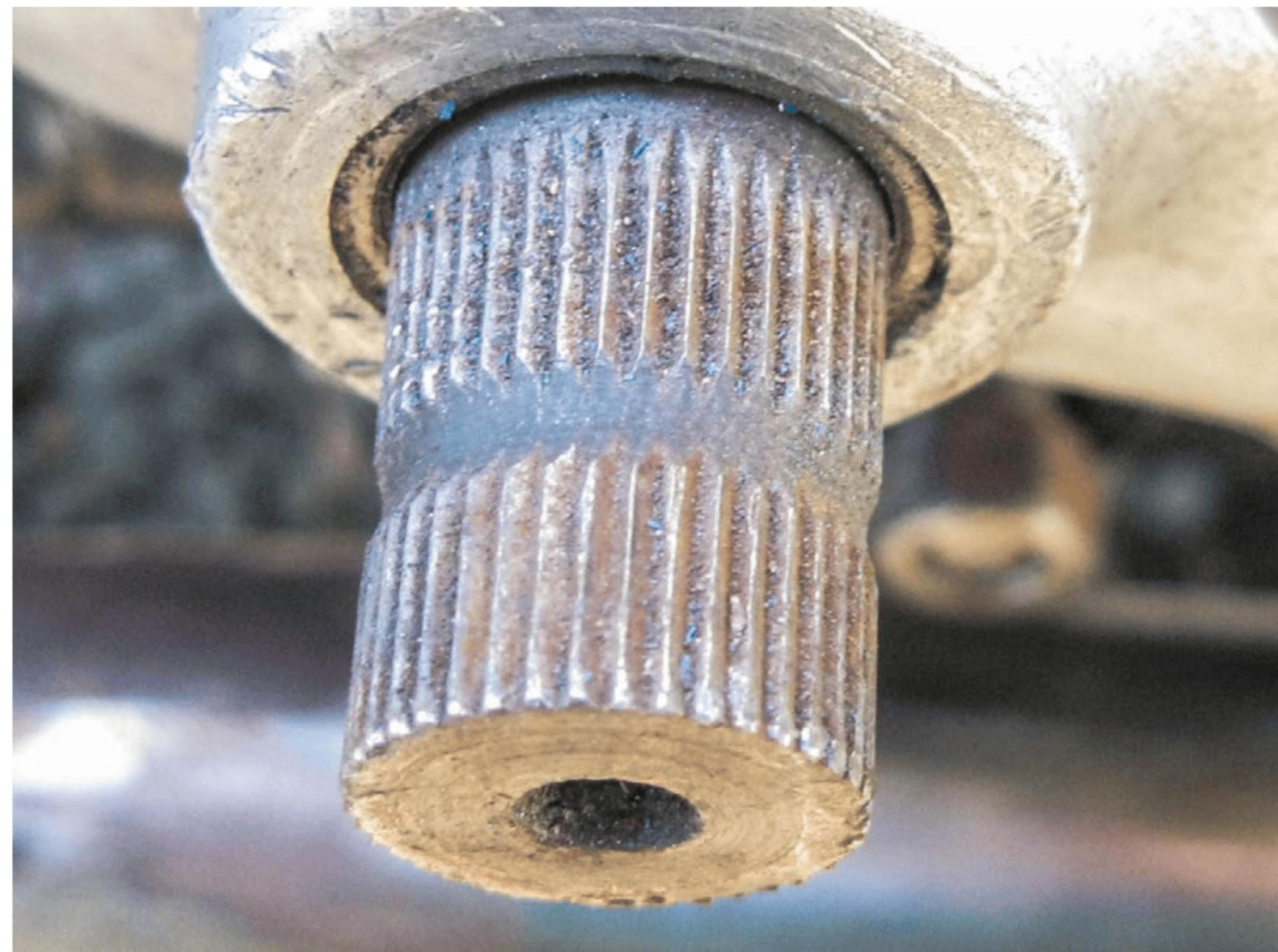
The splines let me down. Actually, these two views of the starter shaft show that the splines here are OK; the problem is in the matching machining in the start pedal. I have strategies for next time
