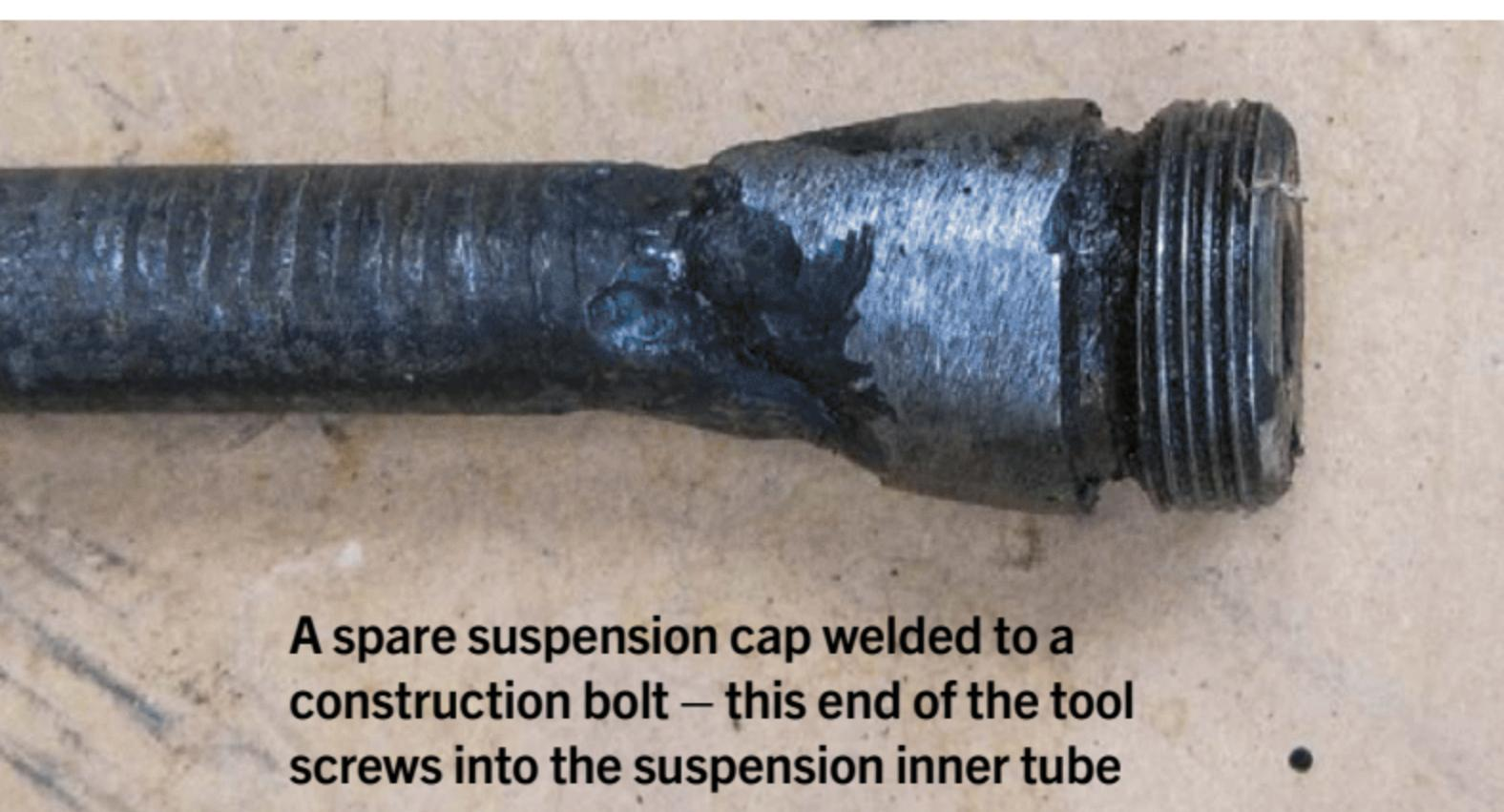
A spare suspension cap welded to a construction bolt – this end of the tool screws into the suspension inner tube
