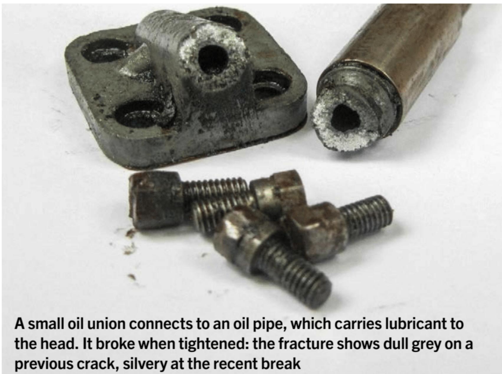
A small oil union connects to an oil pipe, which carries lubricant to the head. It broke when tightened: the fracture shows dull grey on a previous crack, silvery at the recent break
