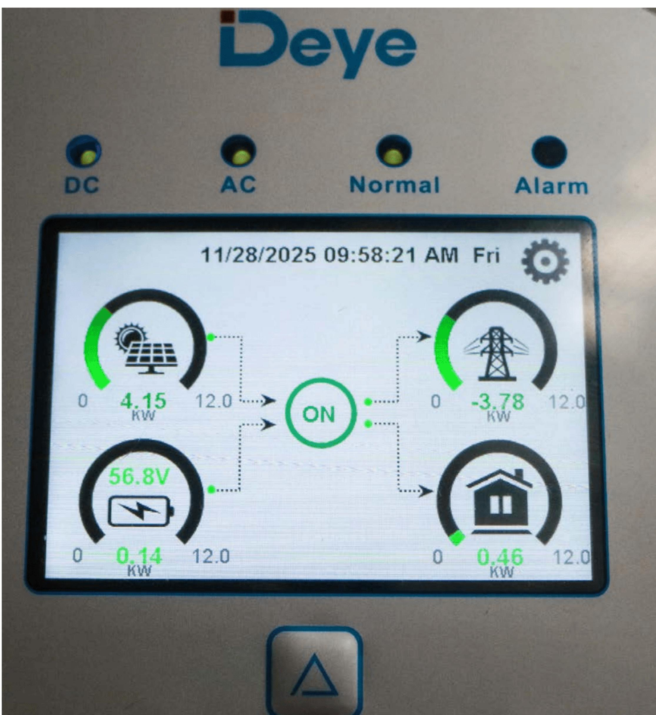
The inverter's control display. You can usually only make changes on the inverter, but you monitor performance on a mobile phone app
