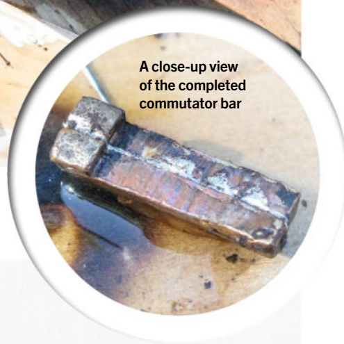
A bit of heating and pressing, and success. The margarine container had cooling water, the butane burner blue bottle base just visible
