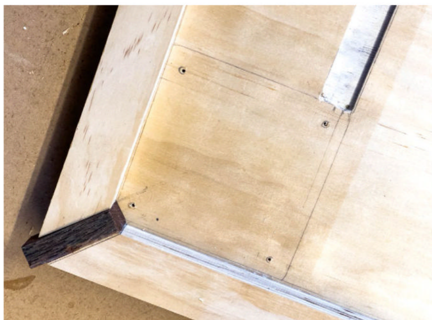
The corner highlight glued in place, all set to be trimmed
