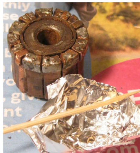
Toothpick and kitchen foil ready for mixing and placing plenty of epoxy
