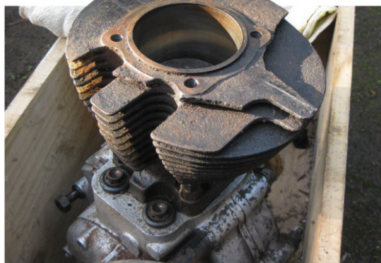
The damaged motor comes out of storage. The broken cooling fin is fixed up as described in part one
