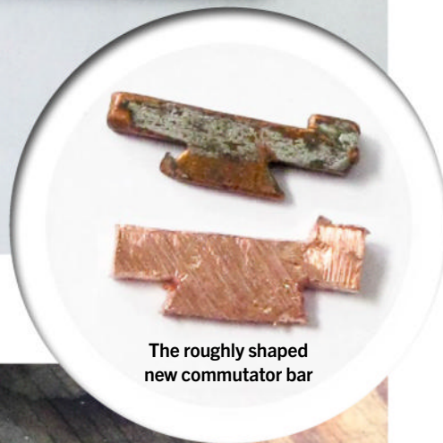
The copper was ground to a wedge shape (discolouration on the strip from grinding heat), and then the blank was cut out
