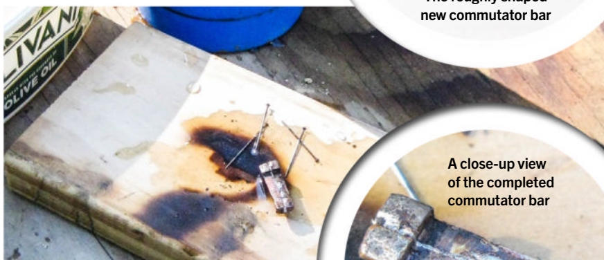
A bit of heating and pressing, and success. The margarine container had cooling water, the butane burner blue bottle base just visible
