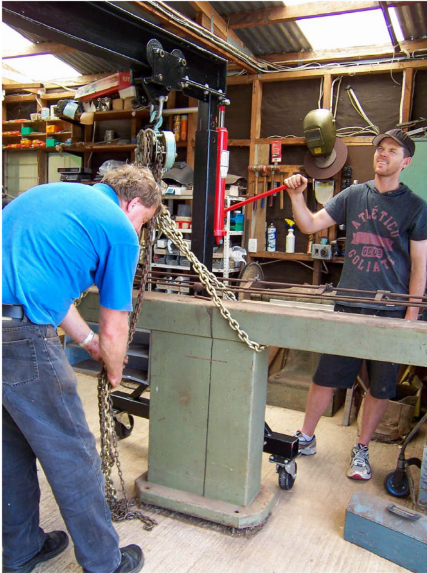
Preparing to lift a 300kg Italian-made mandrel tube bender
