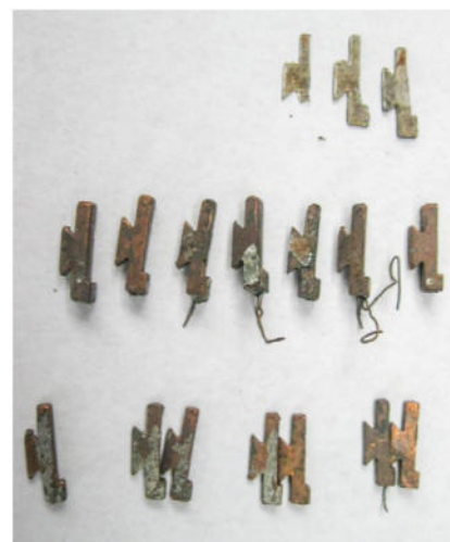
Commutator bars – some are in halves. Also, some bits of old mica. The half-bar at the bottom left has to be mated up with a piece I am yet to make
