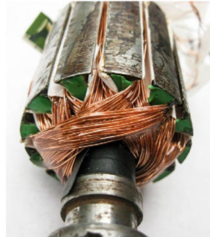
I've rewound the armature. The far end is where the commutator is fitted. Sellotape to help hold bits where necessary
