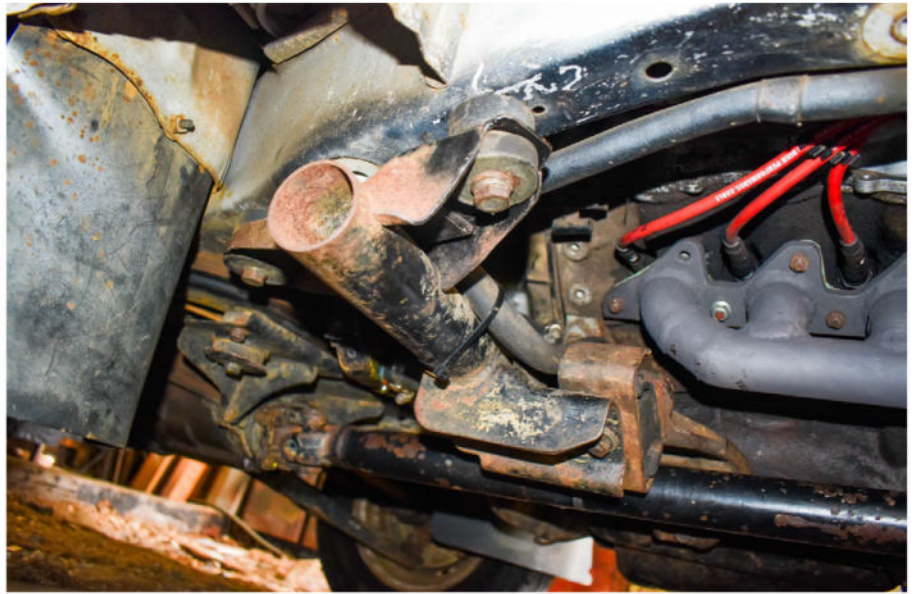
The relocated engine mounts and subframe to the chassis
