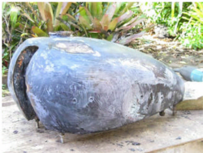
Rust neutraliser goes on
