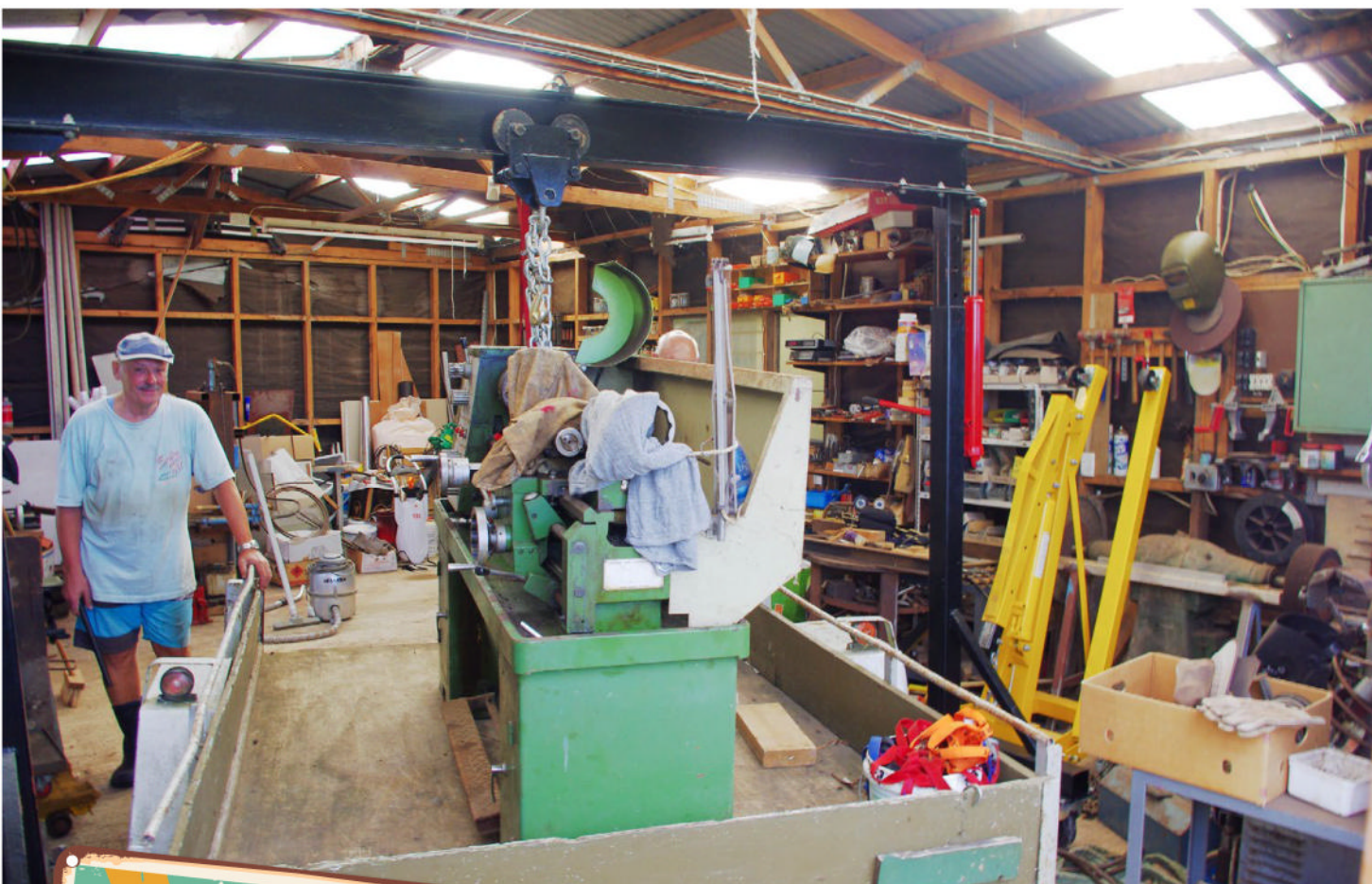
The 750kg lathe sits safely in the trailer, thanks to the homemade gantry crane
