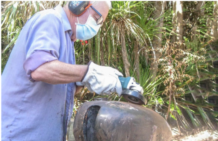
Flap disc cleaning the tank. Much bog will be needed here after rust treatment
