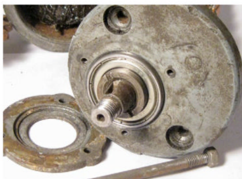
The drive end of the generator carries a chain sprocket in the primary chain case. The bearing went onto the shaft reasonably easily when it was warmed and the shaft had been in the freezer
