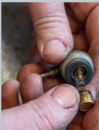
New seal on the non-return valve
