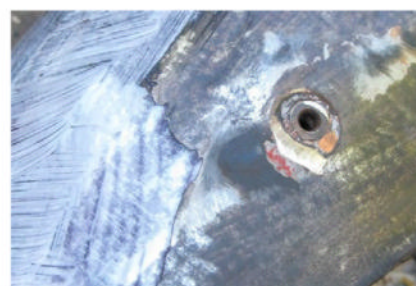
Rust neutraliser to the left. The small screw hole is for a plate which holds knee rubbers. There are further small holes forward (left, out of picture), which carry a small AJS badge
