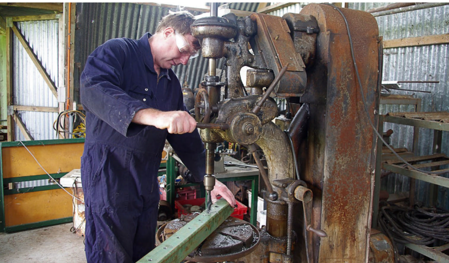
Drilling locking-pin holes at 100mm centres on sliding stanchion
