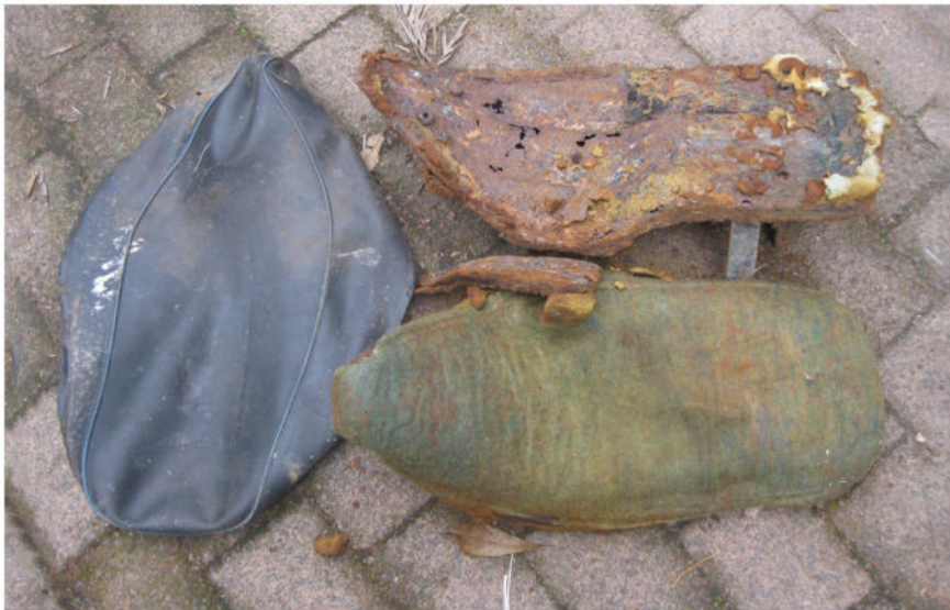
The seat comes out of storage. The vinyl cover is still OK. Luckily, I have a spare steel seat pan. The foam rubber has become brittle and hokey-pokey-like
