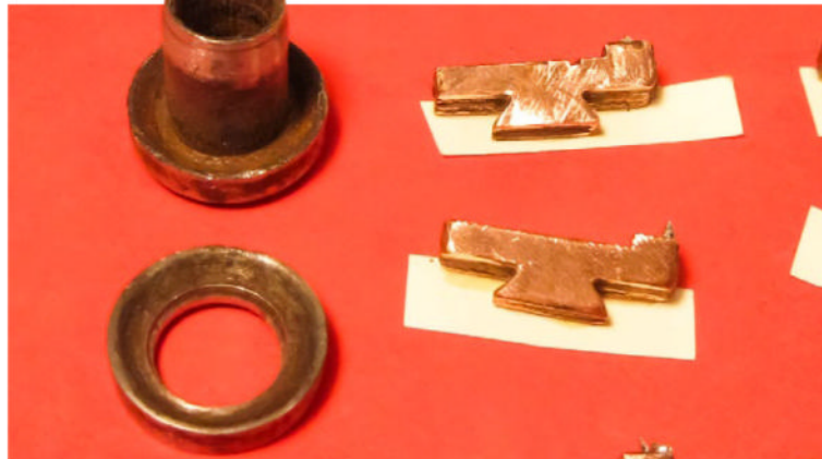
Second attempt. A short circuit somewhere. The old insulation was thrown out, and a total rebuild was done
