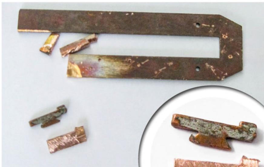
The copper was ground to a wedge shape (discolouration on the strip from grinding heat), and then the blank was cut out
