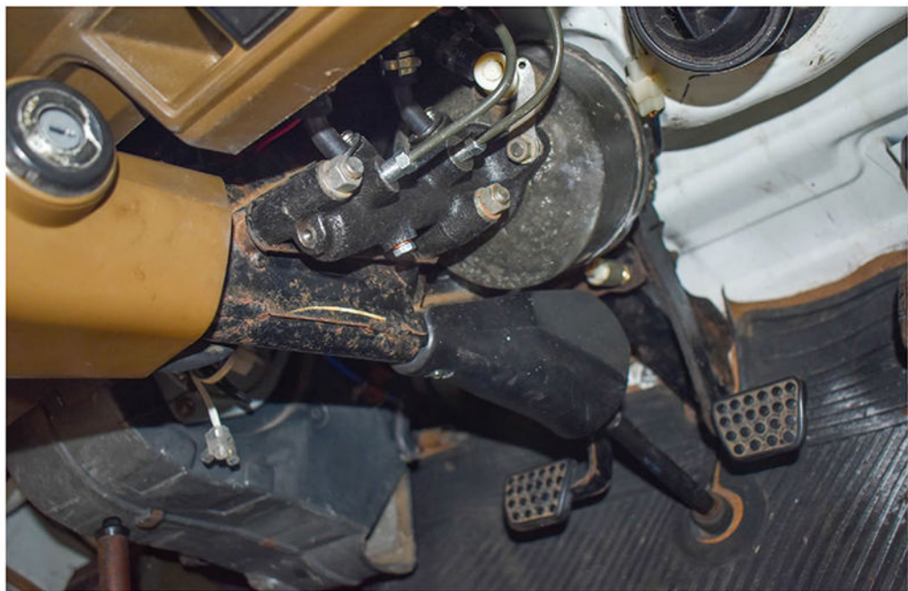
New brake master cylinder and booster installed
