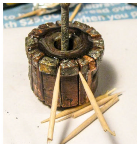
A bit of gap adjustment with toothpicks as wedges
