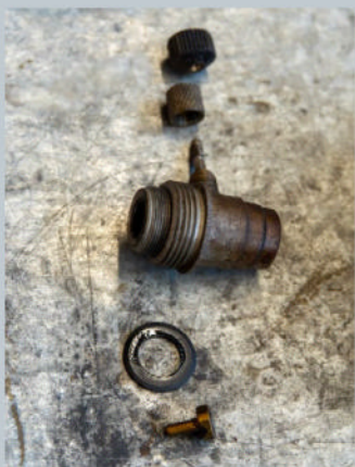
Clean, service, and reassemble the control cock
