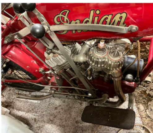
Thin spring steel wound around the pins at the base of the pistons kept the bike going – until it didn't
