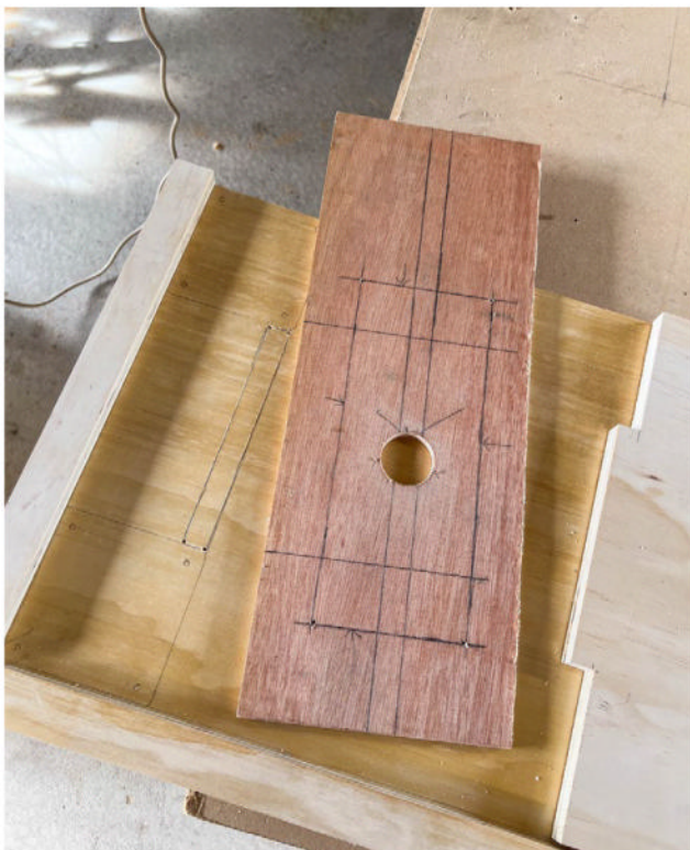
The hole I drilled in the middle so that I could mount it on my scroll saw
