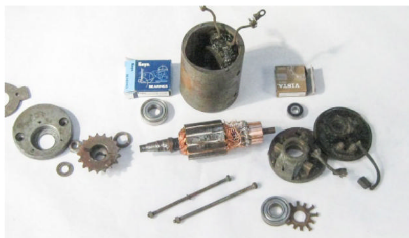
All the components of the generator. New bearings have been fitted, the armature has been rewound, and the commutator rebuilt and lathe-turned. The cardboard 'spider' protects the end of the armature
