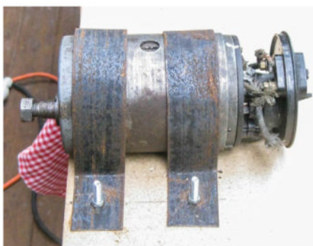
I strapped down the generator onto a breadboard. A cover band over the brushes and the commutator left off for further tinkering if needed
