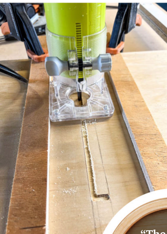
Using my router to cut out the recesses
