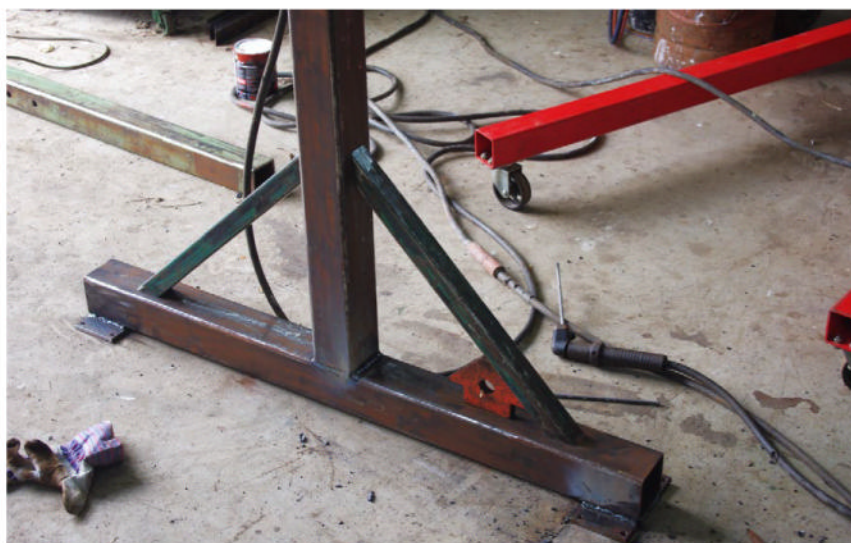
Pre-drilled mounting plates for castors sit the assembly flat on the floor
