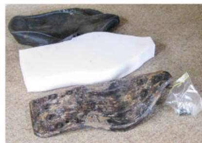
Vinyl seat cover is in OK condition, a spare steel seat pan (rust treated), and a foam block cut to shape at Para Rubber all ready to be wrestled together
