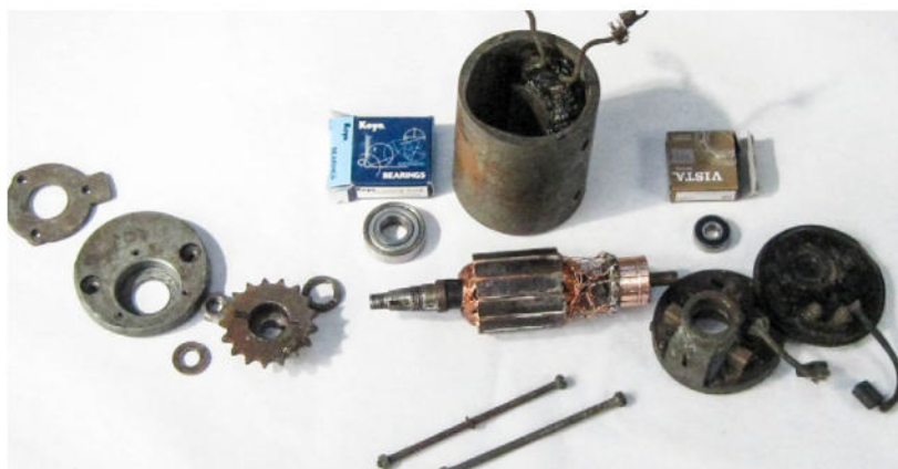
The bits are ready for reassembly. No problem getting new bearings
