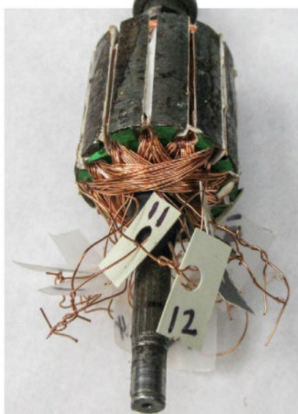
The commutator end of the shaft. No commutator yet. Each coil on the armature is tagged and numbered. You can see the green insulating 'spider' under the coils
