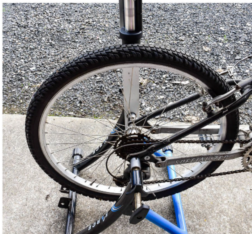
The roller is still there, now grub-screwed to the threaded rod and acting as a shaft locator
