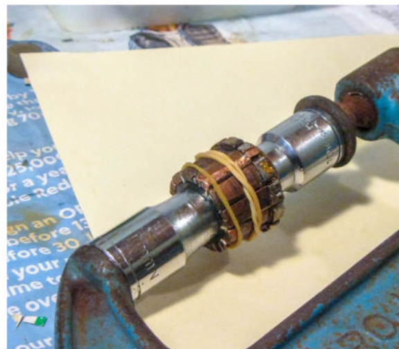
Pressing all into place using a G-clamp and a couple of appropriately sized sockets
