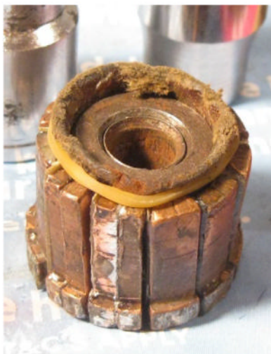
After pressing. The new piece left of centre
