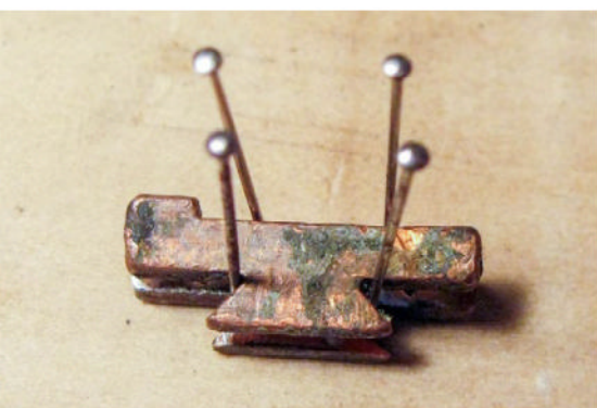
Two half-commutator bars have been tinned on their mating surfaces and positioned with pins ready for heat and pressing
