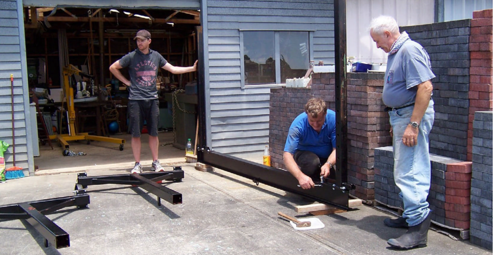
Geoff bolts beam and end-post (upside-down) together
