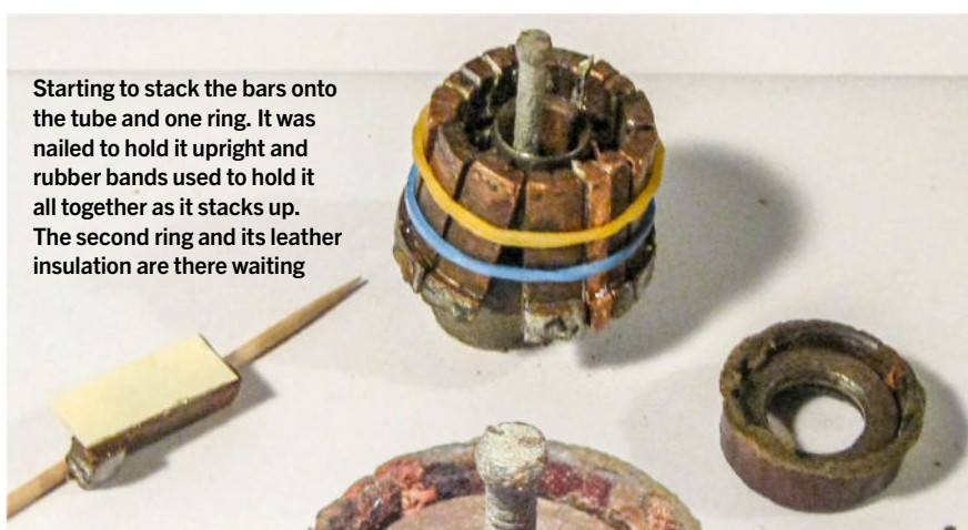
Gluing paper and epoxy onto the sides for insulation. Twelve bars for this commutator
