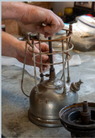
Unscrewing the vaporiser
