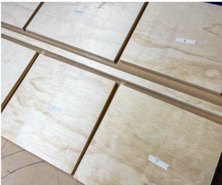
I've put a piece of masking tape on each piece to number them in accordance with my cutting schedule – it's intended to lessen any confusion ...
