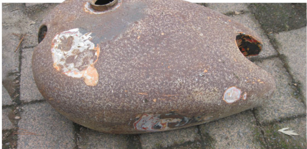
The tank comes out of 50 years' storage, dents visible
