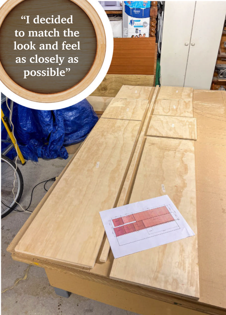
All the pieces I need for the cabinet, along with the cutting schedule I drew up in SketchUp.
