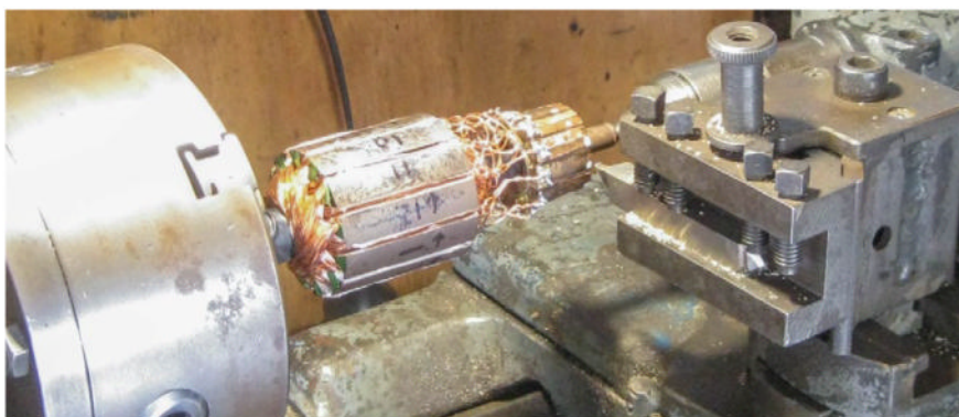
Turning the commutator on the lathe to get the bars at even height cleaned up
