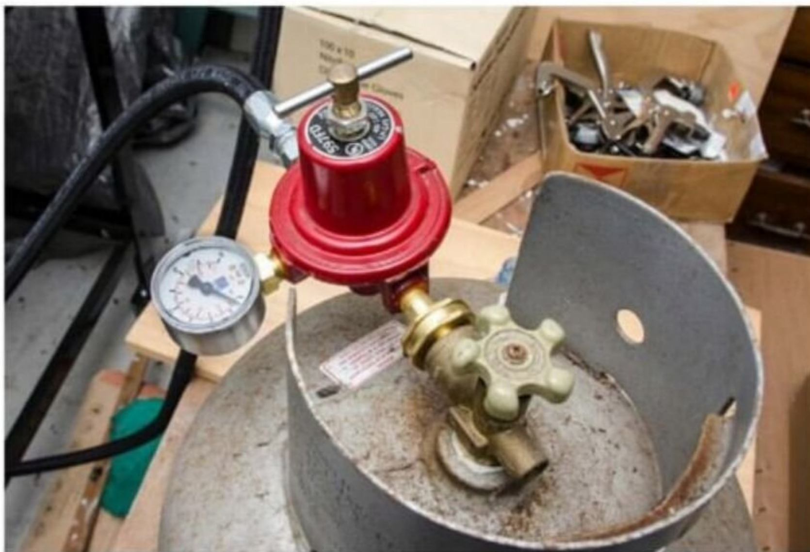
The pressure valve with gauge
