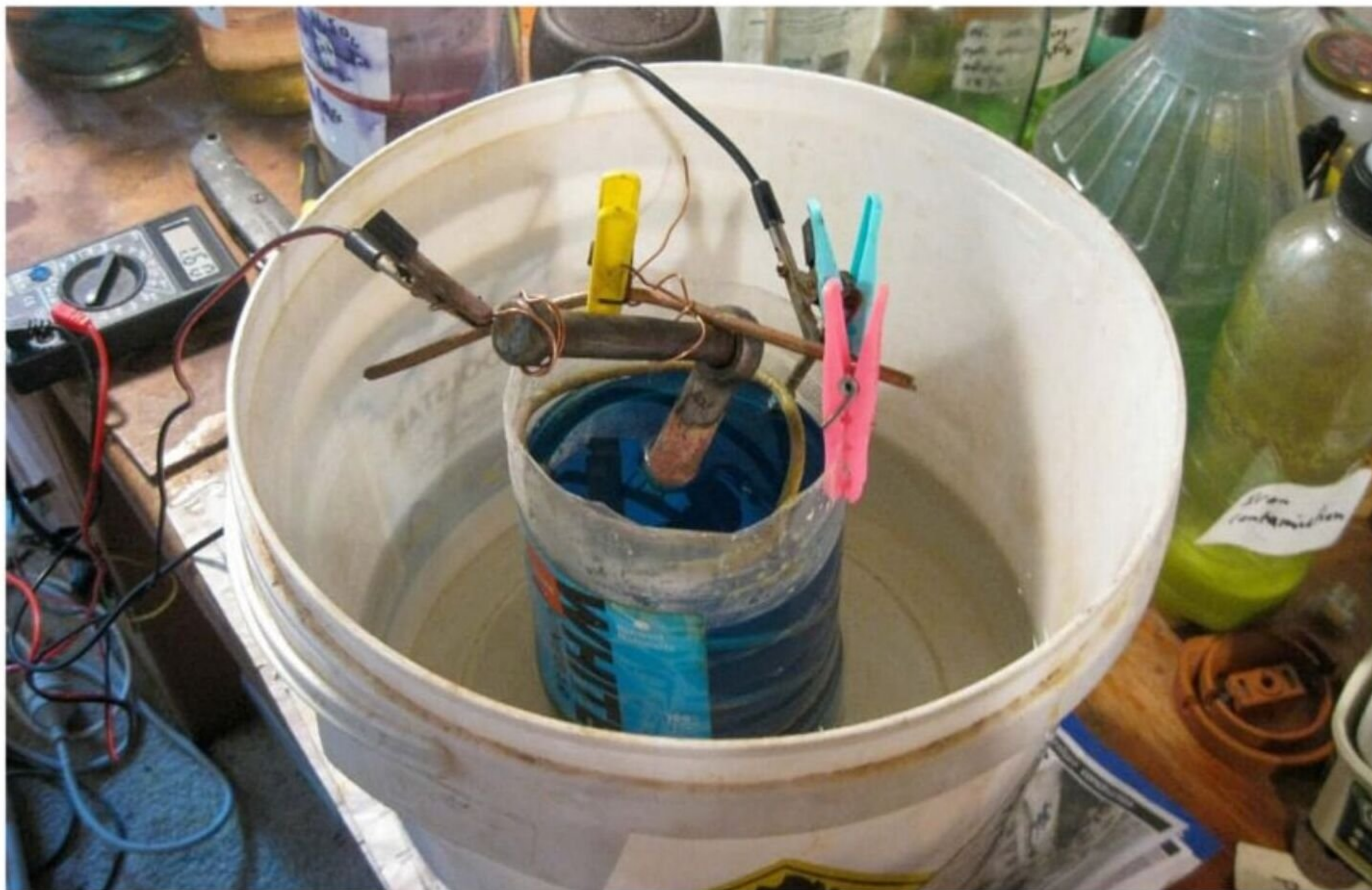
Copper plating in action: the bucket of hot water raises the temperature to about 35 degrees
