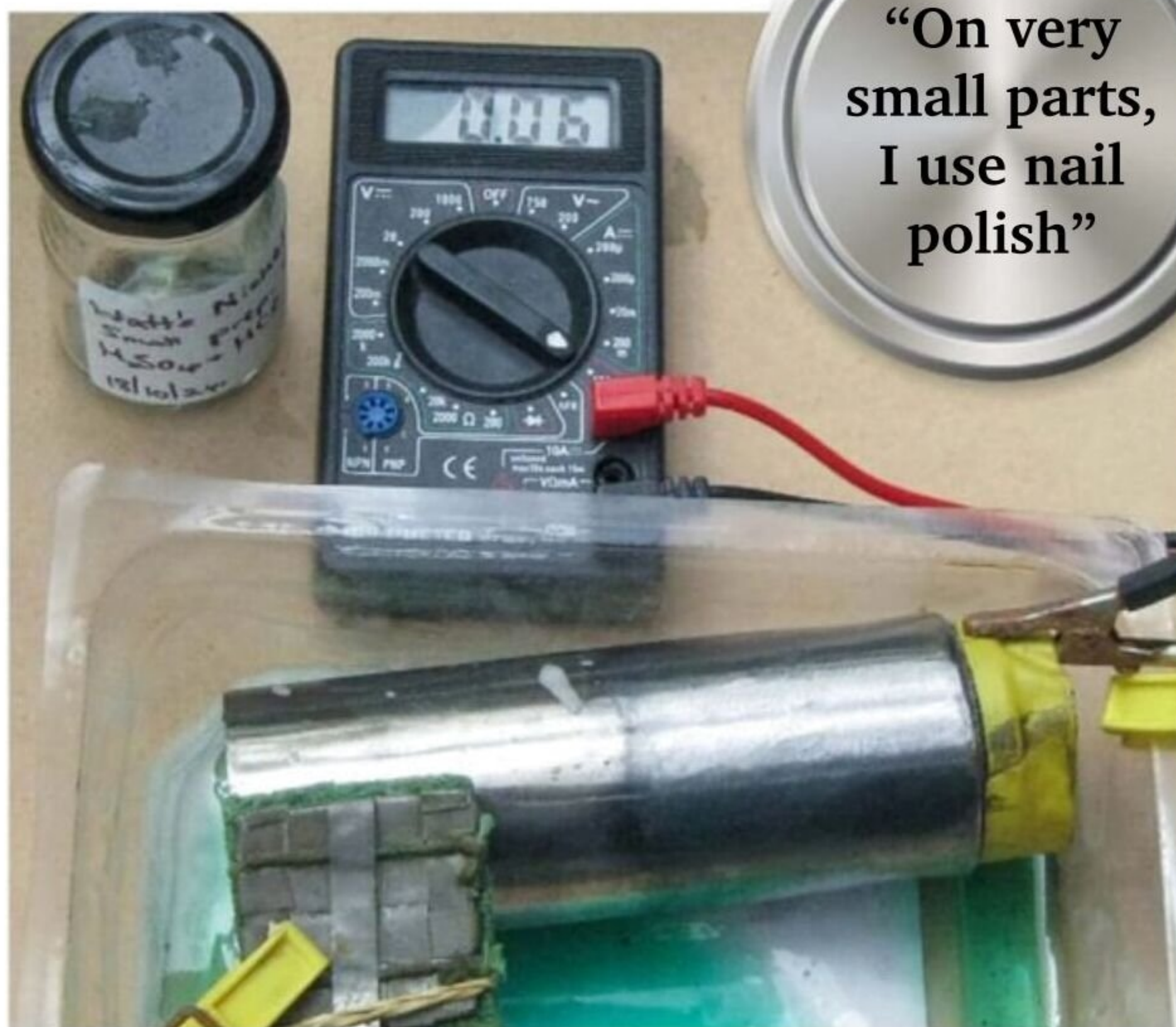
Still brush plating – the creamier-looking nickel plate is to the left of the piece; steel is to the right
