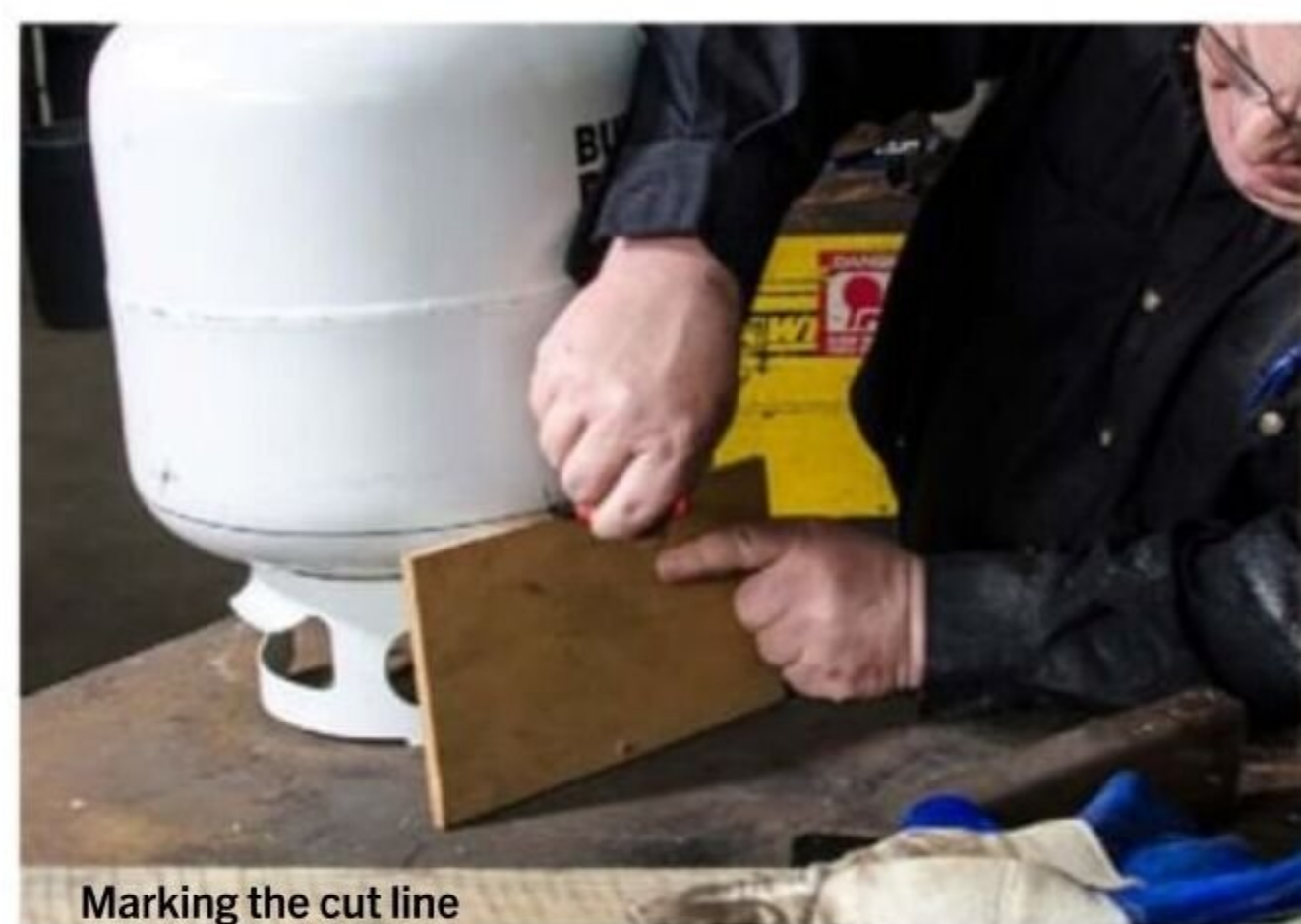
Making a registration mark prior to cutting the end off
