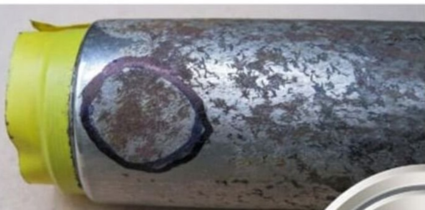
The front suspension tube extension: some rust pitting, a dent (circled), and the screw thread masked by insulation tape
