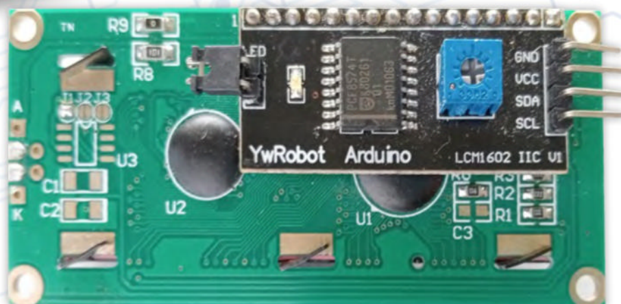
I2C connection for LCD
