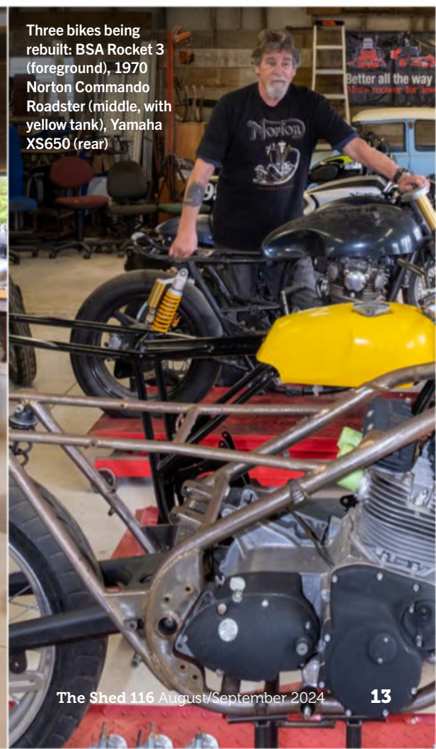
A modern version of the classic Triton taking shape, 2015 Thruxton engine in a custom copy of a Norton "Lowboy" Dommie racer frame
