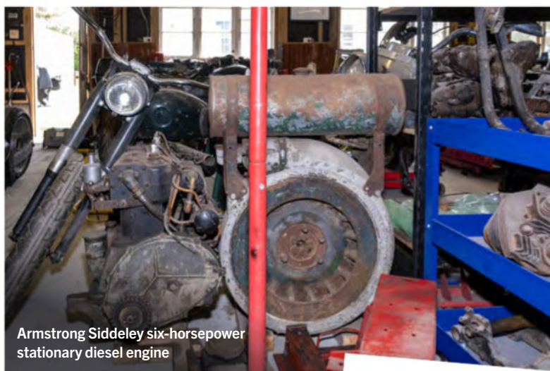
Detail of the Armstrong Siddeley diesel engine
